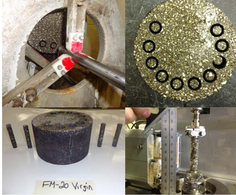
Figure 3.6 Specimen preparation process for FAM specimens including cutting, coring, and test setup.
