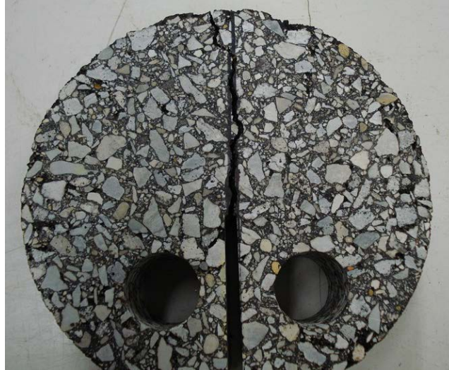
Figure 2.4 DCT specimen after the completion of a test.
