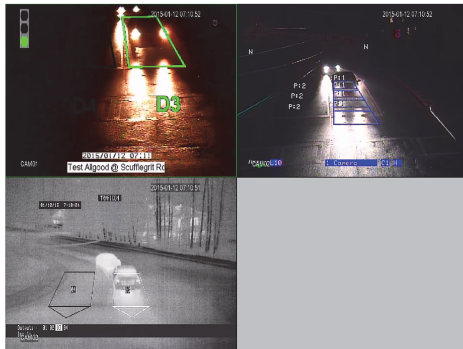
Figure 8.5 Normal conditions – nighttime (site 2; upper left: Autoscope AIS-IV; upper right: RZ4 Advanced WDR; lower left: FC-334T Thermal)
