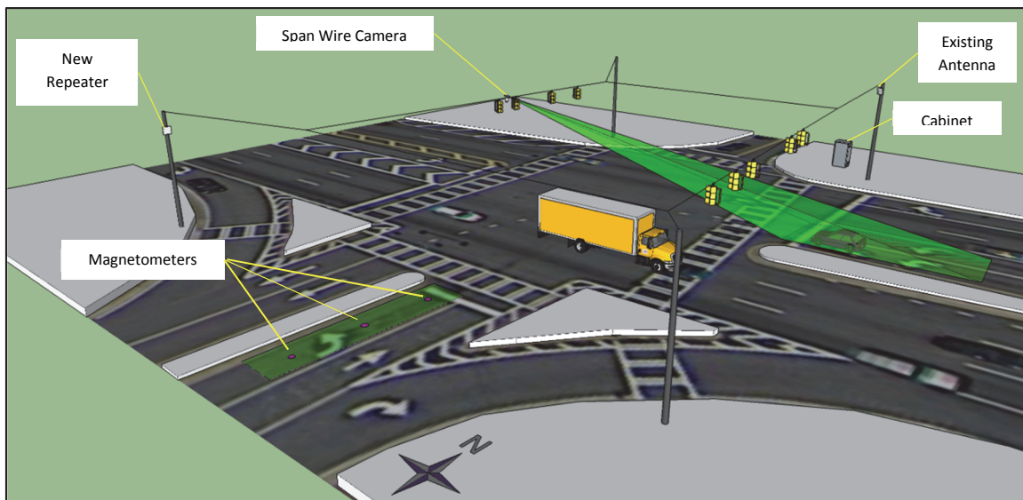
Figure 5.14 Three-dimension aerial view – field setup of wireless magnetometer and Vantage SmartSpan camera.
