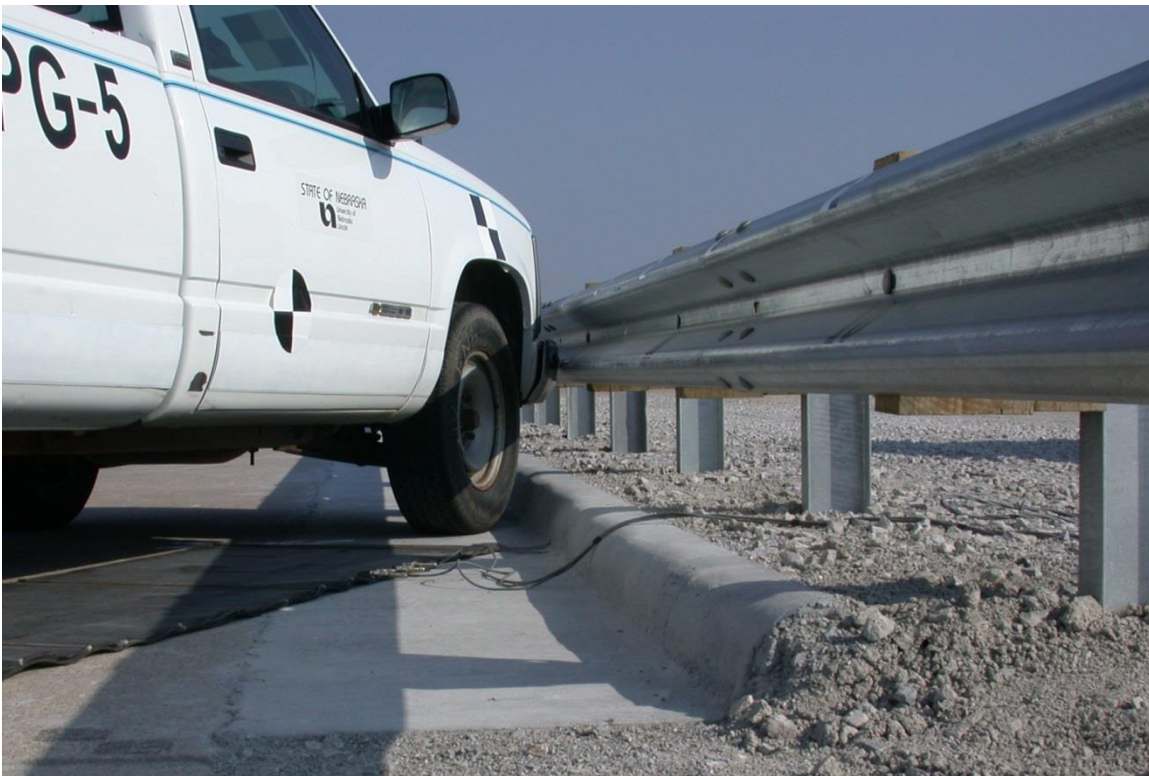
Figure 14. Impact Location and MGS Installed in Combination with Curb, Test No. NPG-5
