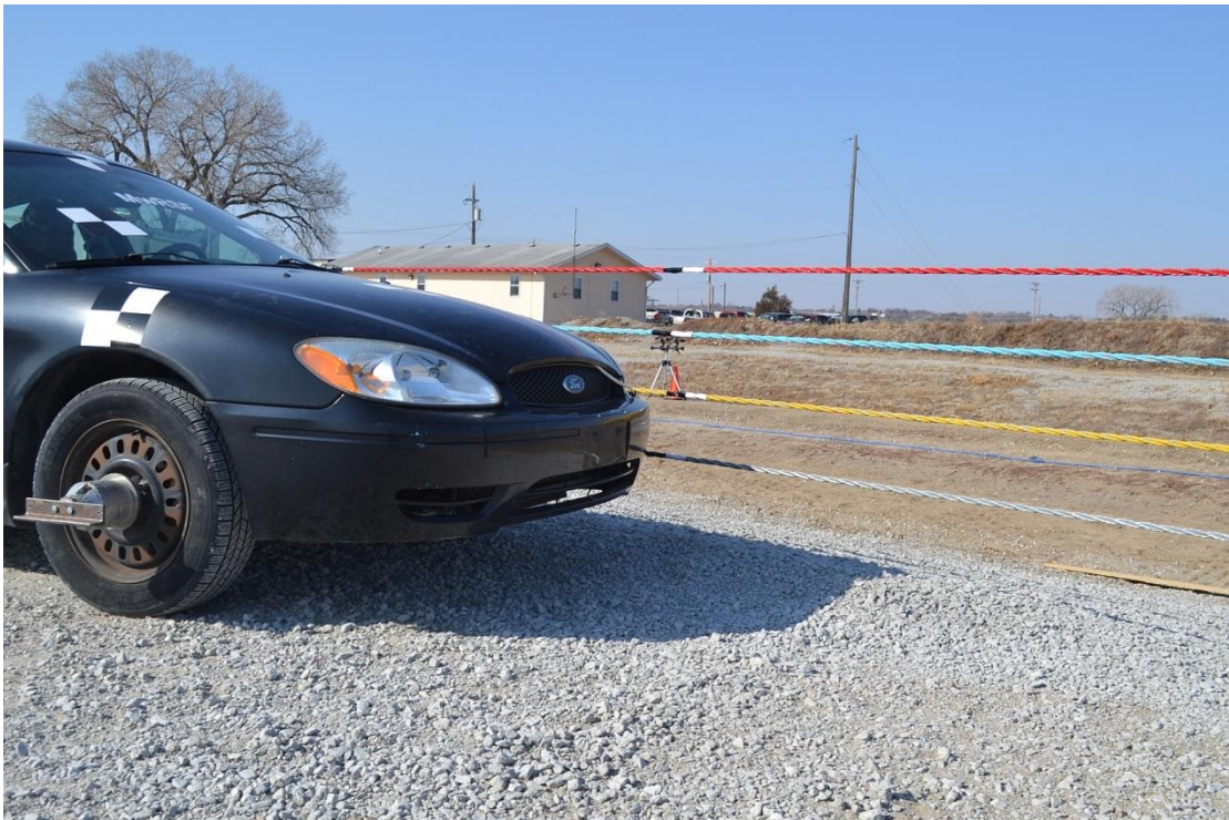
Figure 39. Cable Heights Relative to Test Vehicle, Test No. MWP-1
