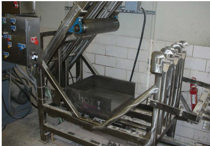
Figure 4.1 Linear kneading compactor for preparing asphalt slabs.
