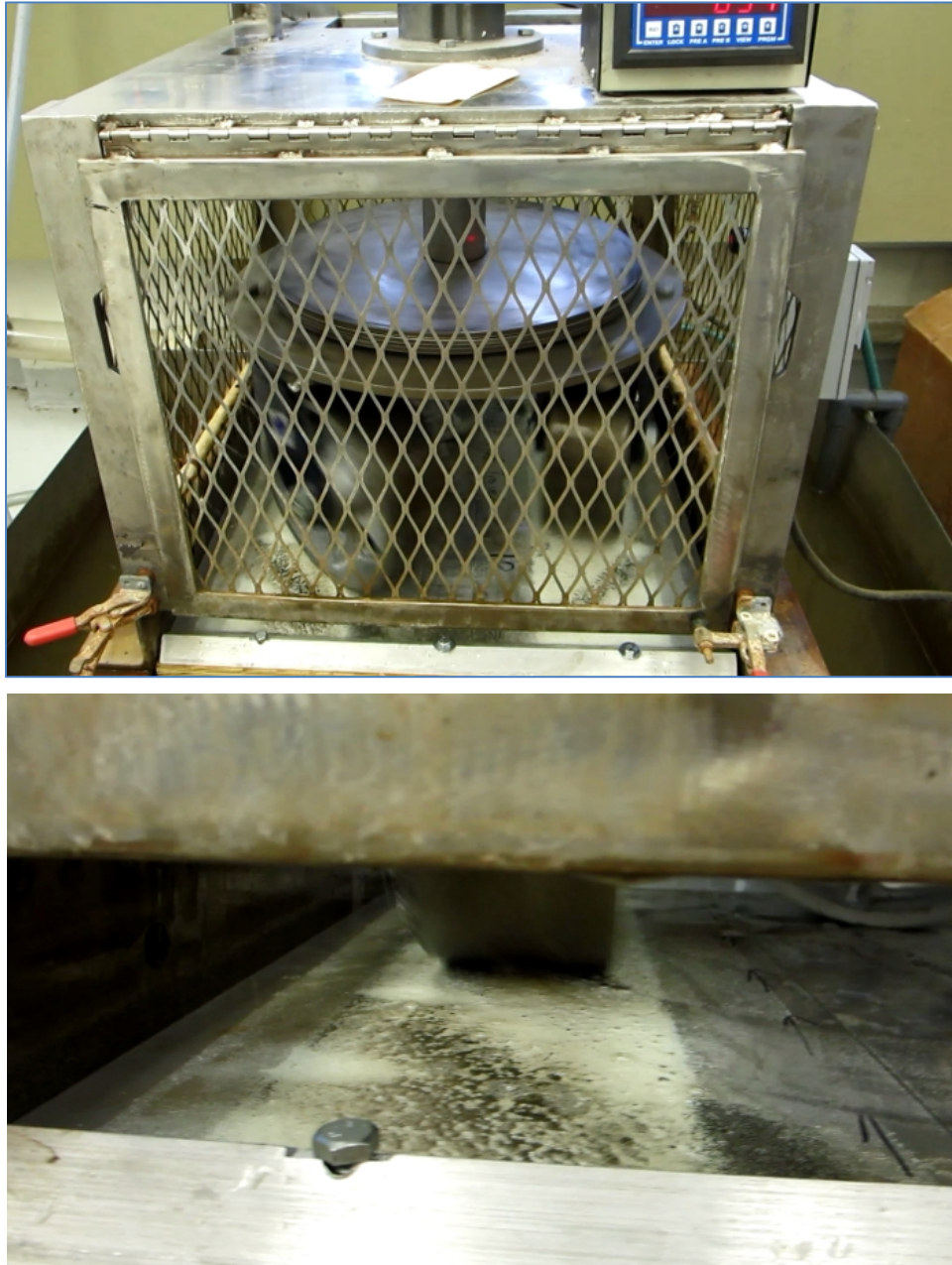
Figure 4.6 Accelerated wearing of samples from test deck.
