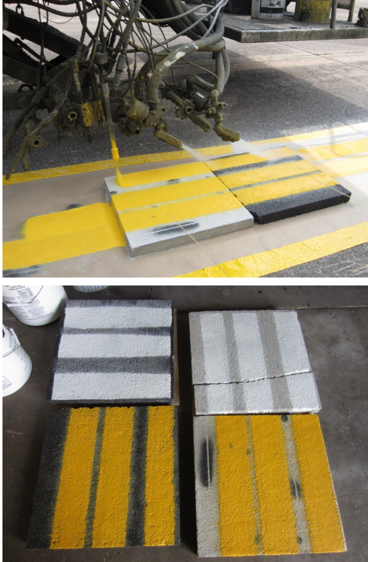
Figure 4.2 Pavement marking samples.
