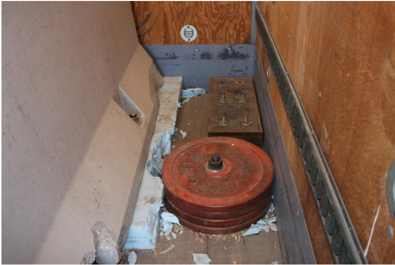
Figure 39. Ballast Installation, Test No. SFH-3
