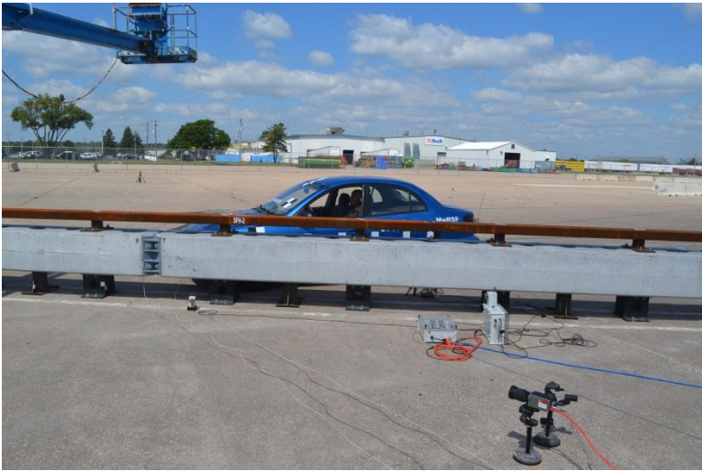
Figure 67. Impact Location, Test No. SFH-2
