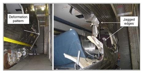
Figure 18. Outward Deformation of the Right Side of Car 7488, Tearing the Sheet Metal and Exposing Jagged Edges
