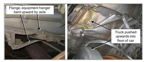
Figure 17. Impact of the Axle of the Front Truck of Car 7488 with the Floor of the Occupant Volume
