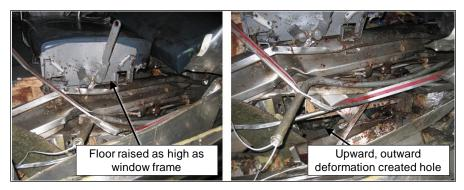
Figure 19. Upward Deformation of the Interior Floor, Resulting in a Breach of the Occupant Volume
