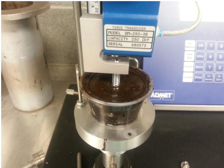
Figure 7: Cone Penetration Test Equipment
