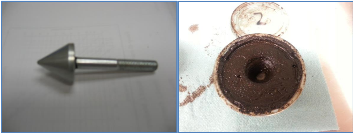
Figure 6: Cone Apparatus and Sample of RAP mortar.
