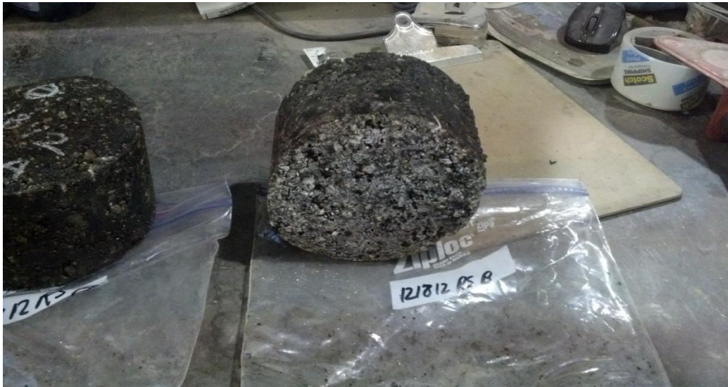
Figure 10: Reflex puck after stability test at 120 degrees
