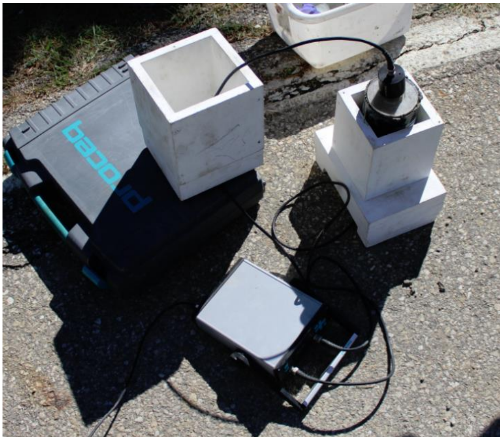
Figure 3. Test setup with sample and transducers in a wooden frame for stability
