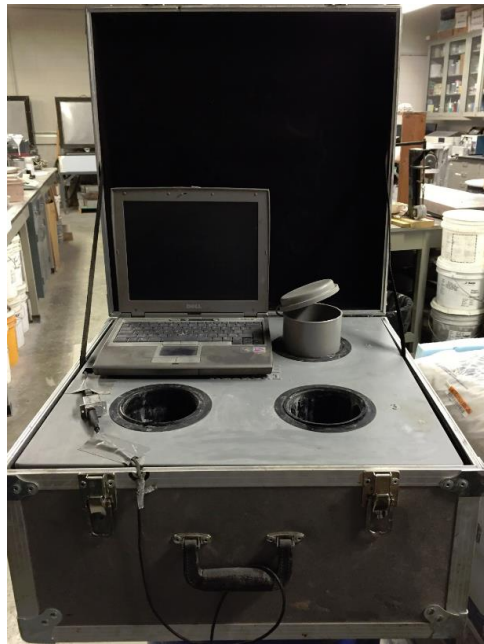
Figure 4. Calorimetry test device for measuring the heat of hydration of concrete
