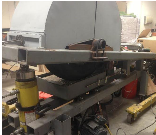
Figure 26: Traction and wear test equipment.
