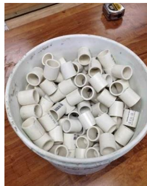
Figure 32: De-burred PVC pipe
