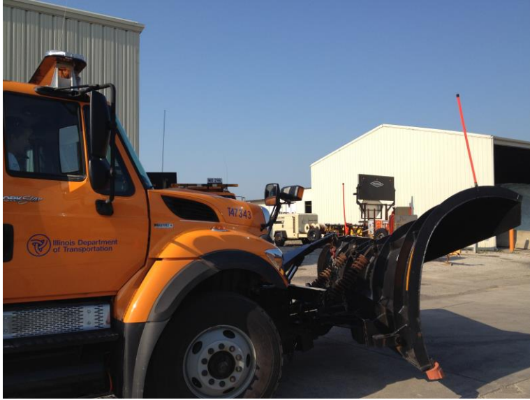
Figure 8. Carrier structure of front-mounted Alaskan plow.
