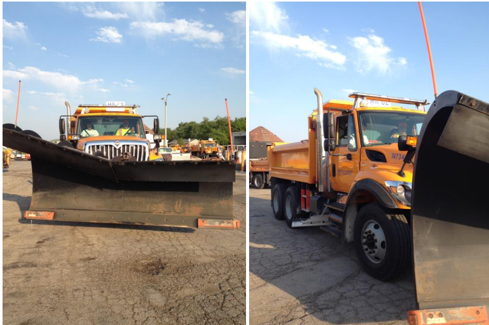
Figure 7. Front-mounted Alaskan plow on tandem dump truck.
