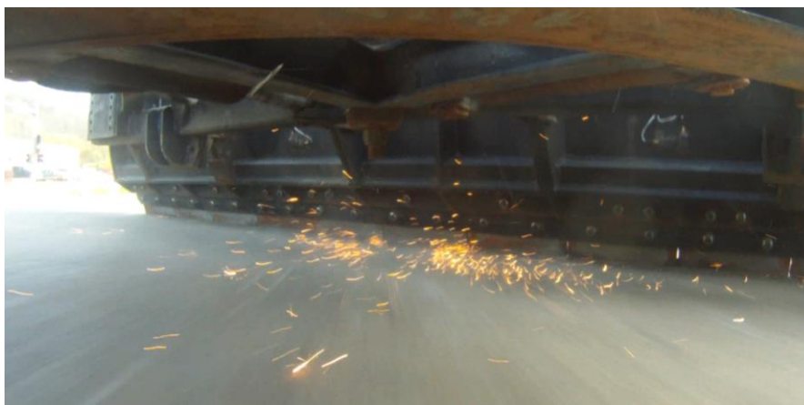
Figure 35. PolarFlex blade on concrete pavement.
