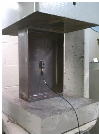
Figure 16. Steel section assembly used for attempted calibration.
