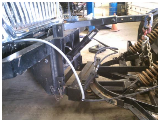
Figure 20. Conduit fed into truck engine bay.
