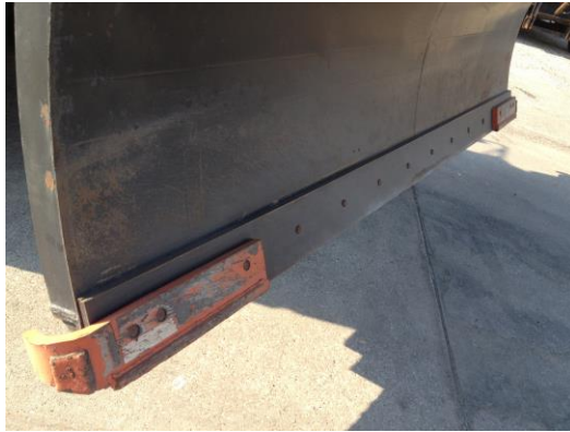
Figure 9. Steel blade with carbide insert and curb guard.
