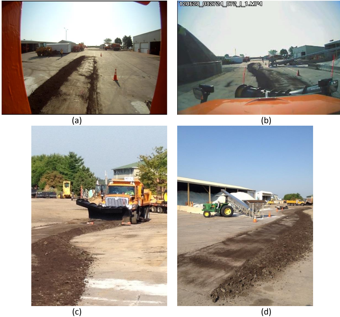
Figure 28. Dry-soil runs: (a) rear GoPro camera view of concrete, (b) front camera view—soil run on concrete pavement, (c) plowing with the Alaskan plow during soil run, (d) complete layout of soil run.
