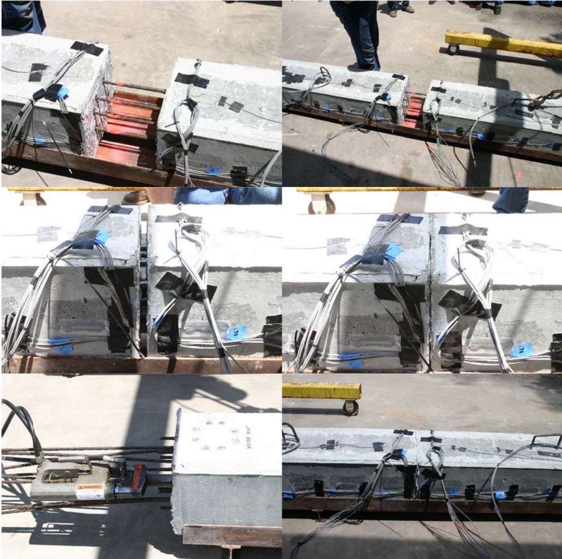
Figure 4.103. Final joining and stressing the splice connection.
