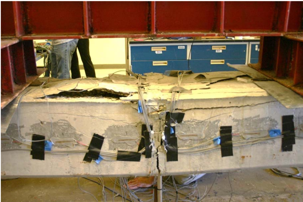
Figure 4.117. Splice Pile 2 before and after testing. Again compression block only in cover. Failure 36kips.
