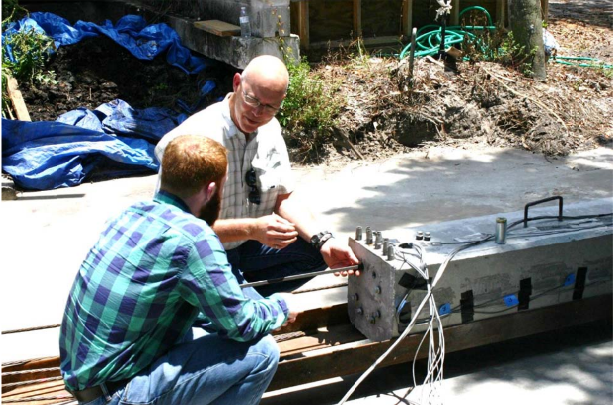
Figure 4.86. 48in long rod used to check anchorages by compression wedge assembly spring.
