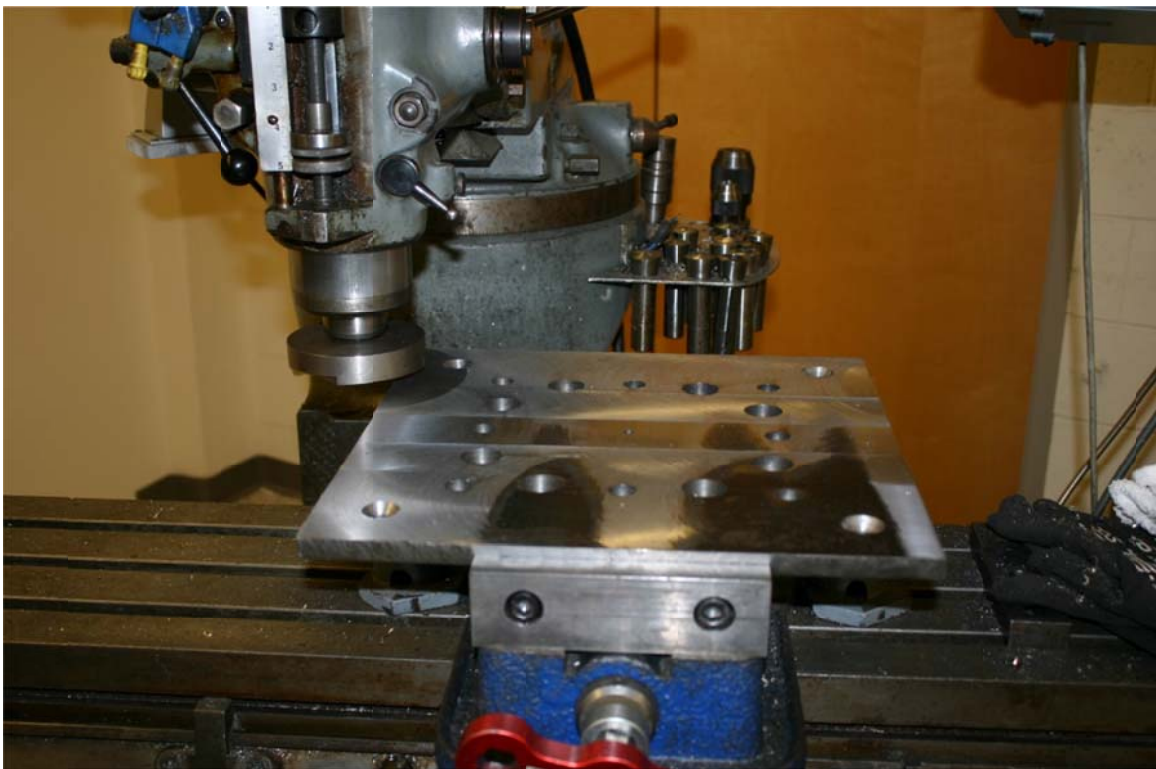
Figure 3.20. Milling header plates to provide smooth, parallel contact surfaces.
