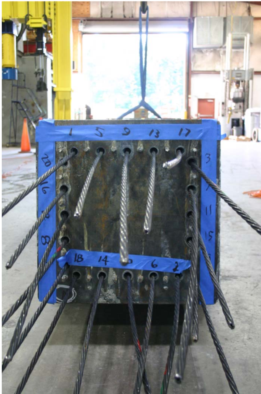
Figure 5.16. Splice stressing order of matched pairs
