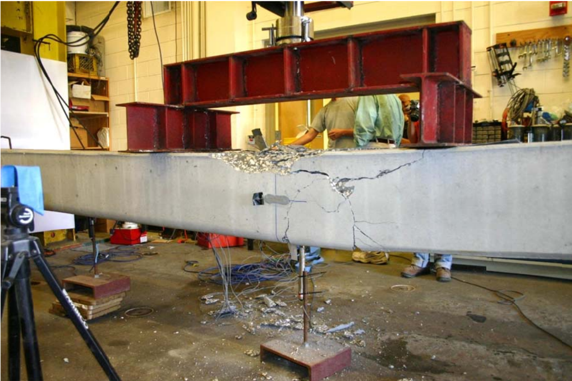
Figure 4.116. Control Pile 2 before and after testing. Again compression block well below spiral level. Failure load 39kips.
