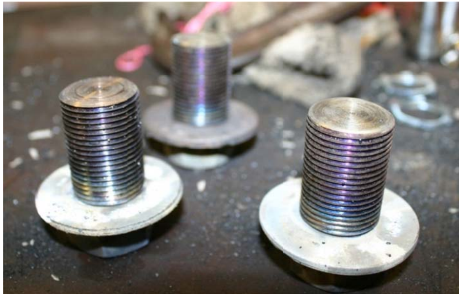
Figure 4.64. Duct inserts were fabricated to prevent debris from getting into the ducts.
