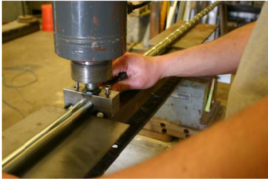
Figure 4.63. Duct deformation in purpose-built hydraulic stamping press.
