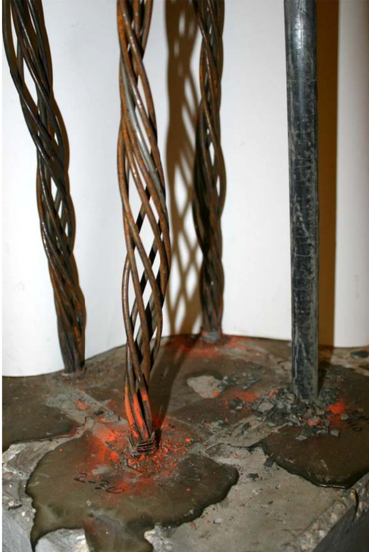
Figure 4.125. Strand pullout specimens: 1in x 40in (back); 2in x 40in (left); smooth (right); and 2in x 30in (front).
