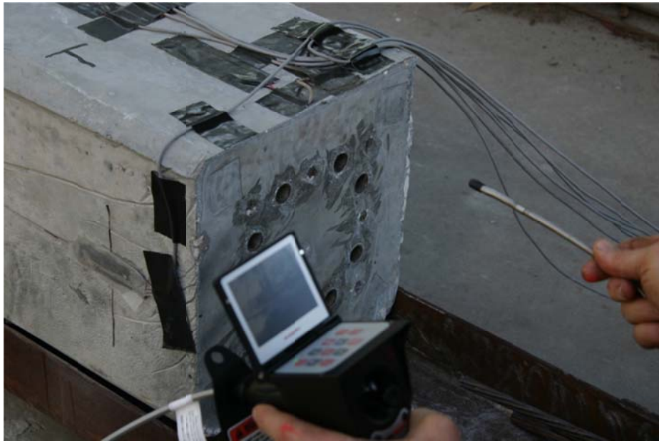
Figure 4.45. Borescope with 360 degree articulating viewing head.
