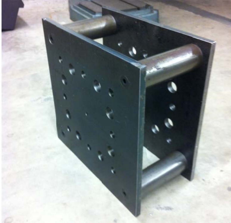
Figure 3.21. Finished splice header assembly.
