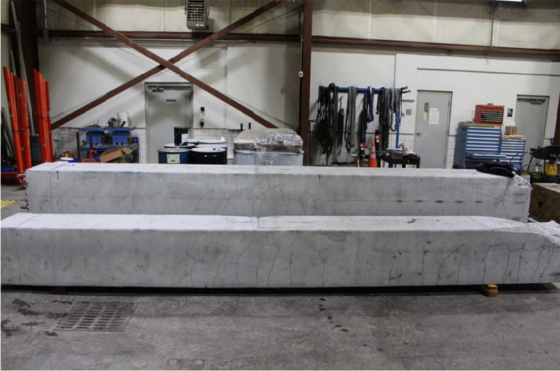
Figure 5.33. Three-point specimens after testing (control foreground; splice background).
