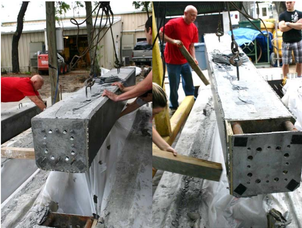
Figure 4.79. Splice pile specimen: lower segment (left), splice header still attached to upper segment (right).
