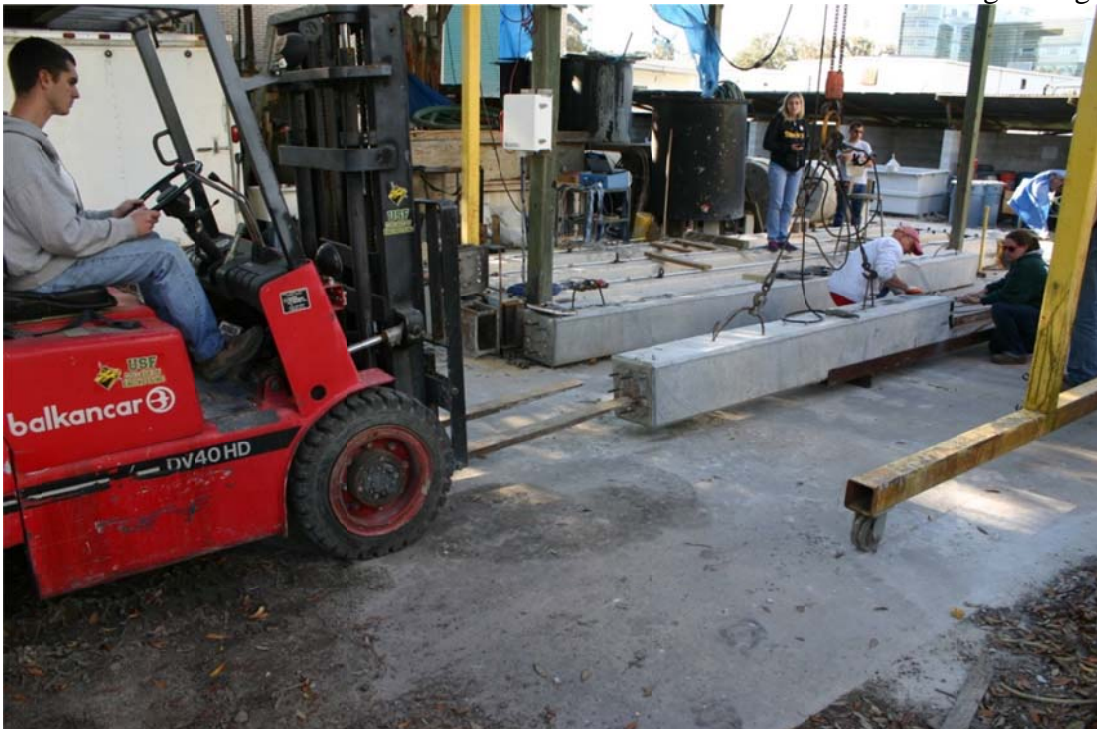
Figure 4.53. Weight of moving segment held by overhead crane while fork lift pushed the segments together and while each strand was sequentially inserted into the lower segment ducts.
