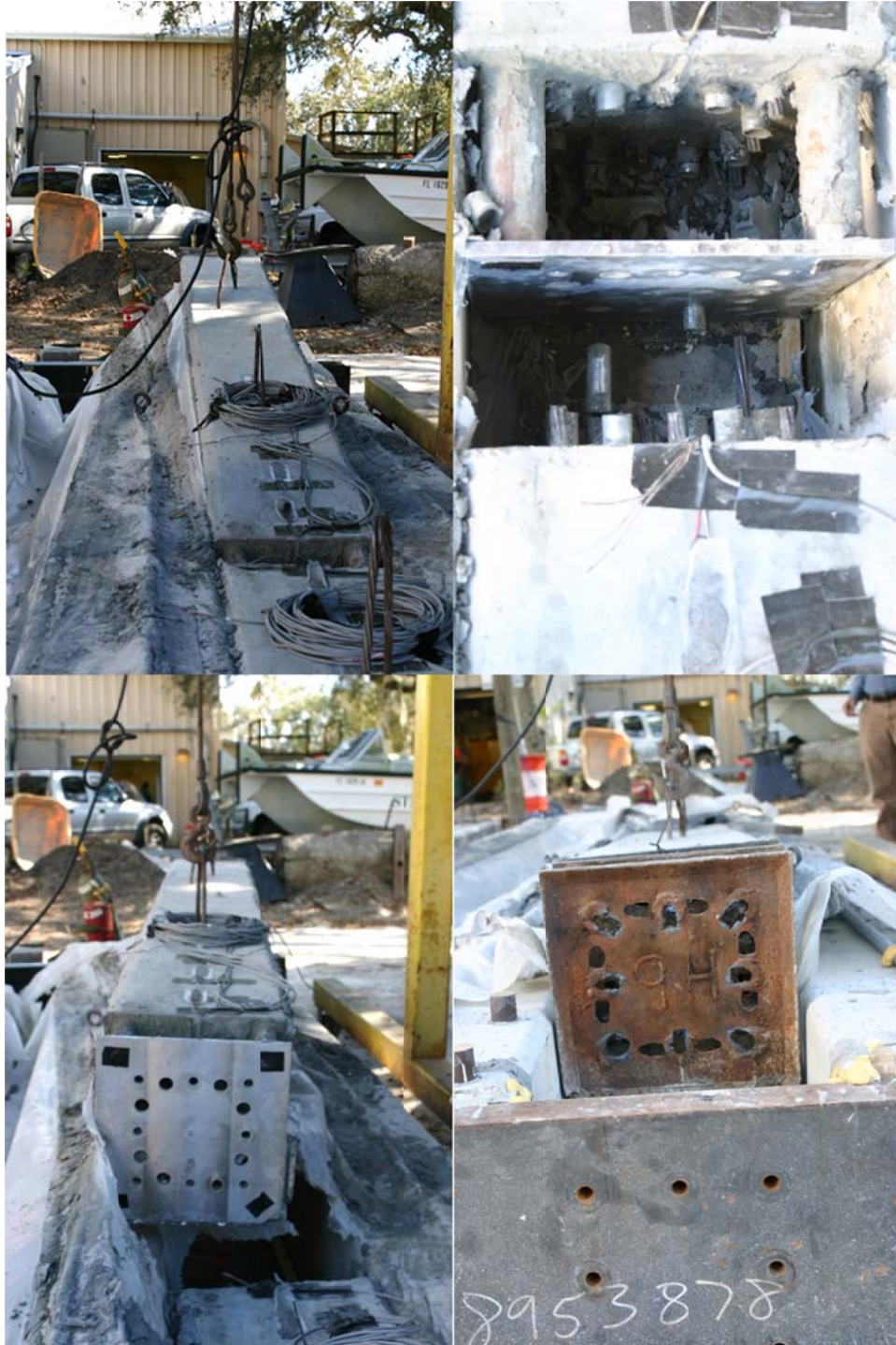
Figure 4.40. Splice pile specimen: lower segment breaking loose (TL), splice header separation (TR), lower segment with splice header (BR), upper segment with end of bed header (BR).
