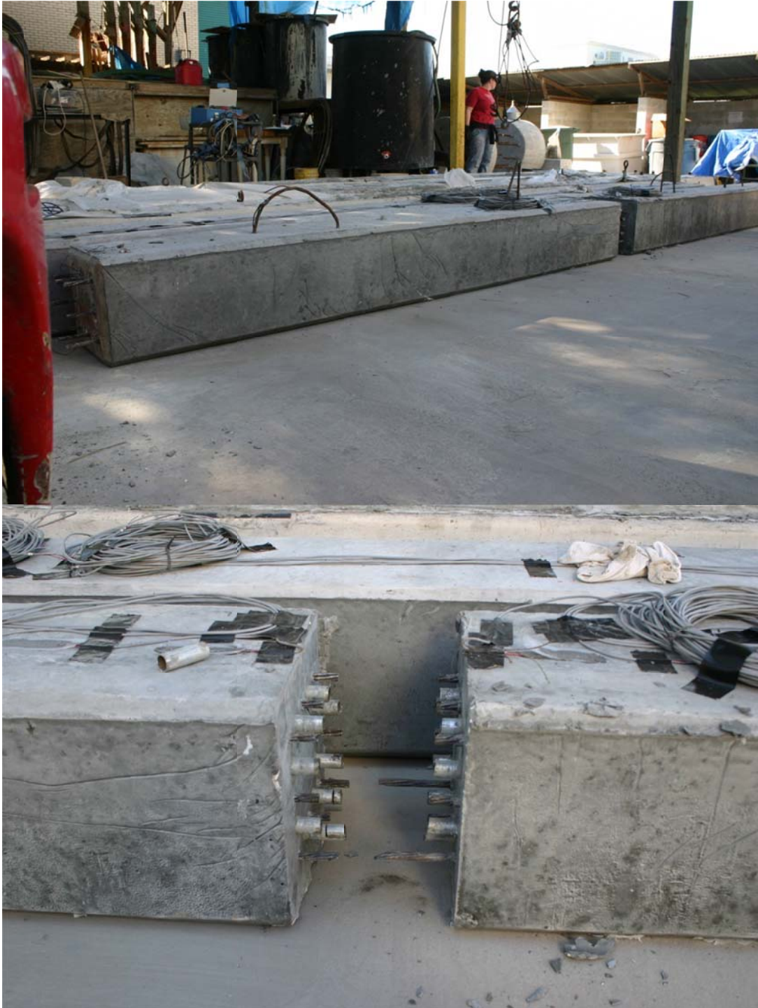
Figure 4.41. Extracted piles before grinding off duct and strand stubs.
