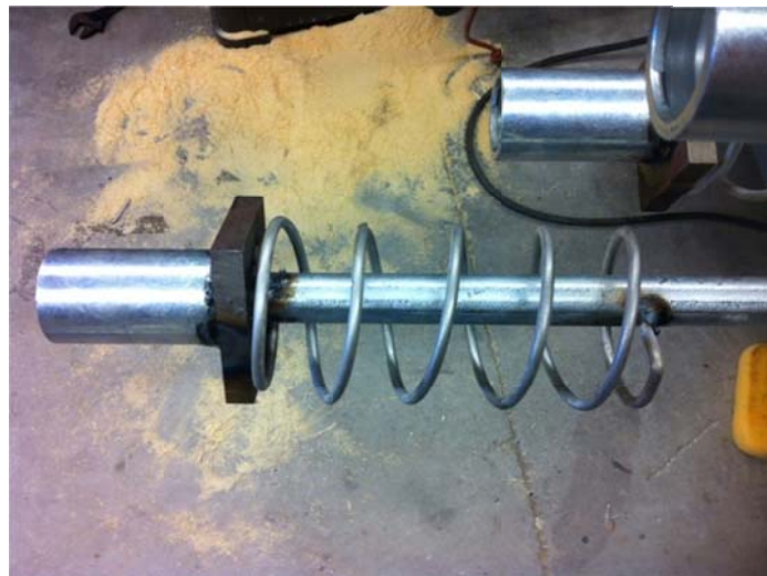
Figure 4.19. Confinement coils used to bolster local concrete stresses in the field identified by modeling.
