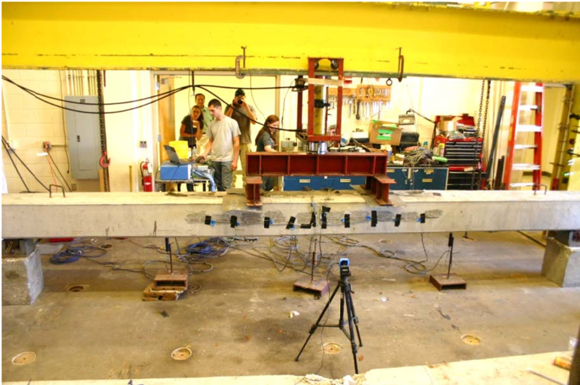
Figure 4.109. Four-point bending set up (control top; splice bottom).
