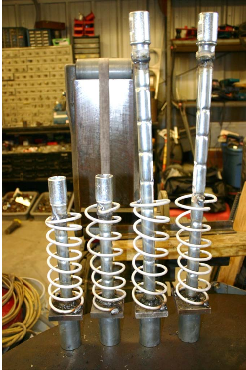
Figure 4.65. Confinement coils used to bolster local concrete strength welded to anchorages in regions of high anticipated stresses.
