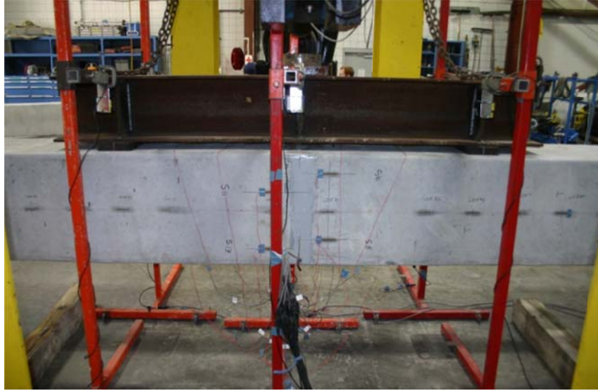
Figure 5.26. Spreader beam with neoprene loading points set at 6.5 ft.
