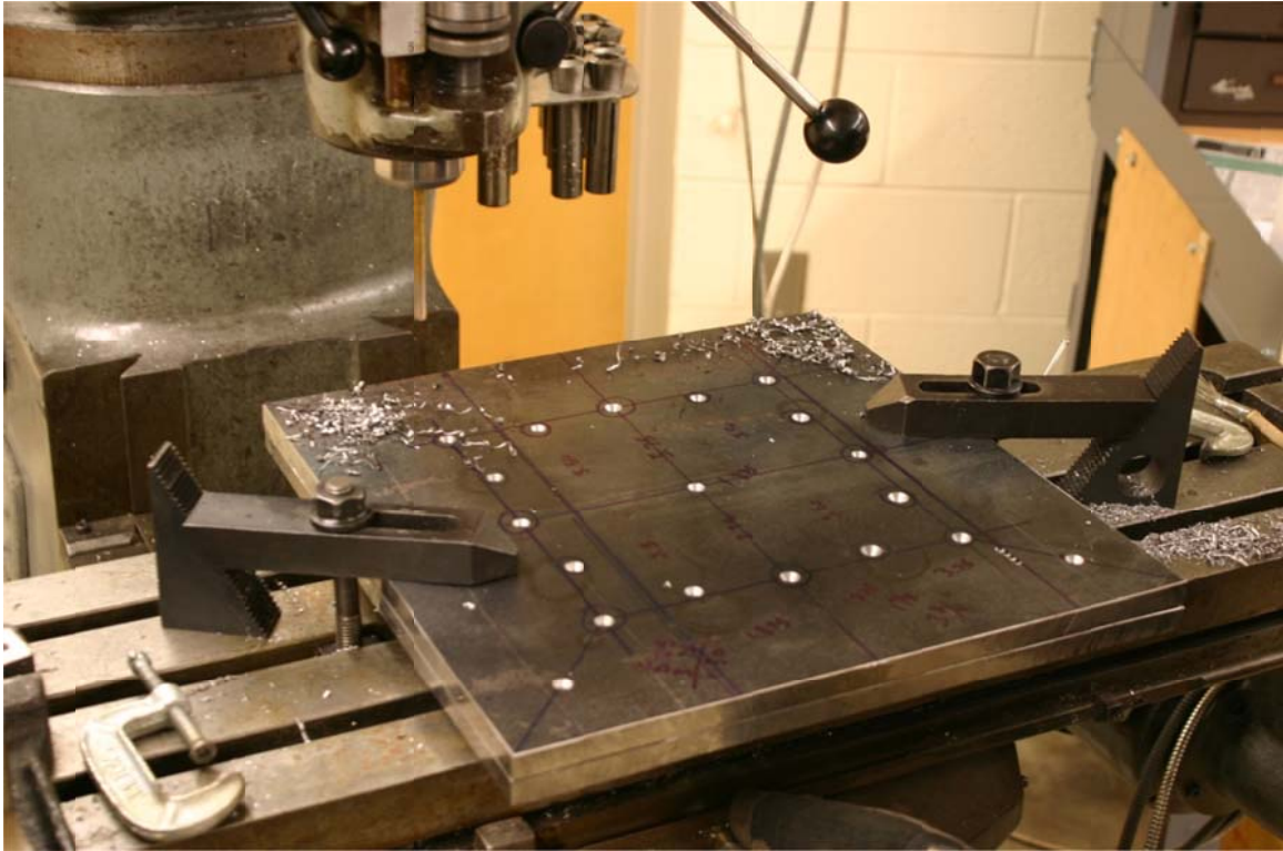
Figure 3.19. Drilling locations for strands and ductwork into the splicing header.
