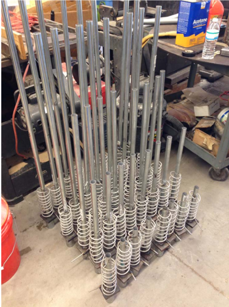
Figure 5.2. Forty confinement coil, chuck and duct assemblies.
