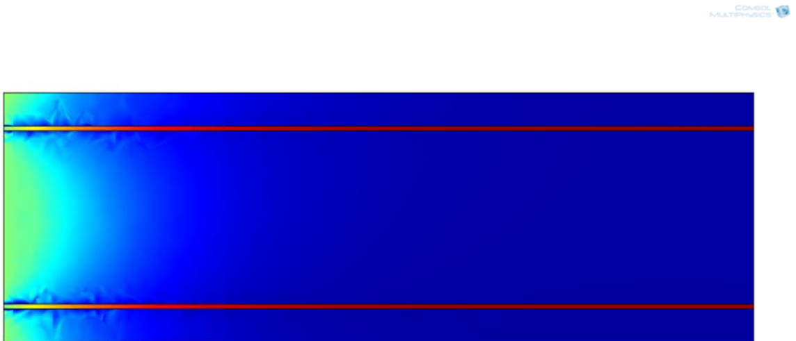
Figure 3.9. Model solution, longitudinal stress variation along mid-plane of pile (blue = compression, red = tension)
