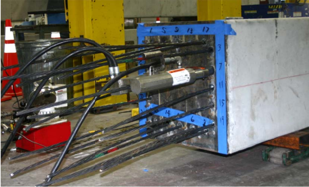
Figure 5.17. Post tensioning of splicing strands.
