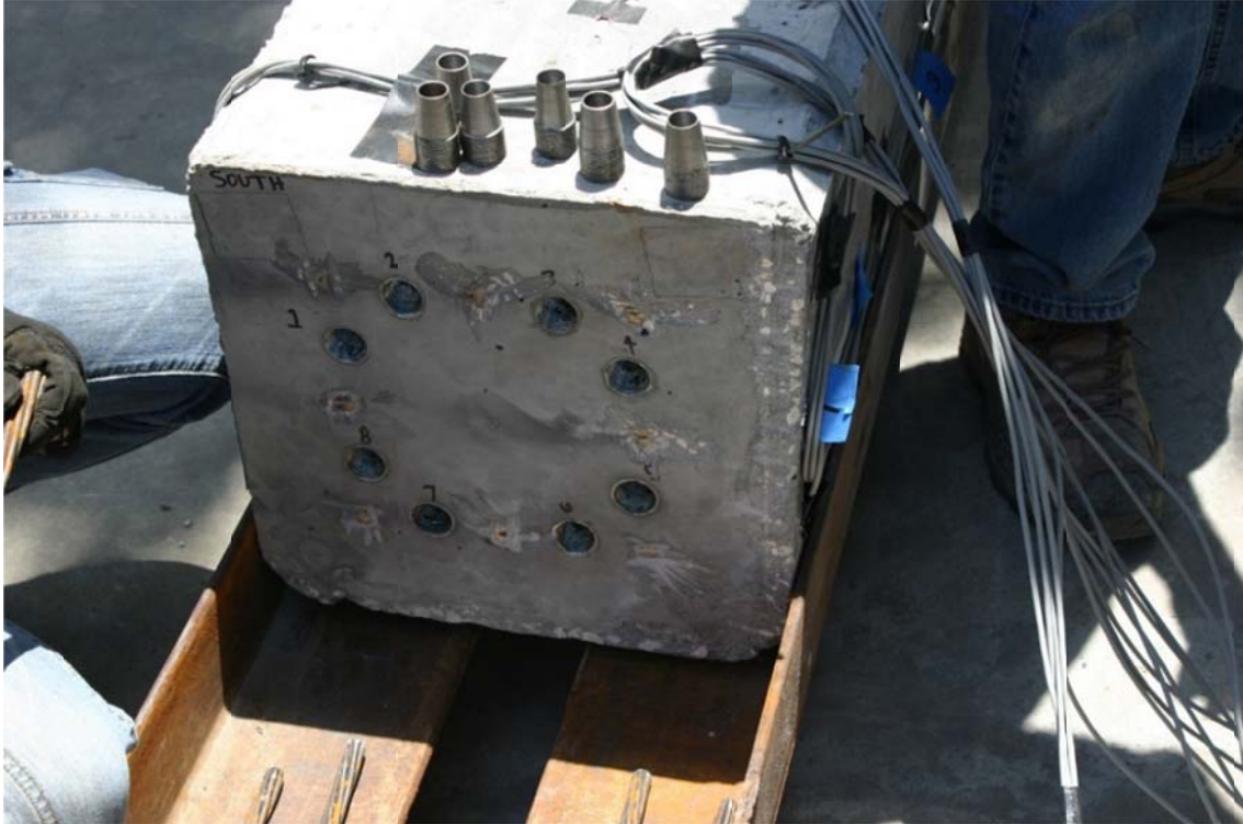
Figure 4.92. Lower pile segment aligned with upper segment on splicing rail.
