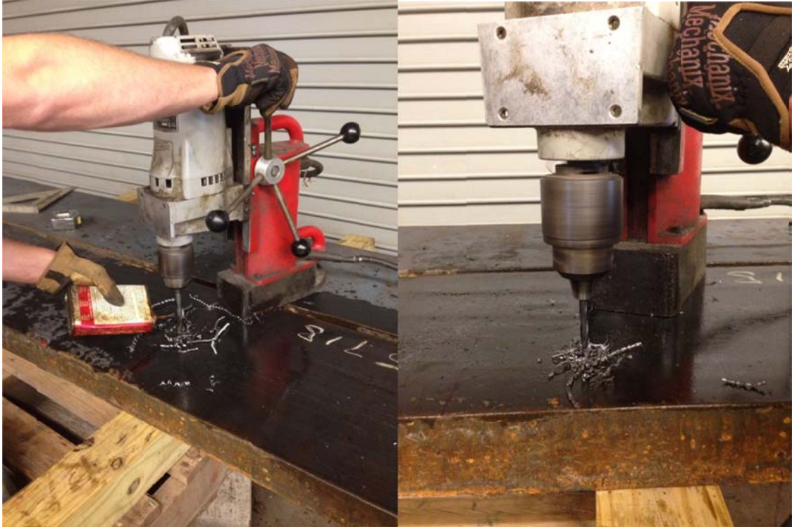
Figure 4.10. 2.5in thick header plates drilled for standard 14in strand pattern.
