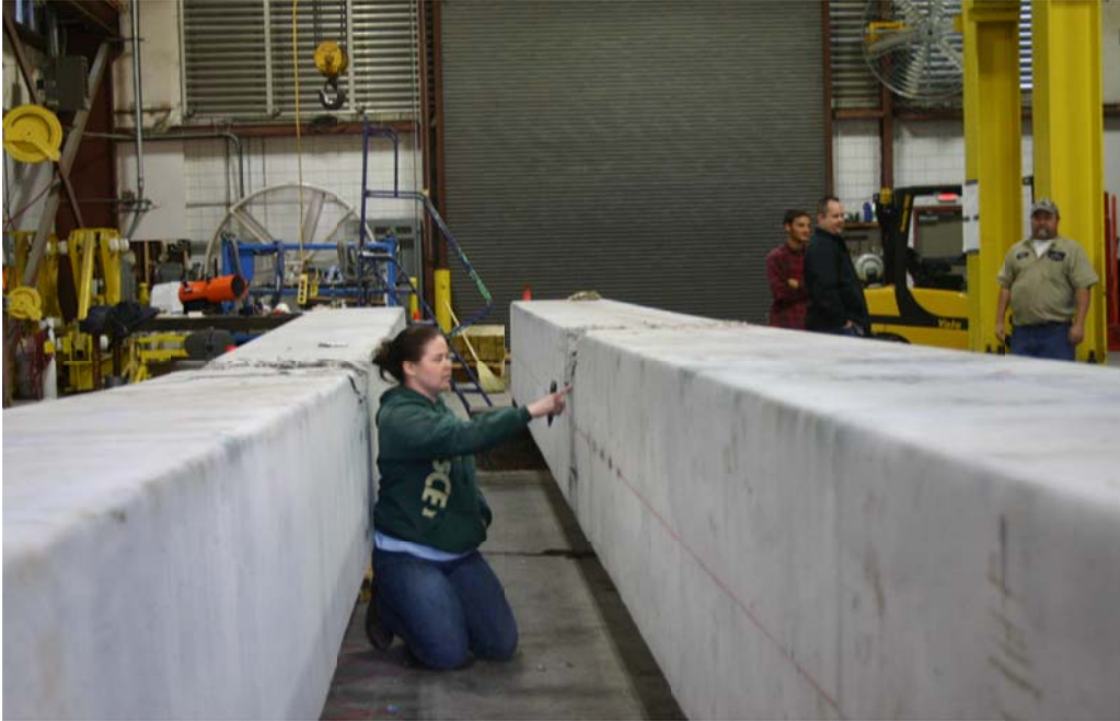
Figure 5.28. Smaller permanent deformation of spliced pile (right); control (left) after testing.
