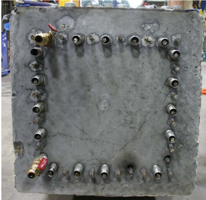
Figure 5.23. Duct ends fitted with 3/4in pipe nipple and/or ball valve.
