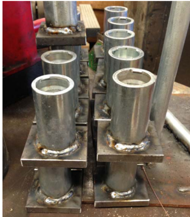
Figure 5.1. Chucks welded to bearing plates.
