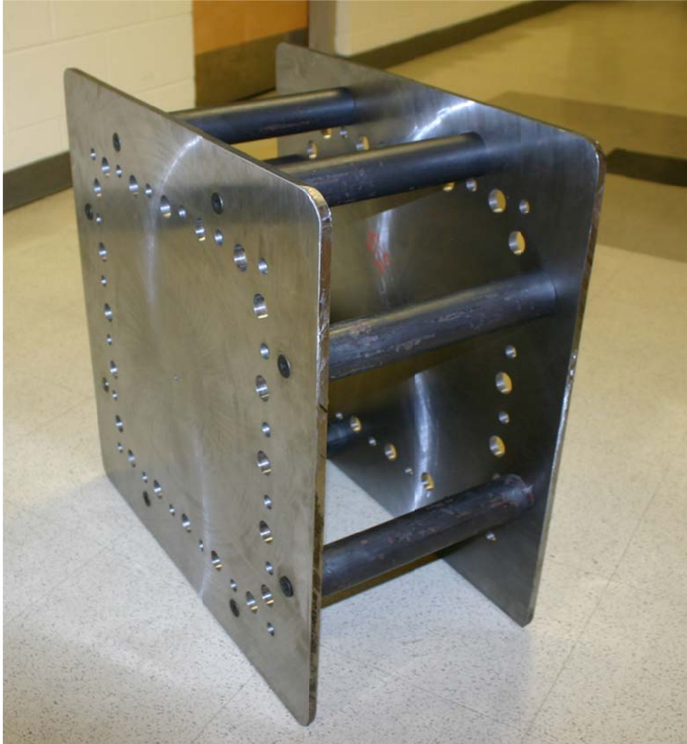
Figure 5.4. Finished header plate assembly.
