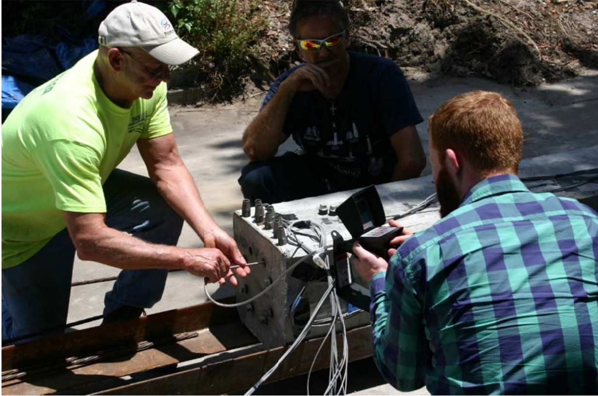
Figure 4.87. Borescope with 360 degree articulating viewing head.
