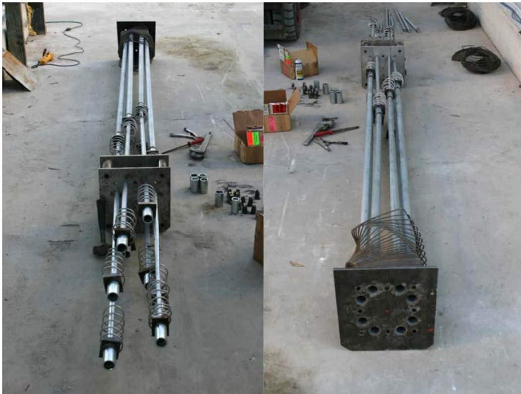
Figure 4.18. Splice header with splicing ducts and extension ducts to the top of pile jacking plate.
