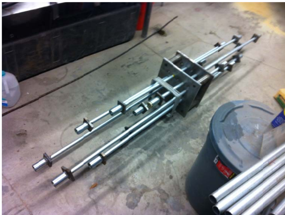
Figure 3.26. Splice header with staggered ducts and embedded chuck assemblies; all ducts are the same length.
