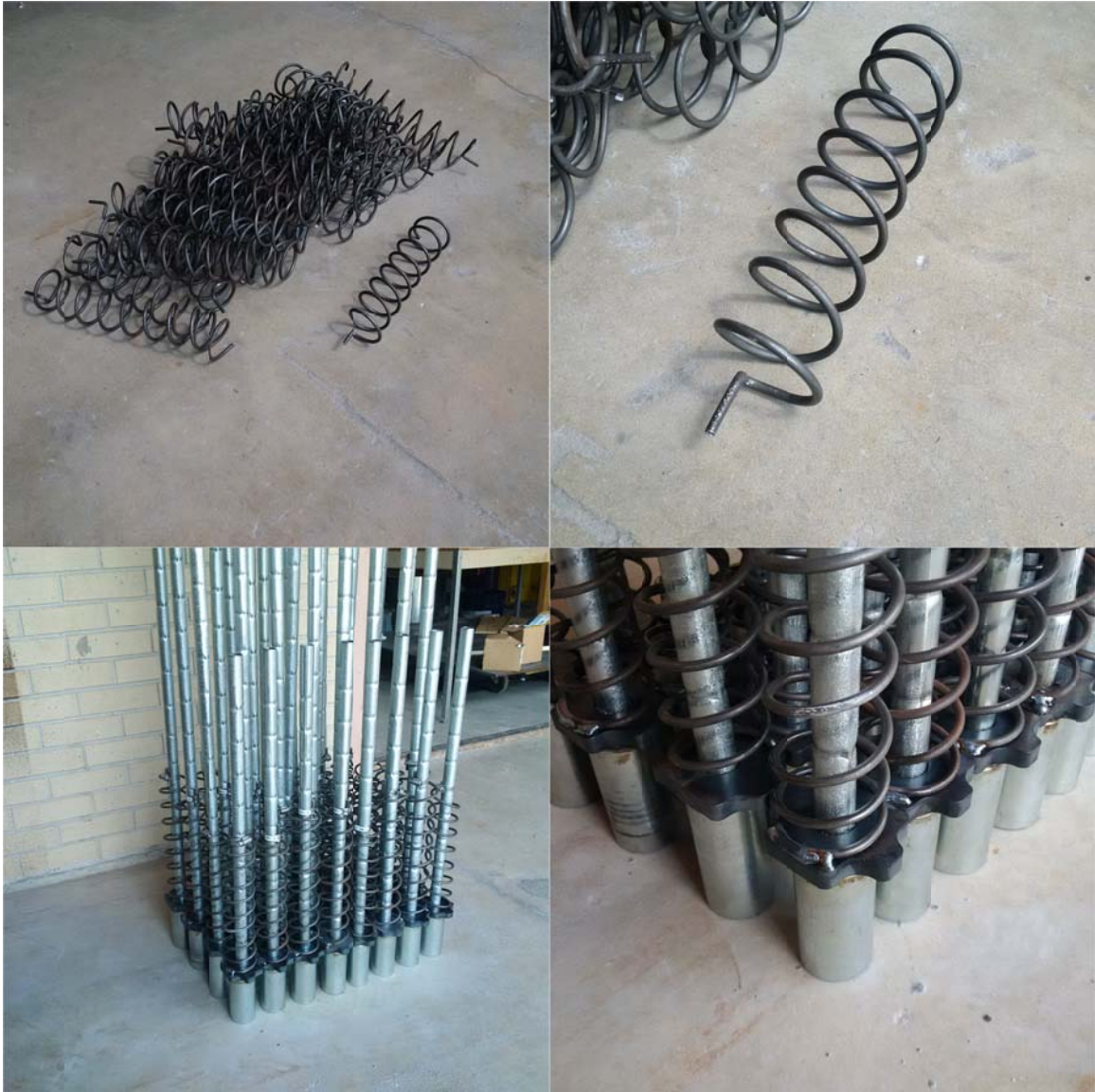
Figure 6.4. 32 confinement coils before and after assembling into completed anchorages.
