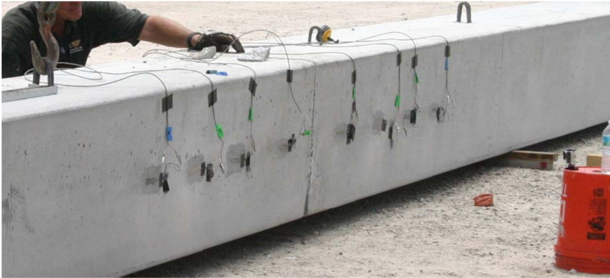
Figure 6.25. Strain gages mounted on both sides of each pile 13.5, 35, 51, and 67in from splice.
