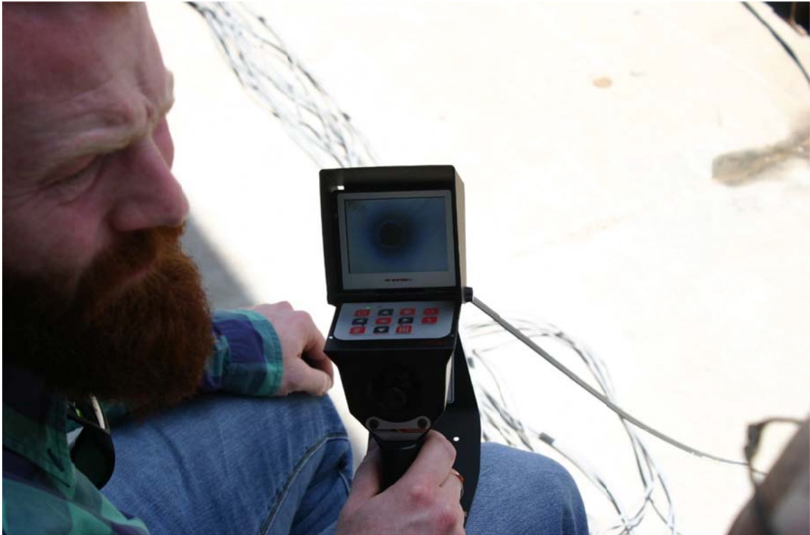
Figure 4.88. Real-time imaging of duct cleanliness.
