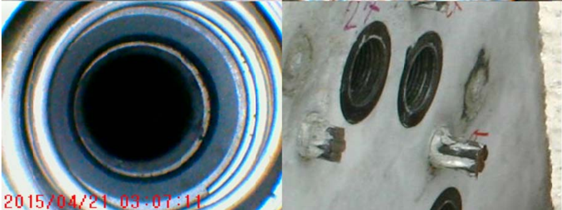
Figure 6.16. Borescope inspection showed no debris in wedges.
