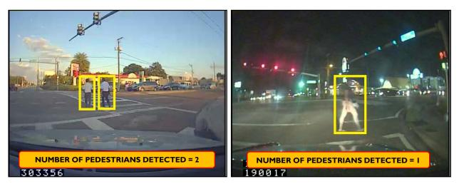
Figure 10. Example of pedestrian detection and tracking
