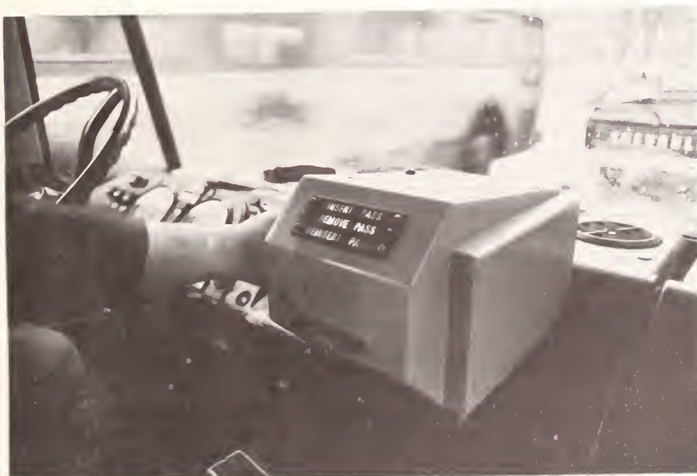
Automatic fare identification recorder used in Portland, Oregon for credit card postpayment.
