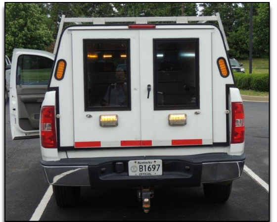
Figure L: Vehicle #6 (Rear), White/Amber Flashing
