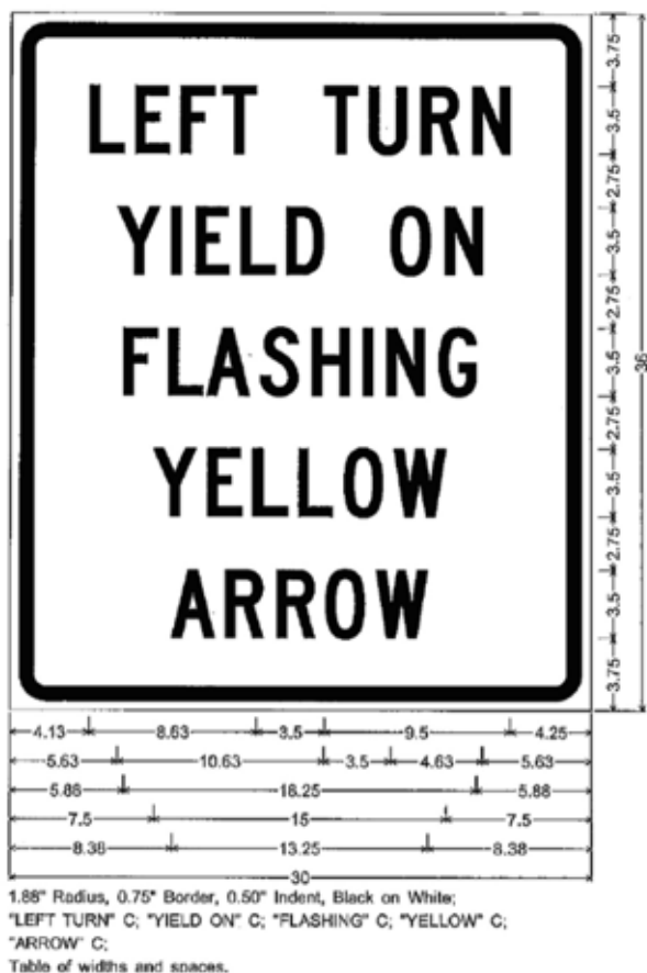
Figure 5.1 INDOT FYA supplemental sign.
