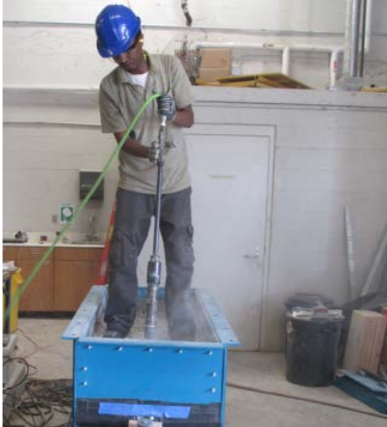
Figure 4.1: Compaction of the Test Sample
