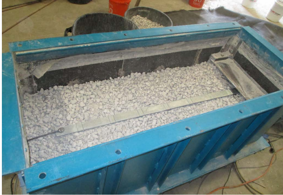
Figure 4.2: Ribbed Steel Strip Reinforcement Placed On Top of the First Layer
