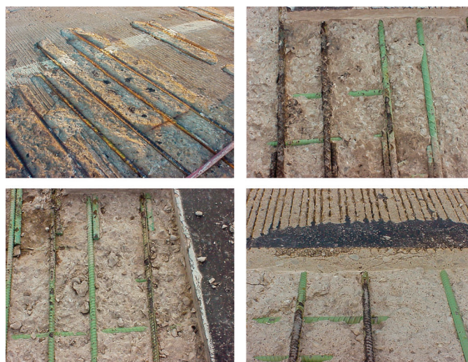
Figure 1.1 Corrosion of epoxy-coated reinforcing steel (photos courtesy of INDOT).
