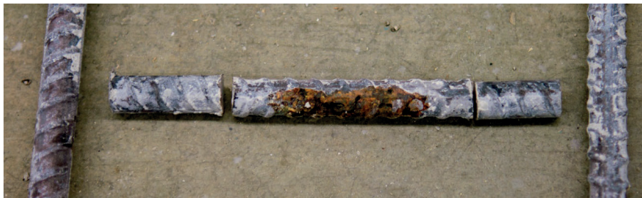
(e) Microcell Corrosion on Top MMFX II bar
