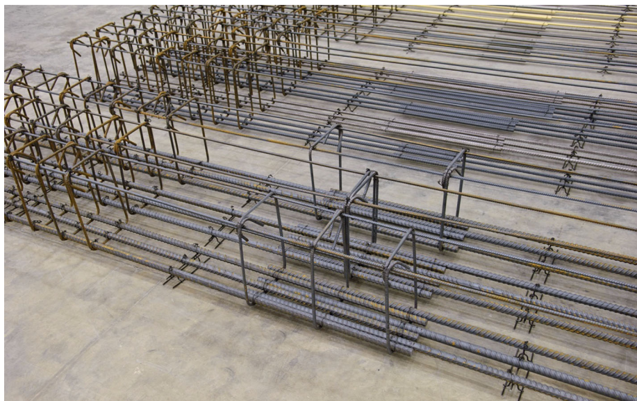
Figure B.16 Details of the reinforcing bar in splice region (series IV).
