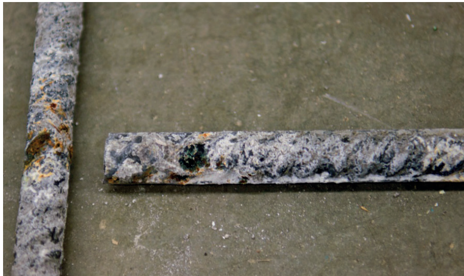
(b) White Corrosion and Iron Oxide Corrosion on Galvanized Bar
