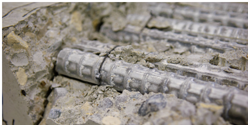
Figure C.17 Concrete attached to tin-plated zinc-clad bars (ZC2-8-S-24).
