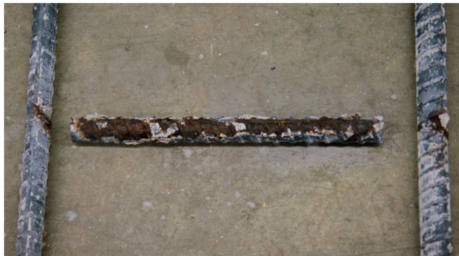
(b) Corrosion on Bottom Black Bars
