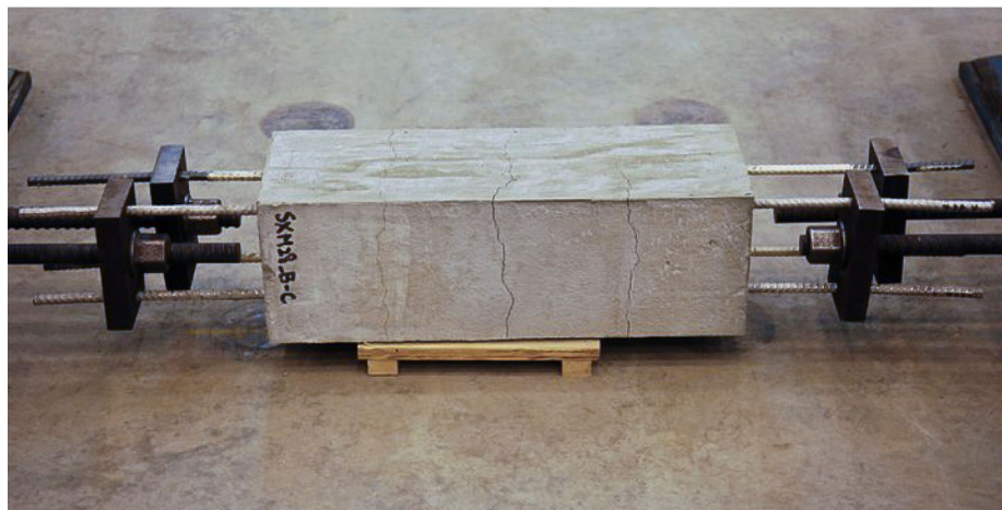
Figure F.15 Typical cracked specimen with dissimilar bars.
