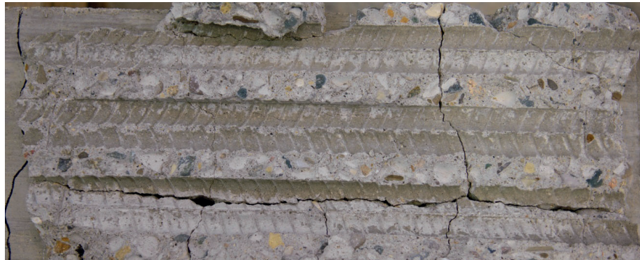
(b) Concrete Cover Removed from Hot-Dip Galvanized Bars
