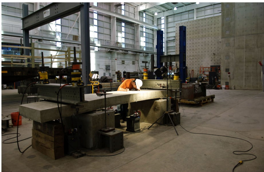
Figure D.7 Measuring cracks during testing (specimen B-12).
