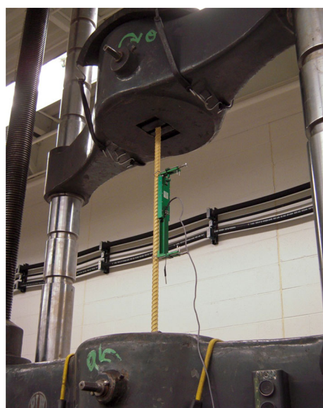
Figure A.2 Test setup for rebar coupon tension test.
