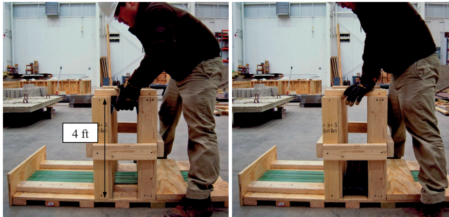
Figure F.7 Creating coating damage.
