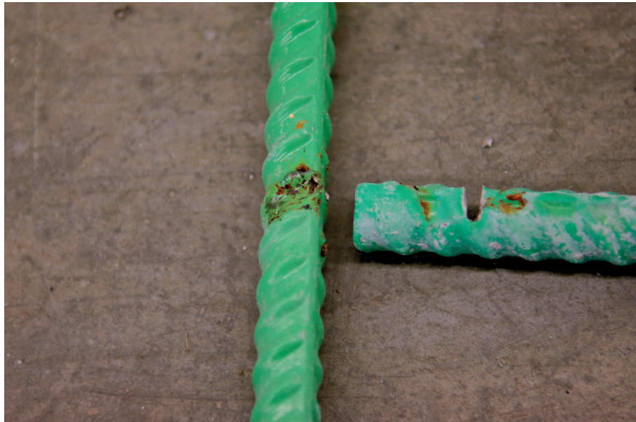
(d) Corrosion Where Steel Was Tied with Black Tie
