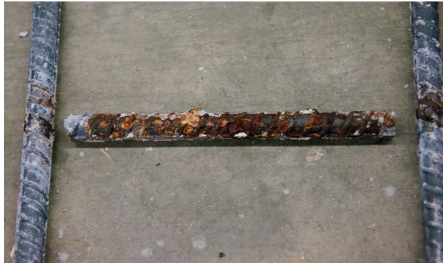
(b) Corrosion on Bottom Black Bars
