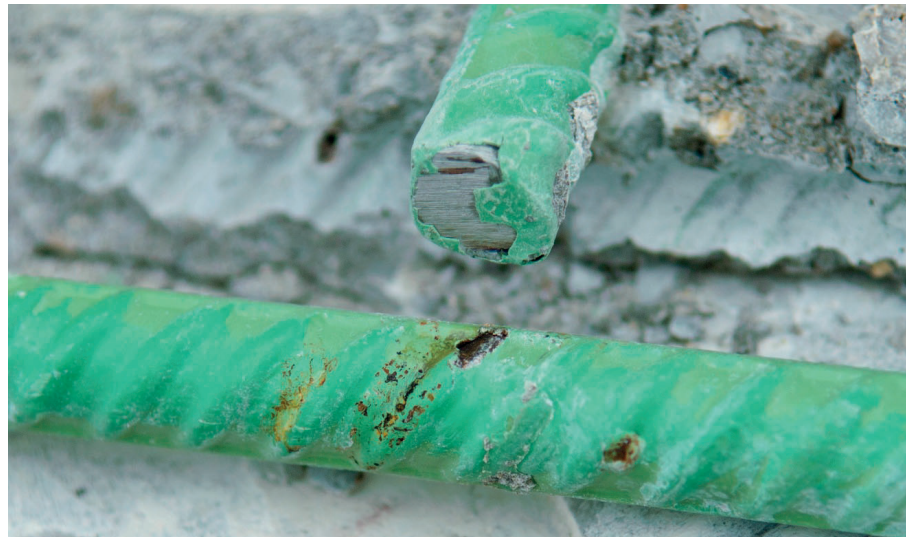
(b) Corrosion on Epoxy-Coated Steel
