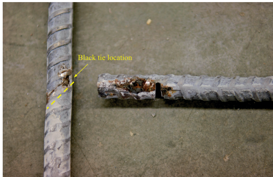
(b) Corrosion where Stainless Steel was Tied with Black Tie
