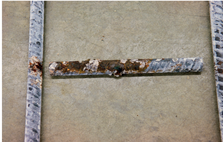
(b) Corrosion on Top Longitudinal and Transverse Steel
