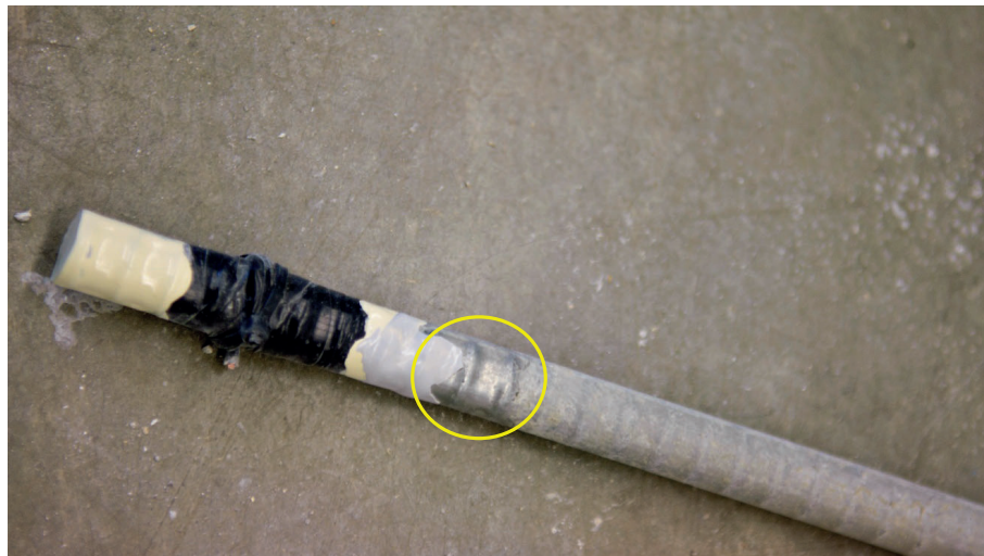
(b) Remaining Pure Zinc Outer Layer
