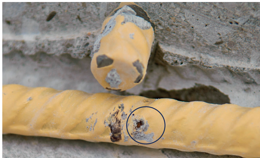
(b) Corrosion of Base Metal at Damaged Location
