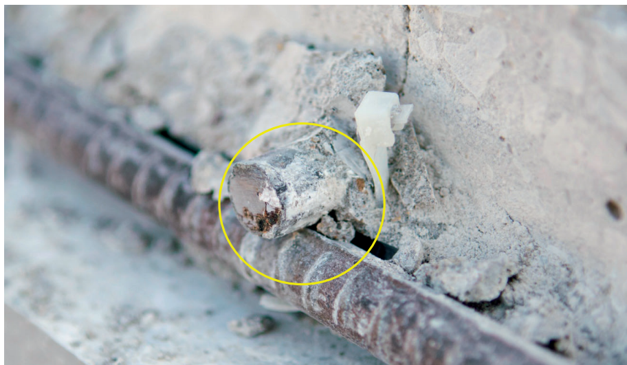
(b) White Corrosion and Consumption of Tin-Plated Zinc Clad
