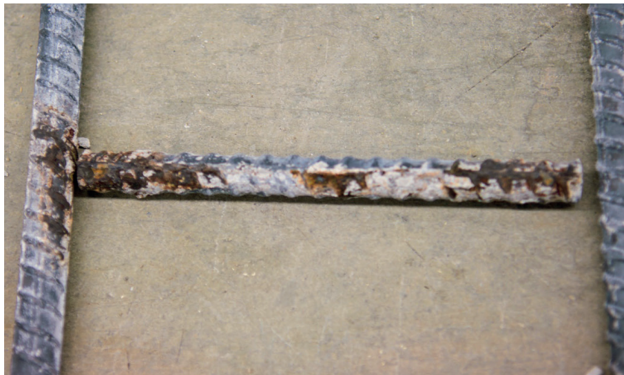
(b) Corrosion on Bottom Black Bars
