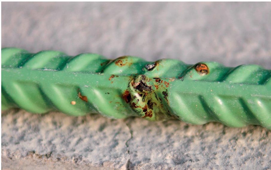
(b) Corrosion on Longitudinal Bar with Black Ties
