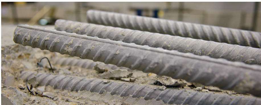
Figure C.11 Adhesion of concrete to XM-28 stainless steel bars.
