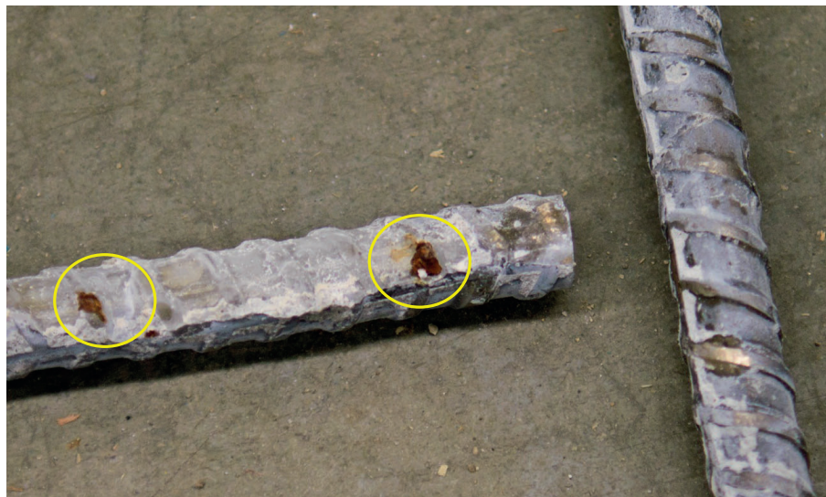
(b) Corrosion Products on Transverse Steel
