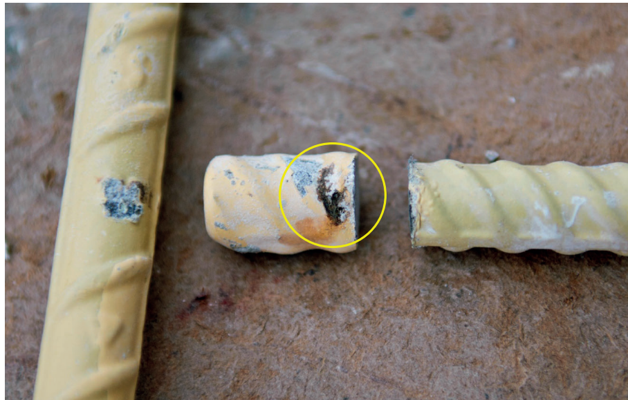
(b) Corrosion on damaged area
