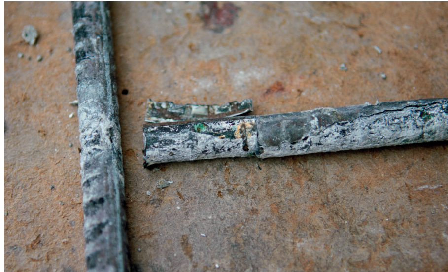
(b) White Corrosion of Zinc, Consumed Zinc Cover, and Peeled off Cover
