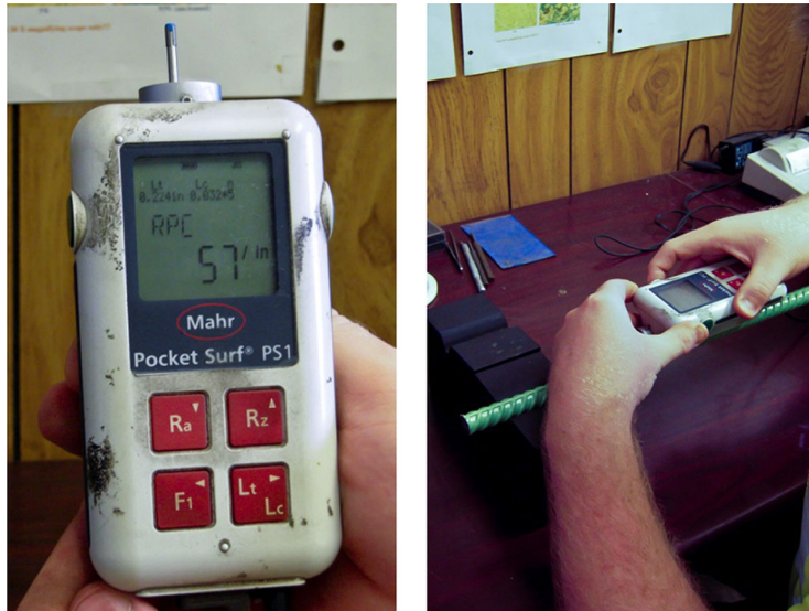
Figure A.7 Surface roughness measurement (profilometer).
