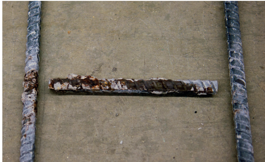
(b) Corrosion on Bottom Black Bars
