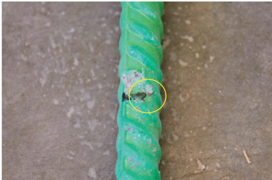
(b) Corrosion on Damaged Epoxy-coated Bar
