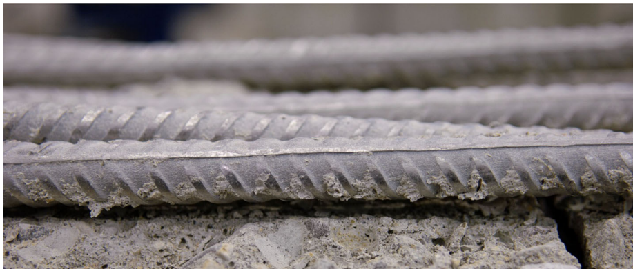
Figure C.10 Adhesion of concrete to Duplex 2304 stainless steel bars.
