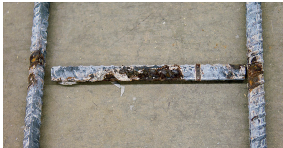
(b) Corrosion on Bottom Black Bars
