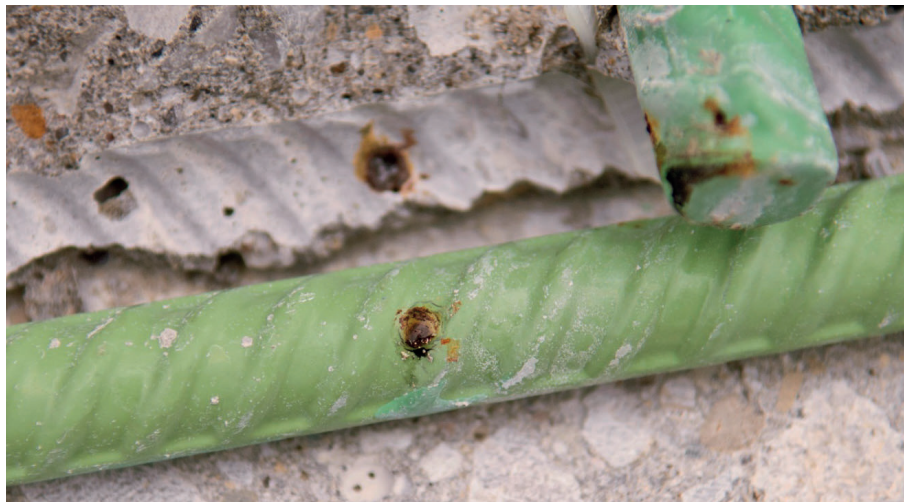
(b) Corrosion on Epoxy-coated Bar
