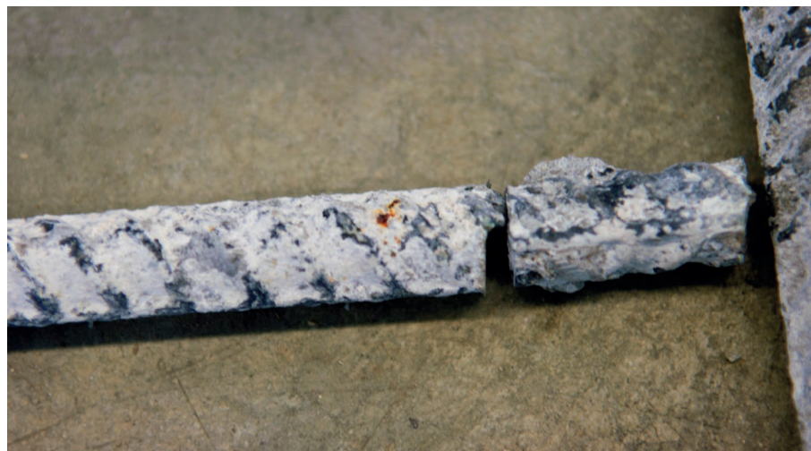
(b) White Corrosion products of Zinc and Corrosion spot of Underlying Base Metal
