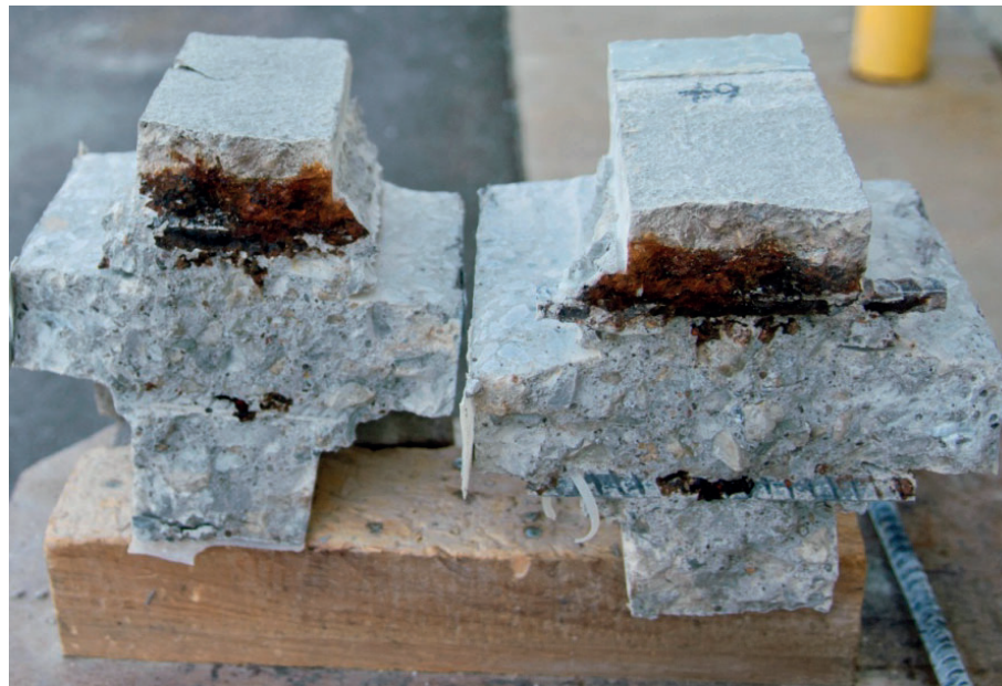
(b) Corrosion Shown at Crack Location (Top Transverse Bars)
