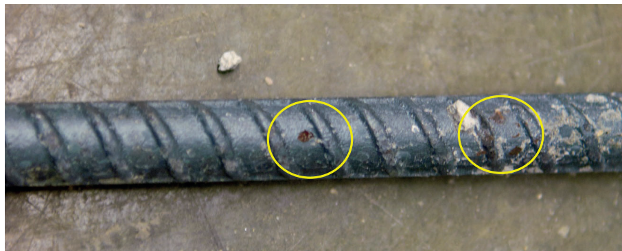
(b) Light Corrosion on Black Bar
