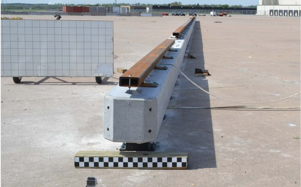
Figure 67. Barrier Stability with Steel Pipe Inserts
