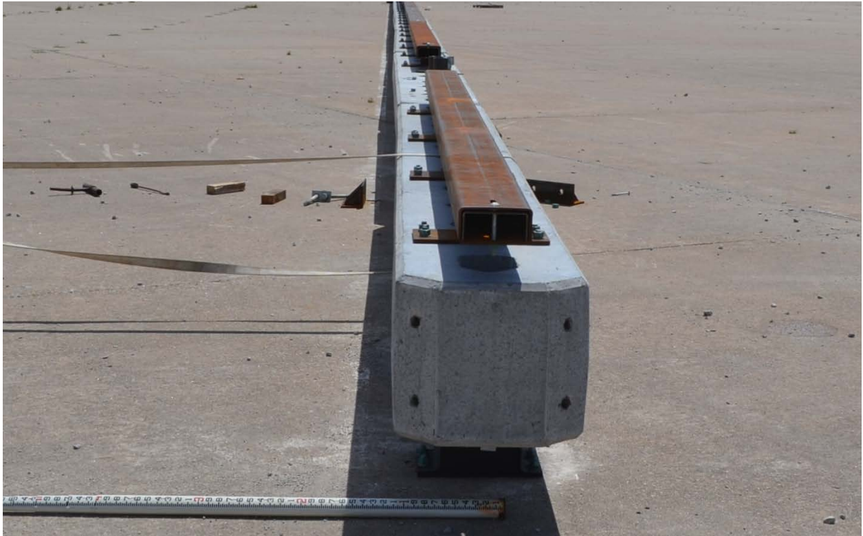
Figure 70. Barrier Stability with Two Support Skids with Shims
