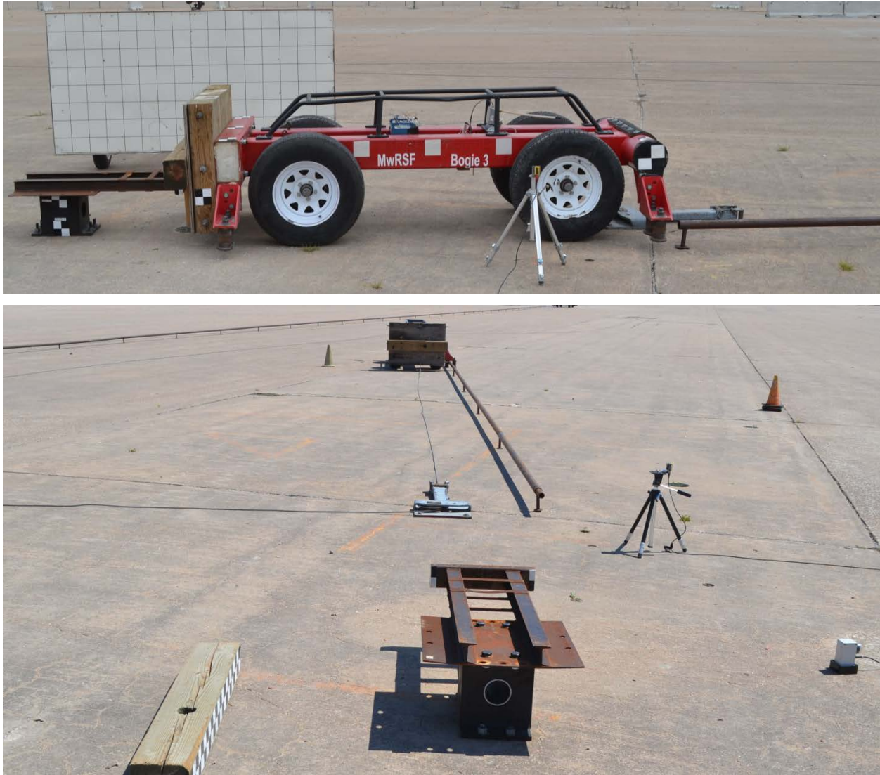
Figure 23. Rigid-Frame Bogie on Guidance Track
