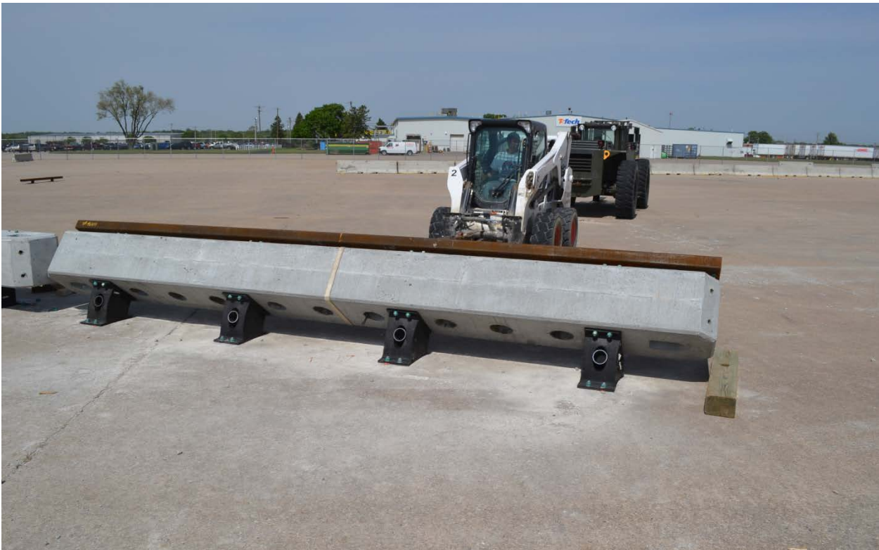
Figure 68. Barrier Deflection with Steel Pipe Inserts
