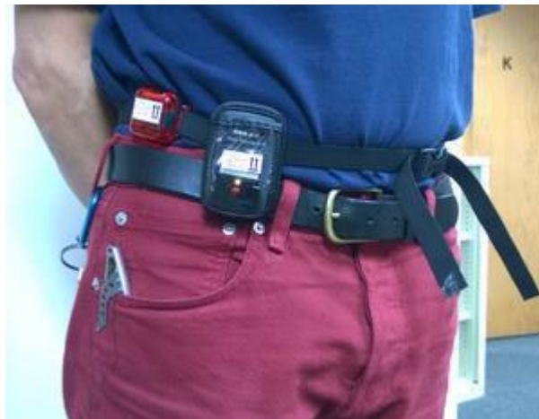
Figure 3-1: Position of accelerometer and GPS
