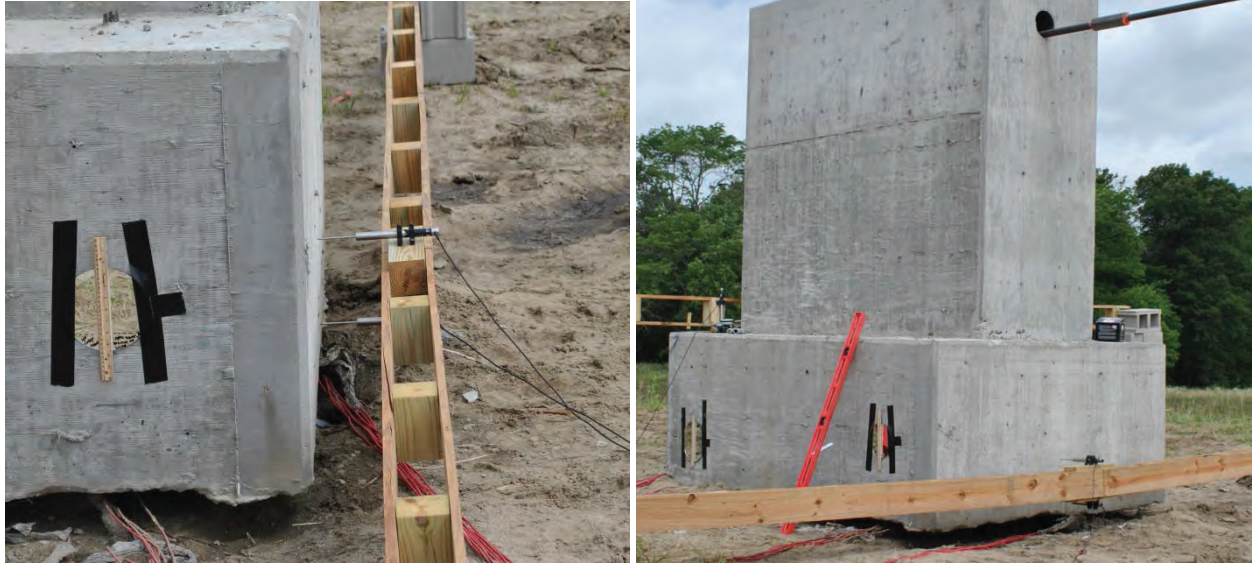
Figure 3.43. LVDTs positioned against front of pile caps to measure lateral deflection. One LVDT was mounted directly above the other to measure rotation.
