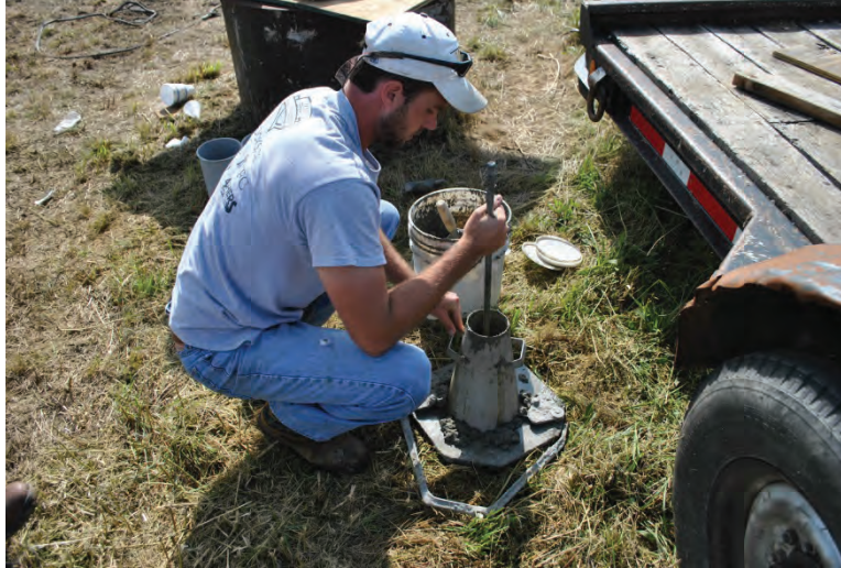
Figure 3.27. Performing slump test in accordance with ASTM C143 (2012) on concrete from each pour.
