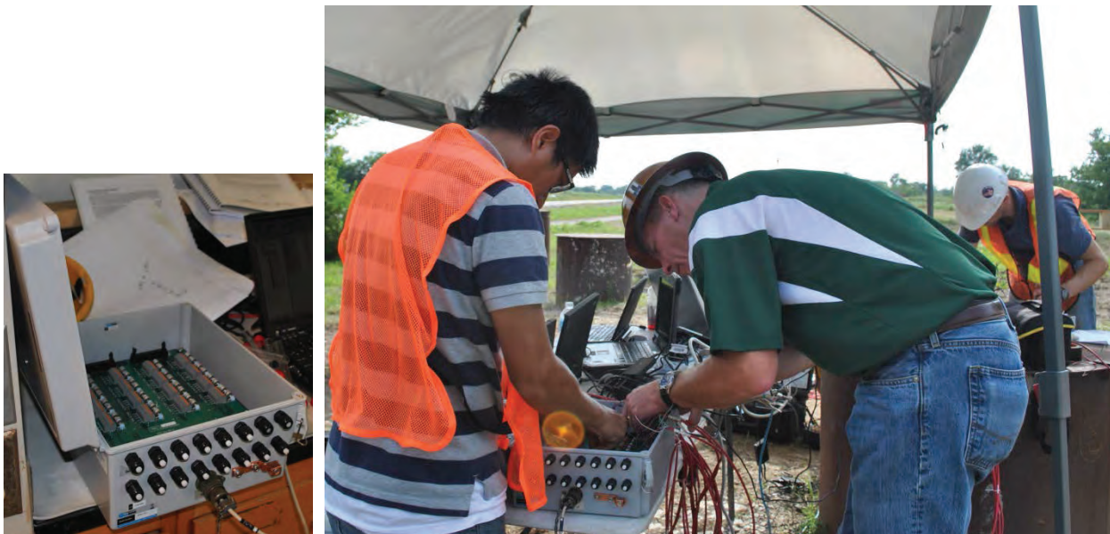
Figure 3.39. Geokon datalogger LC-2x16 in lab (left) and field (right).
