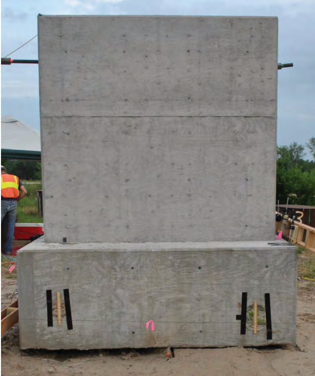
Figure 3.56. H-pile cap during the final load step.
