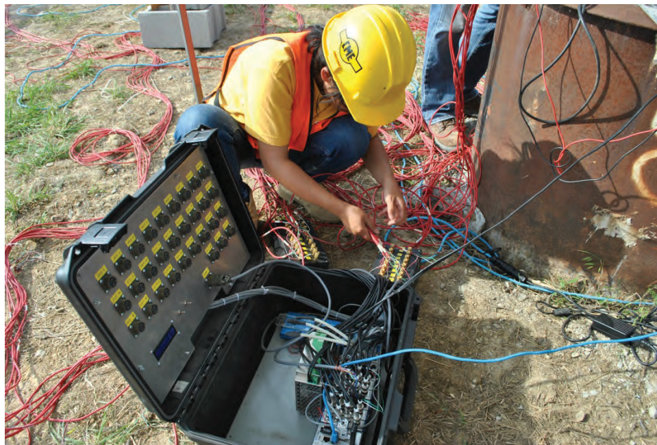
Figure 3.37. DAQ used to read Geokon 4000 gages (Luna, 2014).
