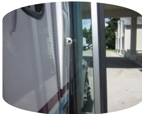
Figure 4-14: Security Camera Mounted on Outside of Transit Vehicle at Council on Aging of St. Lucie, Inc.
