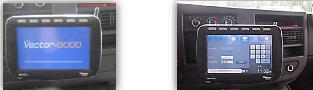
Figure 4-1: MDT (AVAIL Vector 9000) Mounted on Front of Dashboard on Collier Area Transit Vehicles
