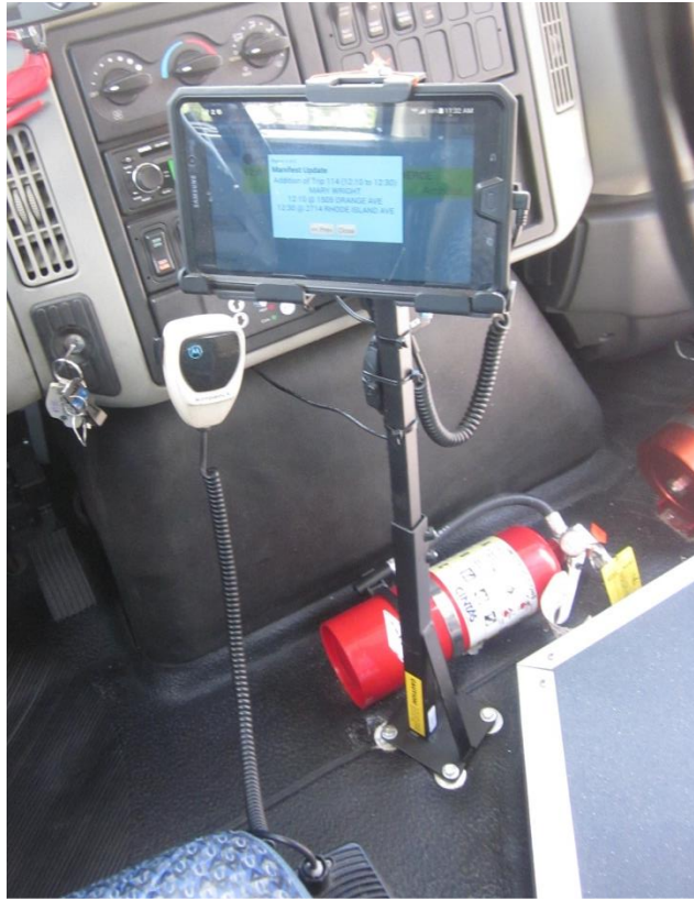
Figure 4-10: New MDT Tablet Mounted on Stand Secured to Floor of Vehicle and Old MDT Ranger Unit Mounted on the Dashboard
