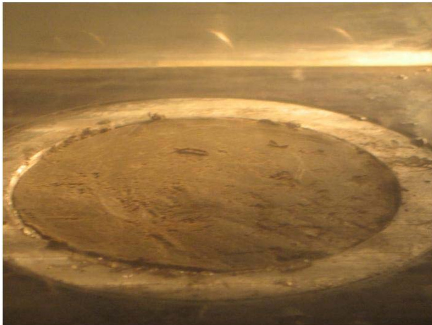
Figure C-23. Porter’s Creek 24.0_4 Sample at Start of 0.3 m/s EFA Test.
