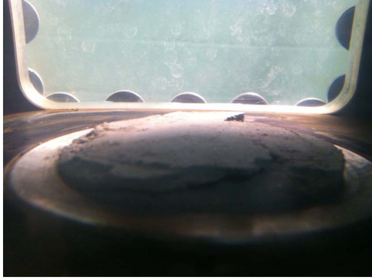
Figure B-6. Yazoo Clay 18.5_2 Test Swelling and Cracking
