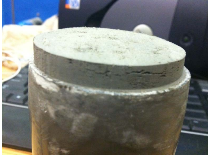
Figure B-16. Prairie Bluff Chalk Formation Cracking Example 1
