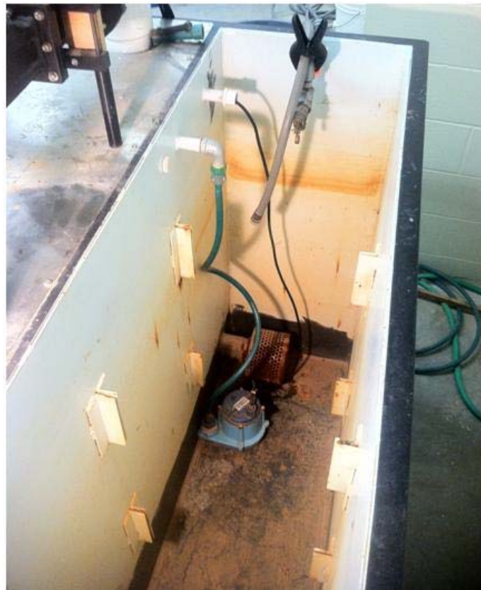
Figure 2-2. EFA Reservoir with Water Circulation to Control Water Temperature.
