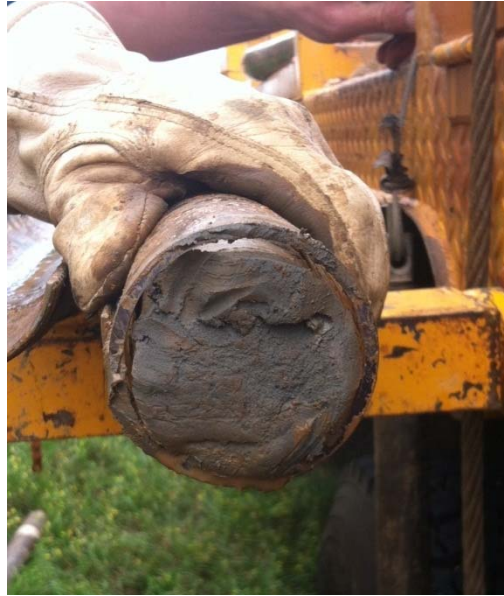
Figure B-1. Bucatunna Clay Sample Smaller Radially than Sample Tube
