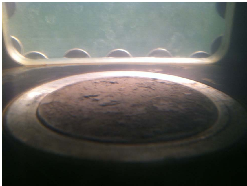
Figure 2-10. Soil Sample in EFA Level with Base of Flume.
