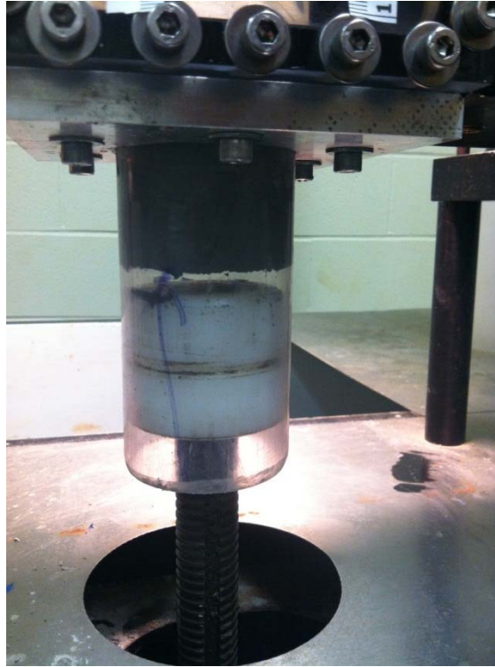
Figure 2-9. Soil Plunger Advancing Sample.
