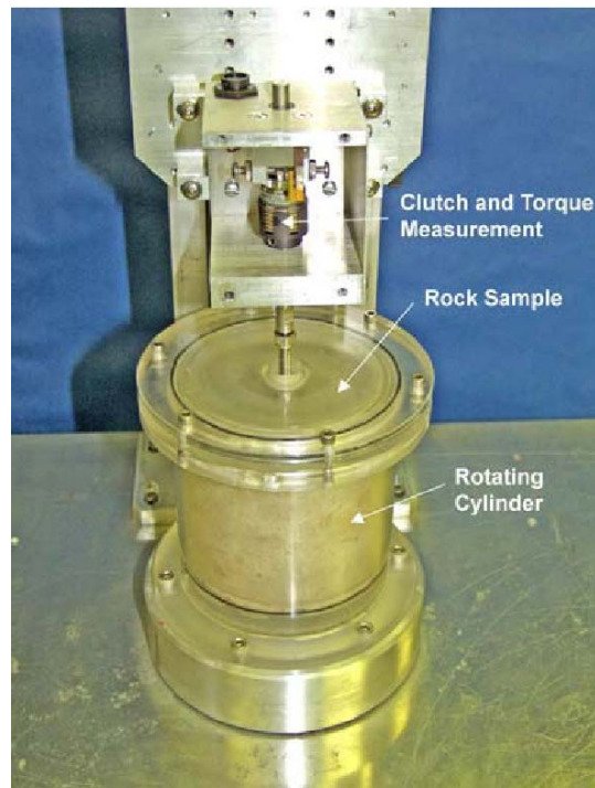
Figure A-4. Rotating Erosion Test Apparatus (RETA)
