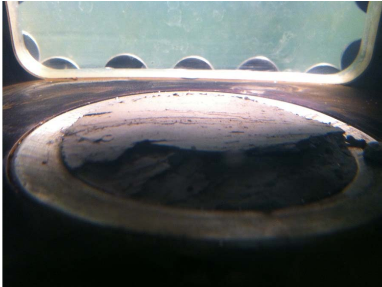
Figure B-5. Yazoo Clay 18.5_1 Test Failure Wedge
