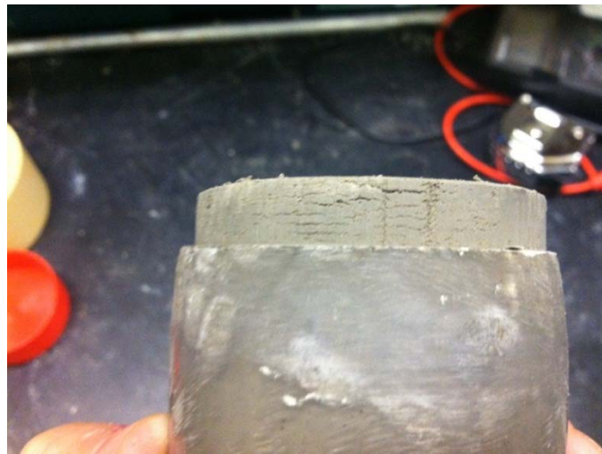
Figure B-17. Prairie Bluff Chalk Formation Cracking Example 2
