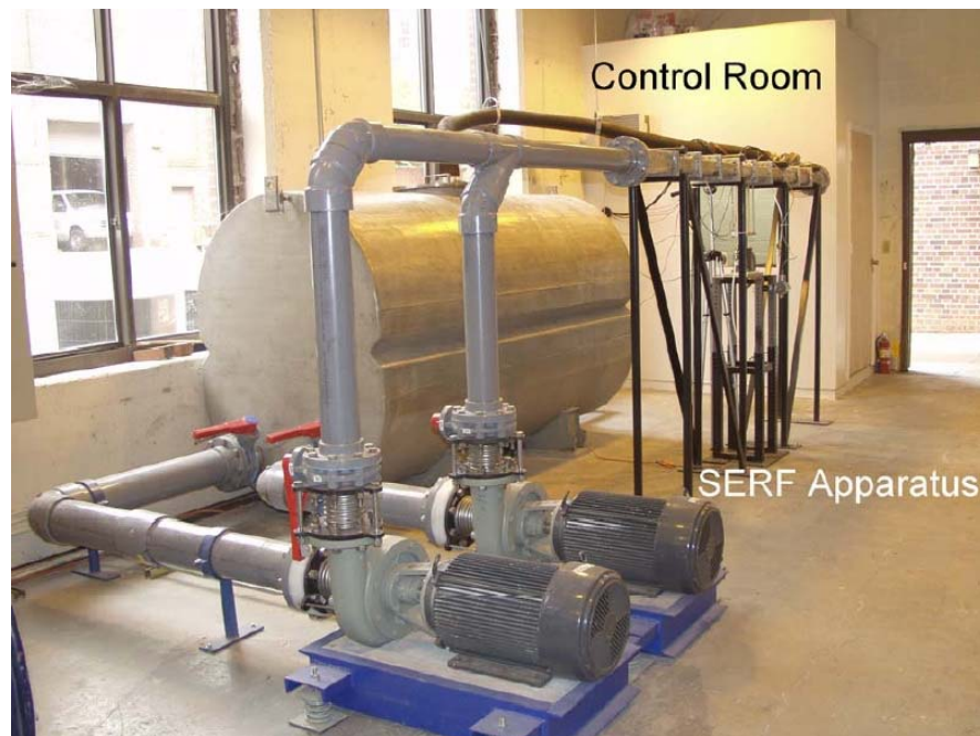
Figure A-5. Sediment Erosion Rate Flume (SERF)
