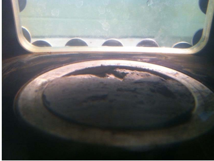
Figure B-8. Yazoo Clay 18.5_9 Test Scoured Area from Front
