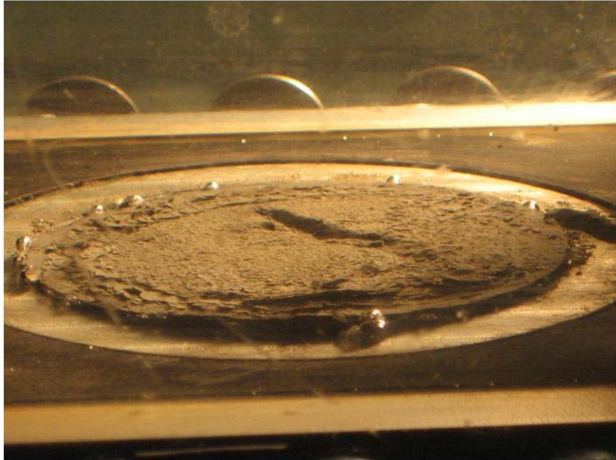
Figure C-21. Bucatunna 26.0_3 Sample Approximately 3 Minutes into 3.0 m/s EFA Test
