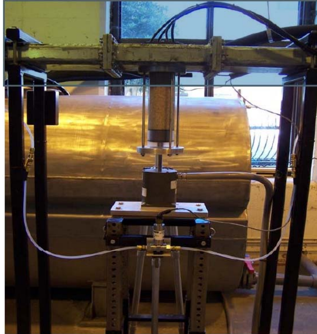
Figure A-6. SERF Sample Chamber and Stepping Motor
