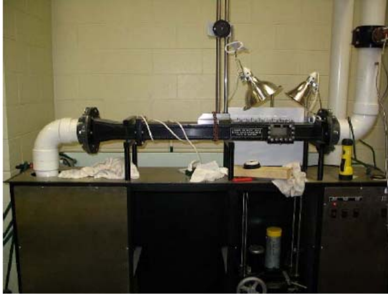
Figure A-1. Erosion Function Apparatus
