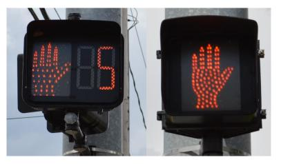
Figure 2.2 Pedestrian countdown signal (left) vs. standard pedestrian signal (right)
