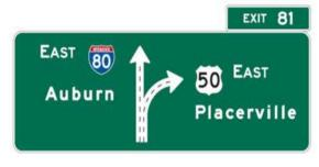
Figure 2.5 Diagrammatic Guidance Sign
