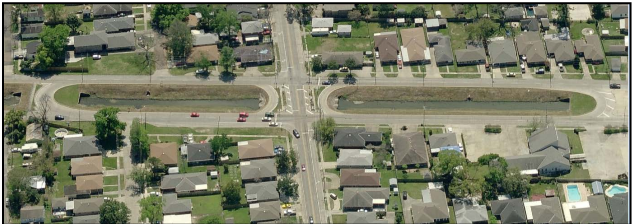
Exhibit 1-16. MUT intersection with water retention ponds in median in New Orleans, Louisiana. (2)
