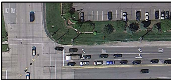
Right-turn and shared through/right on minor street
