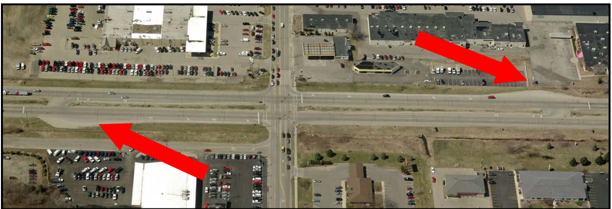
Exhibit 1-5. Use of loons to reduce median width. (2)
