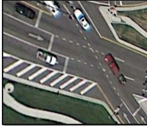
Exhibit 4-9. Pavement marking used to channel vehicles through crossovers. (26)
