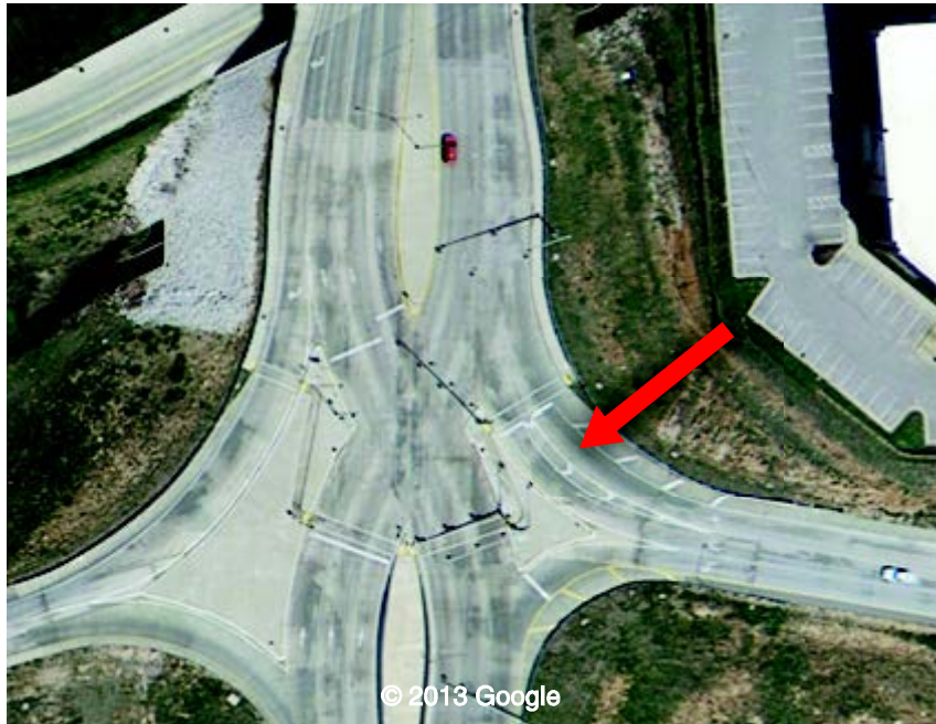
Exhibit 5-12. Lane separation for heavy and emergency vehicle accommodation. (26)
