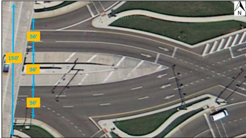
Exhibit 7-11. Cross-sectional distances for a symmetrical alignment with no reverse curves between crossovers (Dorsett Rd., Maryland Heights, MO). (26)
