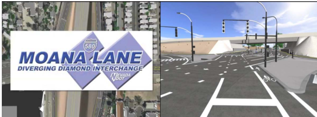
Exhibit 2-3. Example video screen capture from Nevada DOT of how to travel through a DDI. (20)
