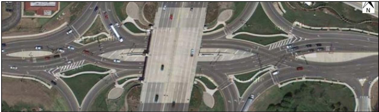
Exhibit 7-10. Symmetrical alignment with no reverse curves between crossovers (Dorsett Rd., Maryland Heights, MO). (26)
