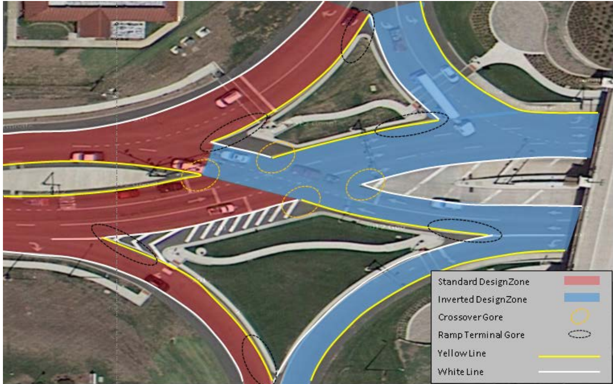
Exhibit 8-22. Example centerline and edge line pavement markings at a DDI. (26)
