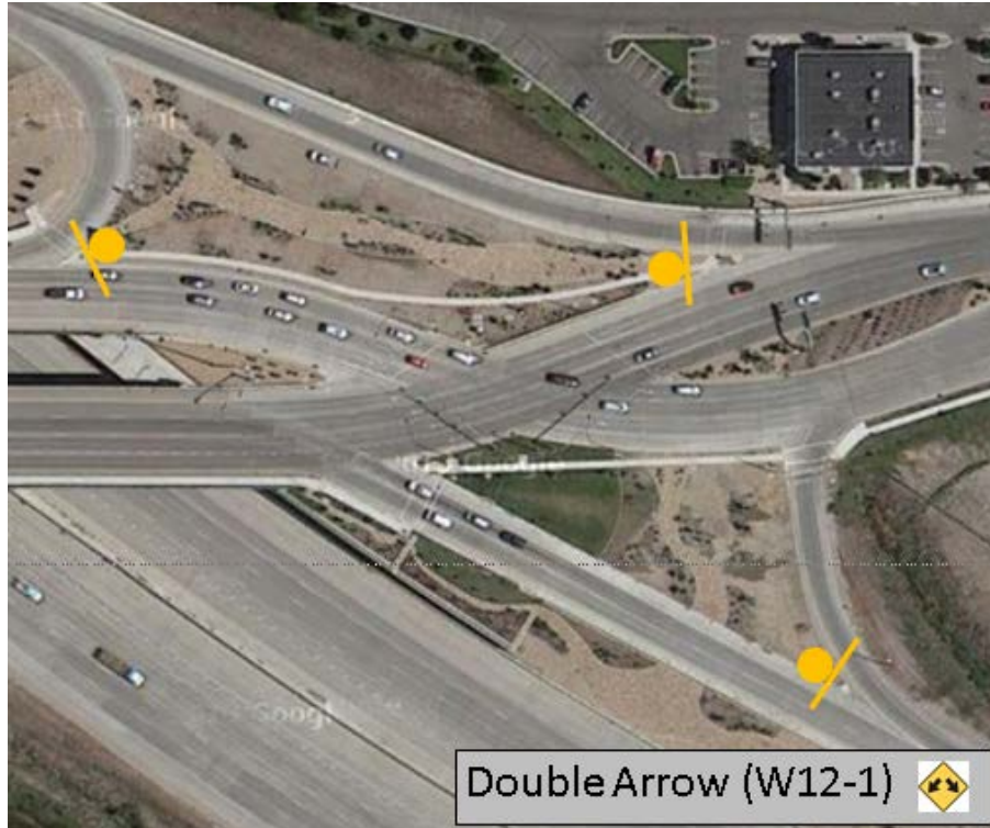
Exhibit 8-20. Double Arrow signs. (26)
