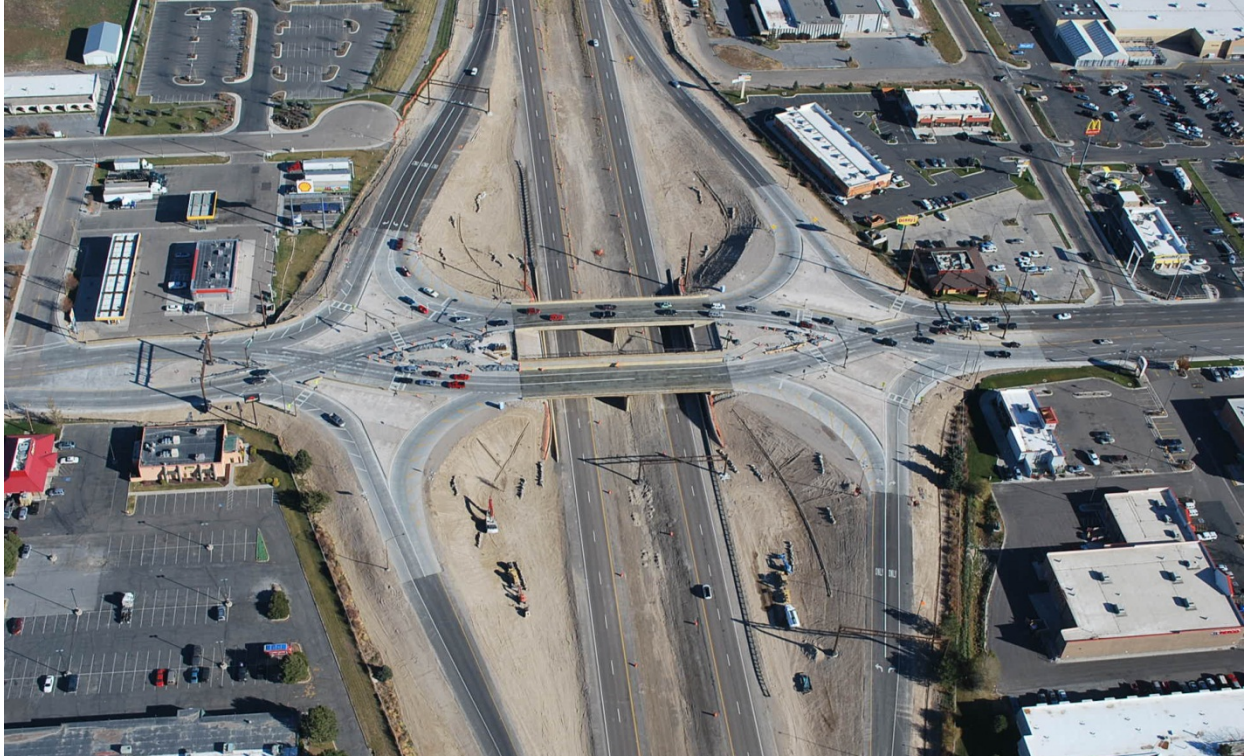
Exhibit 1-6. First constructed DDI in Idaho at Interstate 86 and US 91/Yellowstone Highway (Pocatello-Chubbuck, ID). (4)
