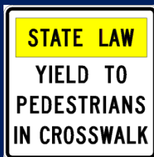
Post-mounted Regulatory Pedestrian Sign (Source: MassHighway Traffic Engineering)
