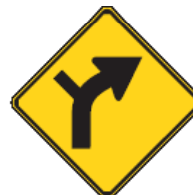
Typical Warning Sign (W1-10) (Source: MUTCD)
