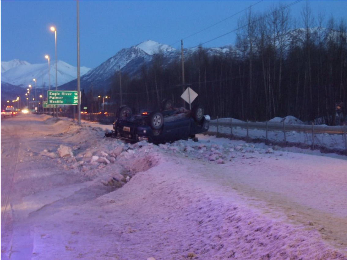
Figure 2. A vehicle rollover due to a snow berm
