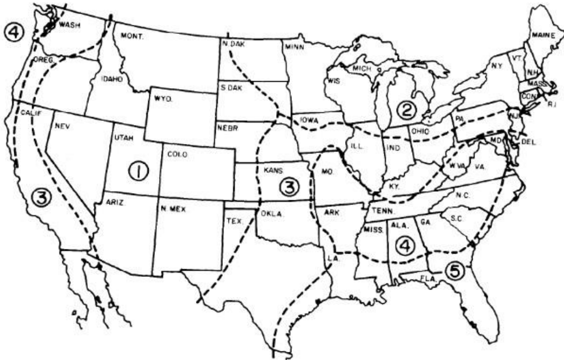
Figure 1.2 Decay severity zones for wood poles
