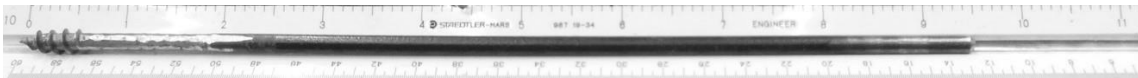
Figure D.1 Drill bit used for checking decay. The total modified bit length was 9.5 inches. The bit was created from a FastenMaster® HeadLok® HLG M010 heavy duty flathead fastener. The head was removed and the threads were machined down to four full turns, starting at the tip.
