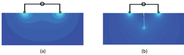
Figure 4.5 Heatmap from Finite Element Simulations showing regions of equipotential conducted on (a) plain slab specimen and (b) notched slab specimen, taken from Niemuth (2004).
