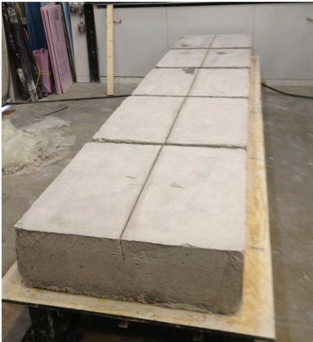
Figure 3.5 Slabs, with molds removed, after curing, and during the drying stage.
