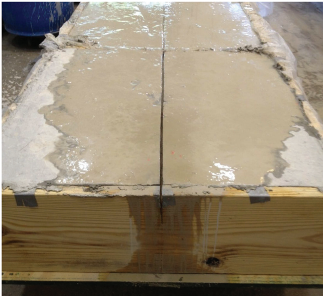
Figure 3.4 Slabs after the saw-cut joints had been made.
