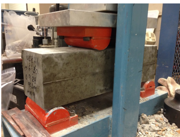
Flexural strength testing
