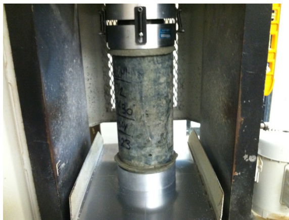
Compressive strength testing
