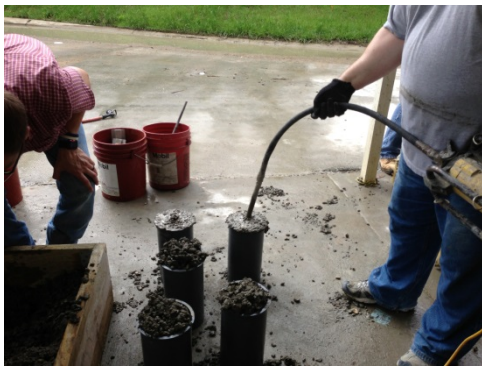
Casting 6" x 12" cylinders
