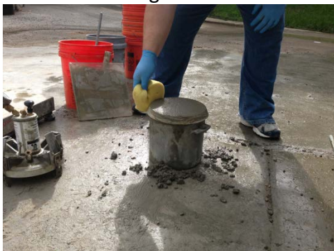
Pressure for air content measurement
