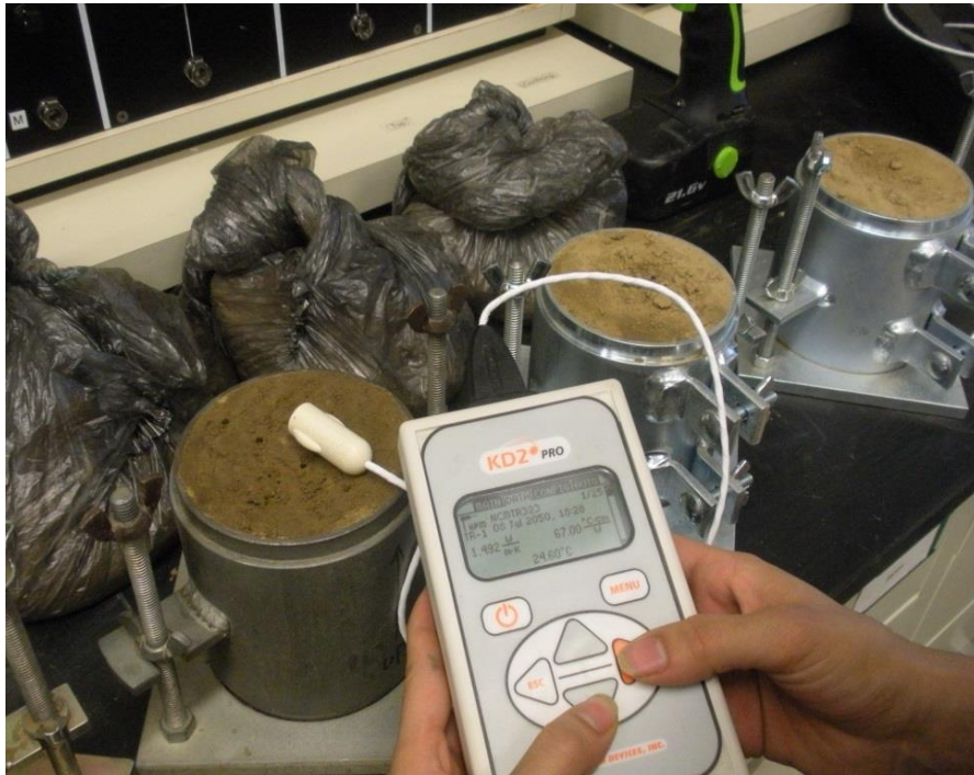
Figure 3-5 Thermal conductivity measurement using KD2 pro
