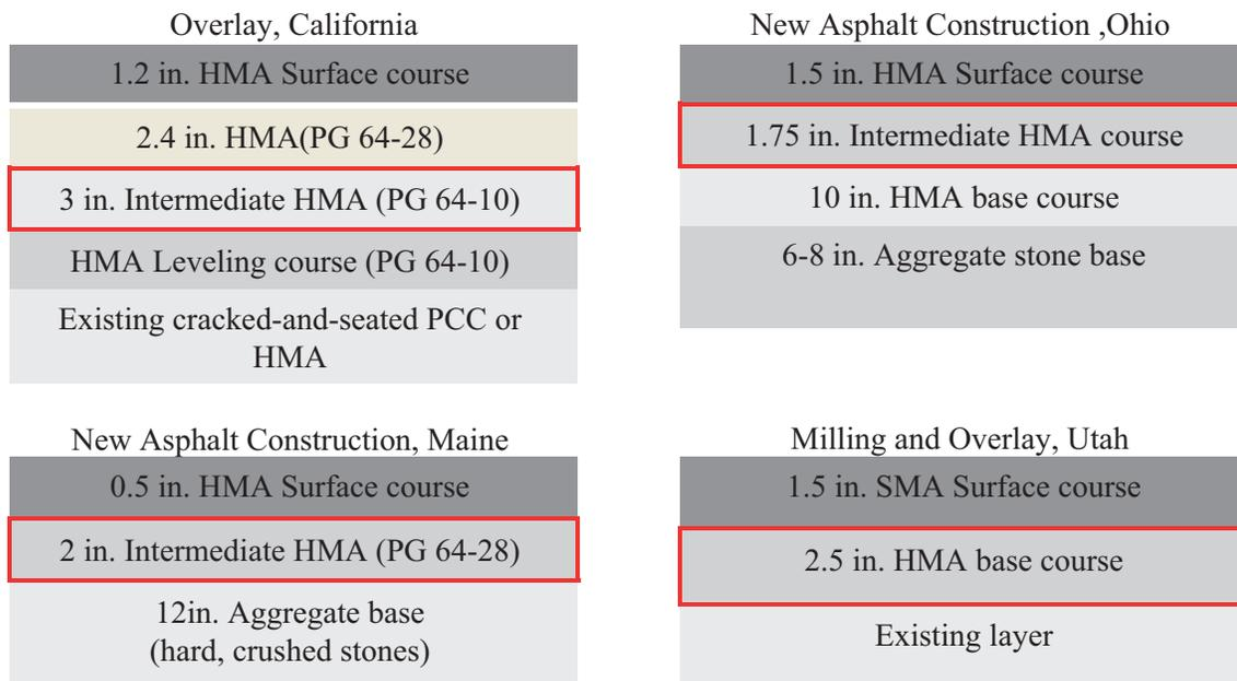
**Figure 2.12** IC demonstration layers in the four selected projects in CA, OH, ME, and UT. (Note: The target layers are illustrated with a box around it.)
