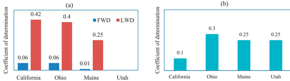
**Figure 2.15** Correlations of final coverage data for the four IC demonstration projects: (a) FWD/LWD and compaction response values; (b) core density and compaction response values.
