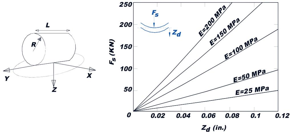
Figure 2.10 Relationship between contact force and drum displacement per cylinder on elastic half-space theory (Mooney & Adam, 2007).
