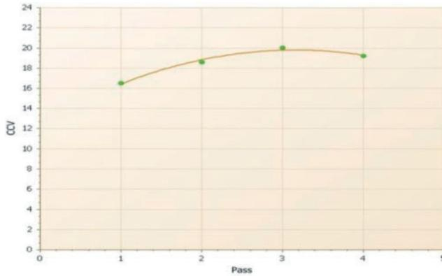
**Figure 2.11** Compaction curve (by Veda).
