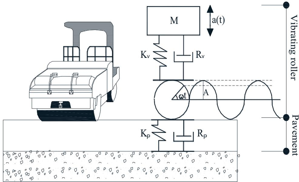
**Figure 2.6** Mechanical and analytical model for the pavement. (where,  $a(t)$ : acceleration,  $M$ : roller mass,  $K_v$ : spring stiffness of vibrating roller,  $R_v$ : damping of vibrating roller,  $A$ : amplitude,  $\omega$ : circular frequency,  $t$ : time,  $K_p$ : spring stiffness of pavement,  $R_p$ : damping of pavement).
