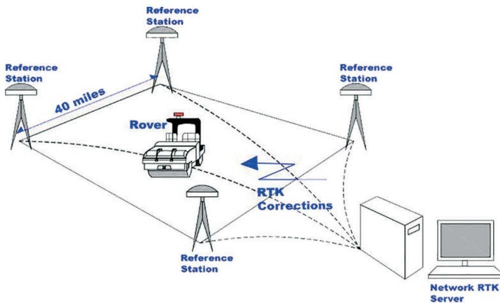
Figure 2.4 Virtual Reference Stations (VRS) GPS system.
