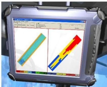
Figure 2.2 Integrated on-board documentation system (HAMM).
