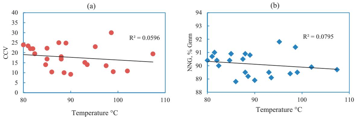
Figure 5.4 Comparison of coefficient of determination: (a) relationship between CCV and temperature (all passes); (b) relationship between NNG and temperature (all passes).
