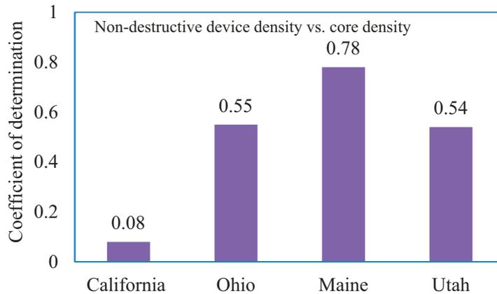
Figure 2.13 Coefficient of determination for the four IC demonstration projects.
