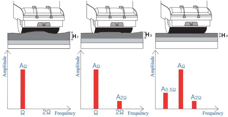
**Figure 2.8** Harmonic wave spectrum (Chang et al., 2011b).
