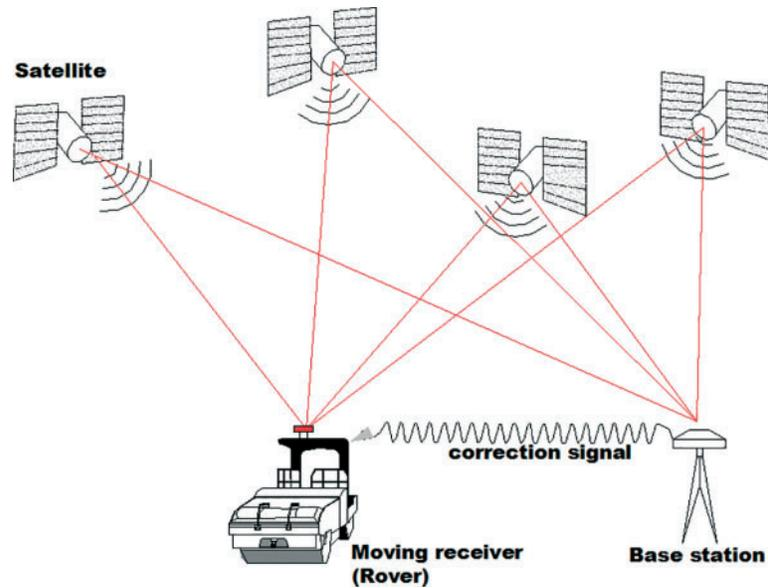
Figure 2.3 Real-Time Kinematic (RTK) GPS system.
