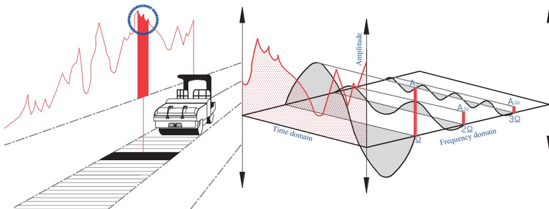
**Figure 2.7** Compactor principle for compaction meter (Texas Instruments, 1980; Thurner & Sandström, 2000).
