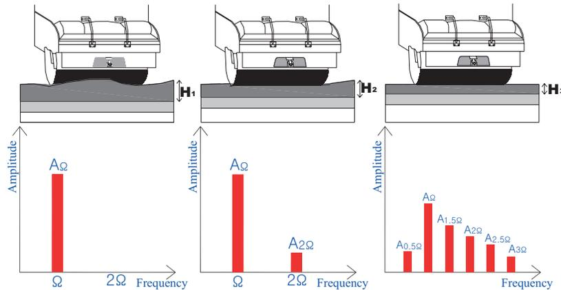
**Figure 2.9** Changes in amplitude spectrum with increasing ground stiffness (Chang et al., 2011b).
