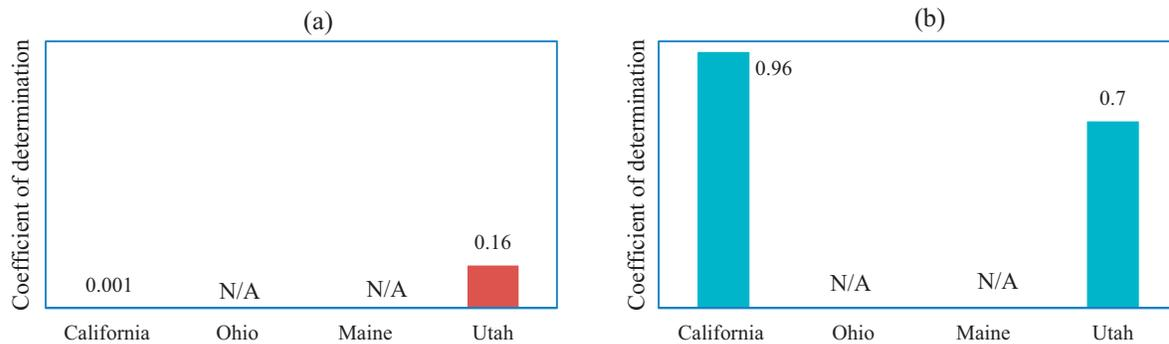
**Figure 2.16** Correlations between NG density and ICMV data for the four demonstration projects: (a) final coverage; (b) all-passes data.
