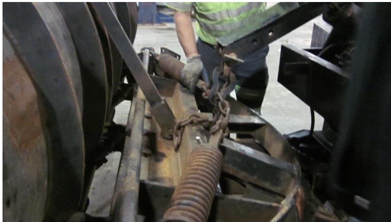
Figure 7.12: Adjusting the Spring Counterbalance after New Blade is Installed.
