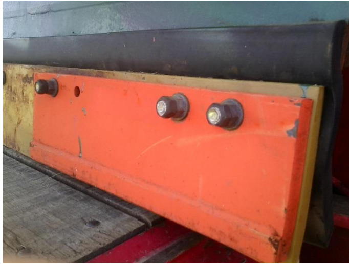
Figure 7.11: Head of Bolts Facing the Back Side of the Trip Edge.
