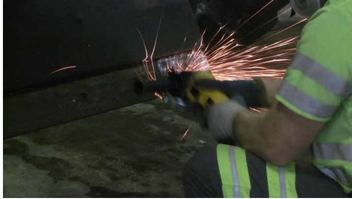
Figure 7.9: Removing Loose Debris from the Trip Edge Prior to Installing New Blade.
