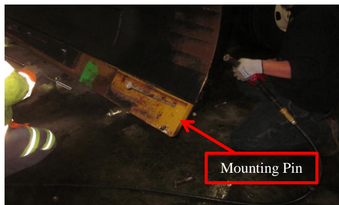
Figure 7.8: Removing the Worn Blade from a Plow.
