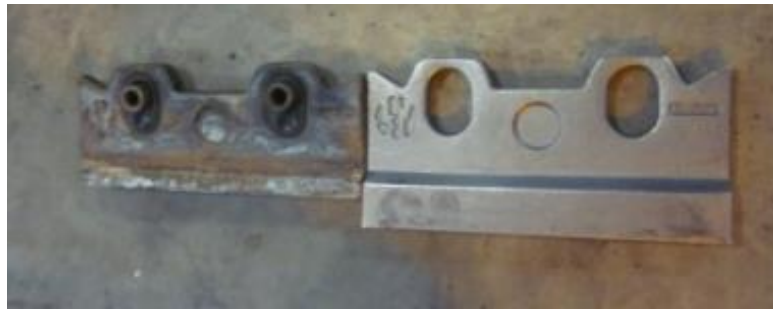
Figure 5.4: Original Carbide Tooth (on the left) compared to Replacement Carbide Tooth (on the right) for the PolarFlex Blade.
