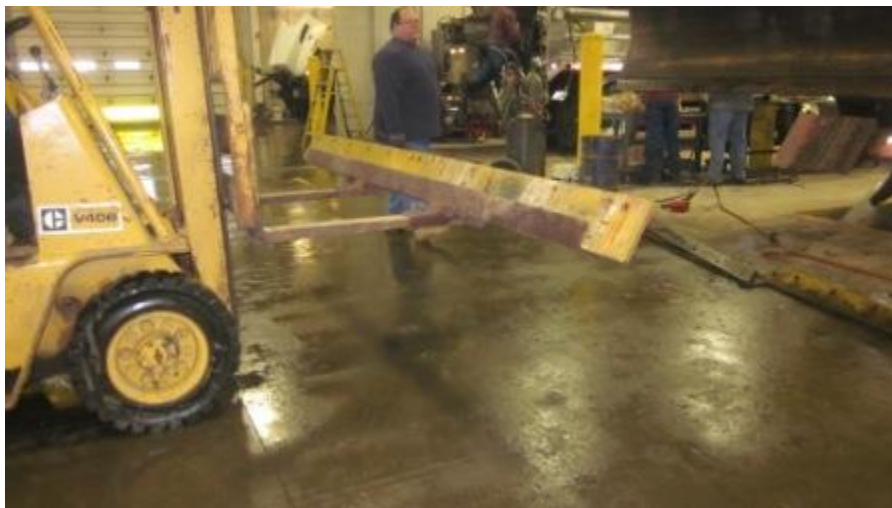
Figure 7.3: Homemade Blade Lift in Fairfield County.
