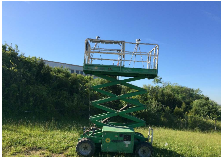
Figure 30: Two Cameras Mounted on the Scissor Lift
