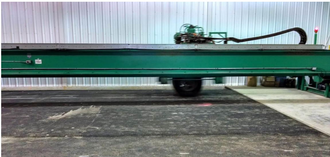
Figure 56. Load wheel passing over test pavement in the APLF.
