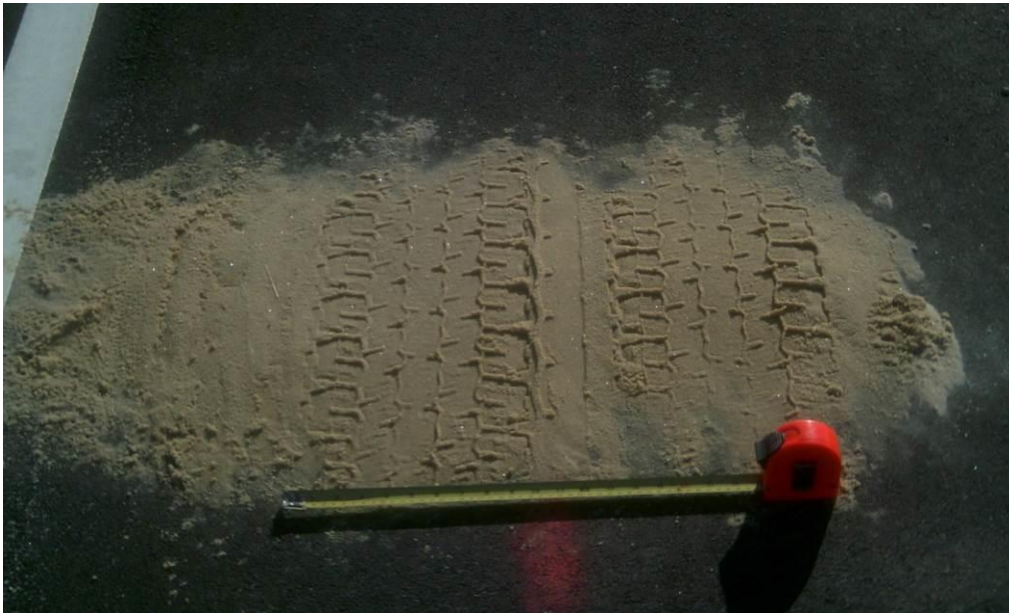
Figure 8. Measurement of lateral offset from tire track after loaded truck has passed over the sensors.
