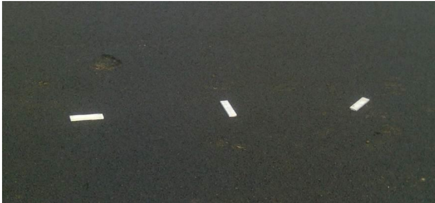
Figure 3. Surface layer strain gage orientations.
