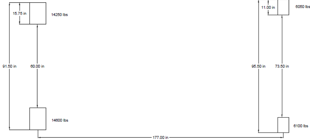
Figure E.2 Single axle wide-based tire (max load) (1 in = 2.54 cm, 1lb = 4.45 N, 100 psi = 689 kPa)
