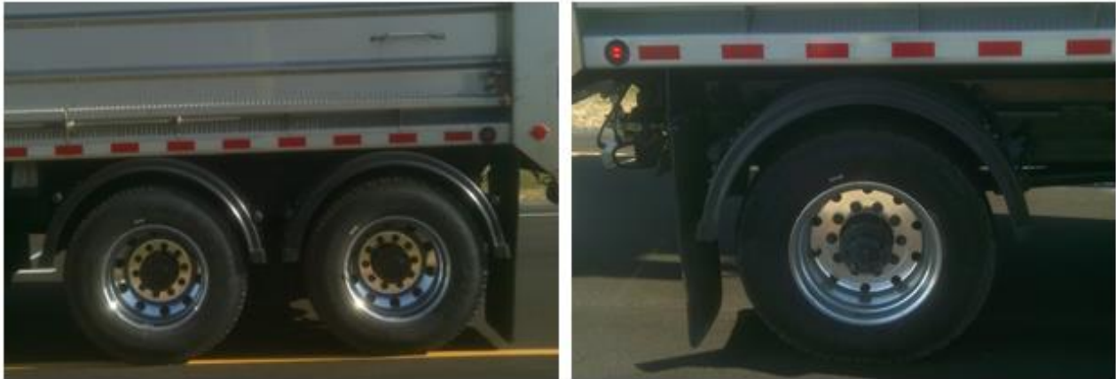
Figure 10. Axle configurations used in CVL tests: Left, tandem axle; right, single axle with wide base tire.
