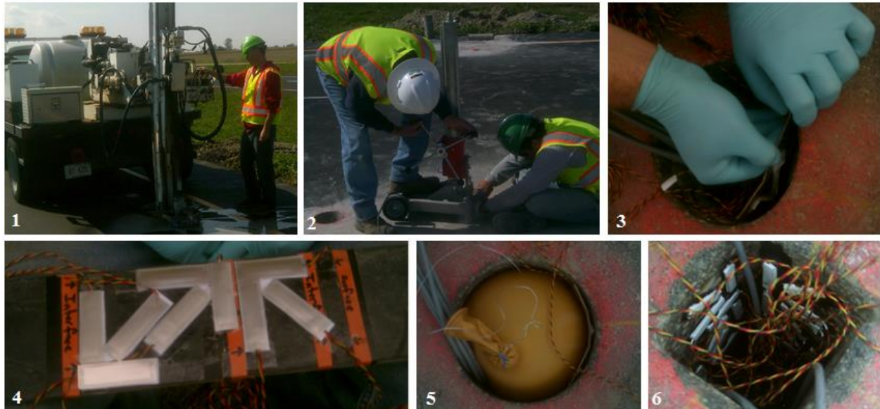
Figure 6. Strain gage rosette installation: 1. Drilling hole; 2. Grinding square hole; 3. Attaching gage to round hole; 4. Gages arrayed for installation; 5. Balloon used to hold gages in place while adhesive dried; 6. Gages in square hole with lead wires attached.
