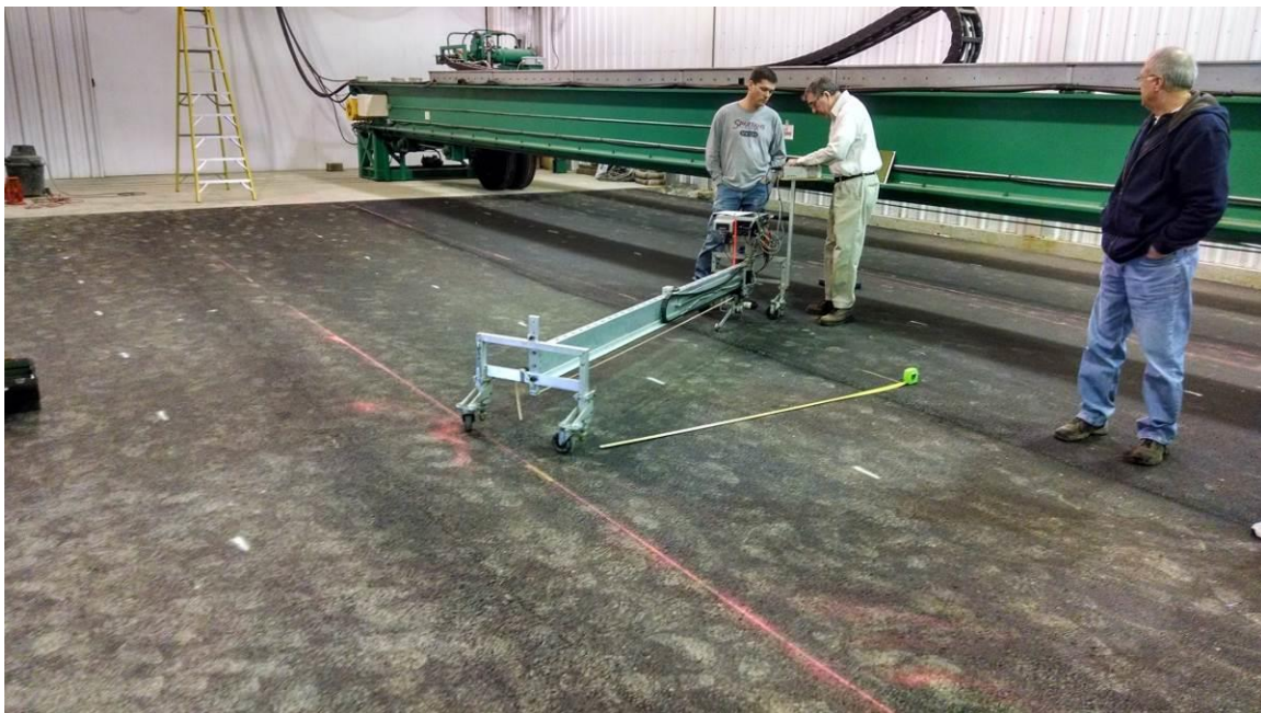
Figure 58. Rolling wheel profilometer in use at the APLF.
