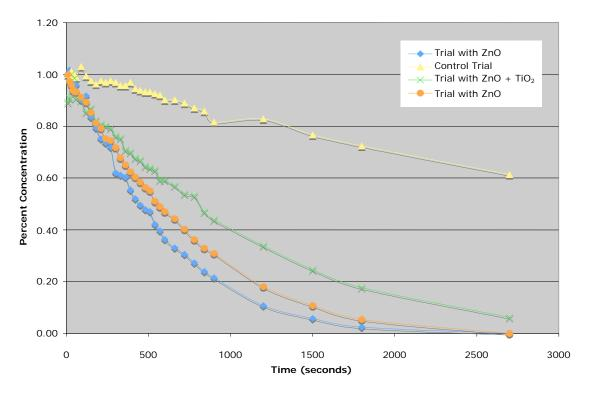
Figure 27. Nitrogen Dioxide30 ppm NO<sub>2</sub> Gas Concentration Reduction with Titanium Dioxide (Indoor)
