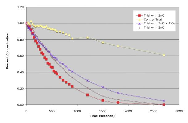
Figure 28. Nitrogen Dioxide Reduction without Titanium Dioxide 60 ppm NO<sub>2</sub> Gas Concentration (Indoor)
