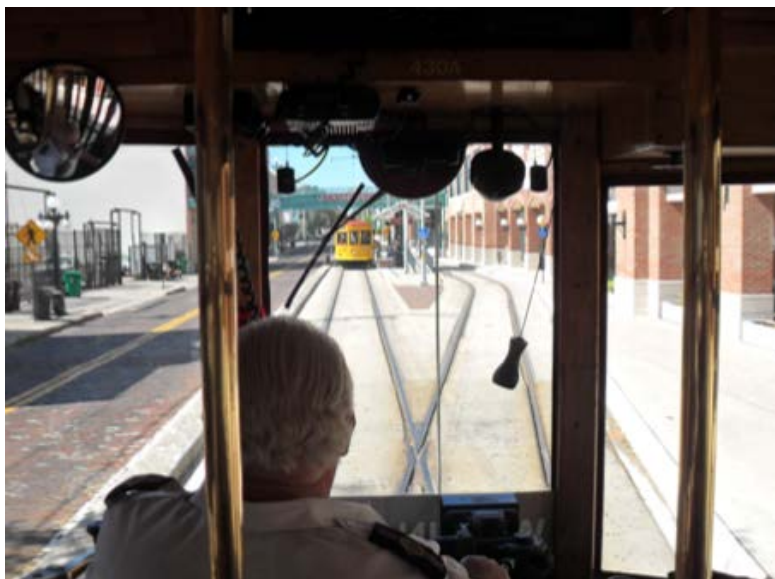
Figure B-7 TECO streetcar approaching meet with opposite- direction streetcar in single-track non- signaled street-running territory
