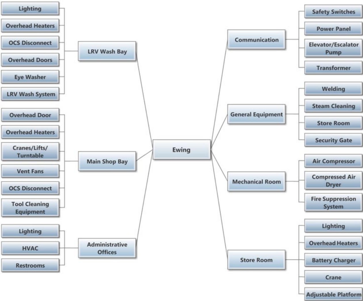
Figure 4-7 Typical Rail Maintenance Facility Hierarchical Components
