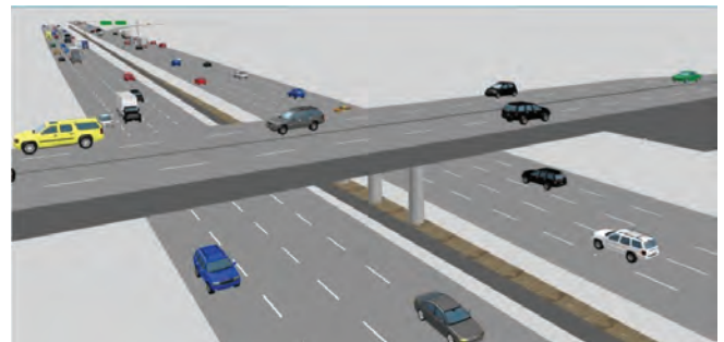
Figure 3-10. 3D engineered models can be imported into traffic simulation software to perform traffic flow analyses.
