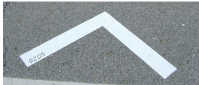
Figure 2-12. This photo shows a control point target that was used on the I-35 & IA92 interchange project.
