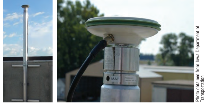
Figure 2-6. Permanent base station.
