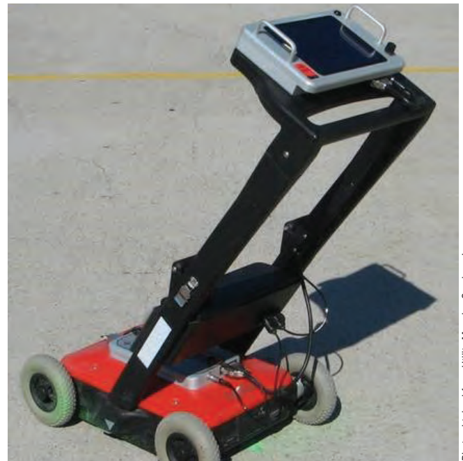
Figure 2-24. Walk-behind ground penetrating radar system.
