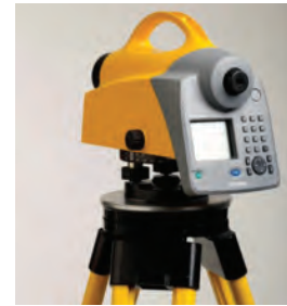
Figure 2-10. Digital level used for transferring elevations across a project site.
