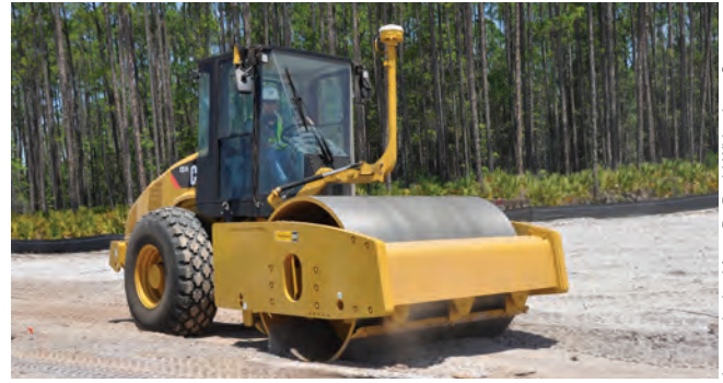
Figure 4-7. Intelligent compaction can utilize GPS for location on a project site.
