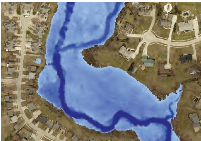
Figure 3-4. Discharge and elevation data from a hydraulic model can be shown on a digital terrain model developed from LiDAR data to accurately demonstrate impacts of different flood events.
