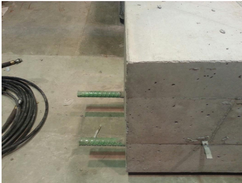
Figure 4. Protruding #14 bars from Side A of the specimen
