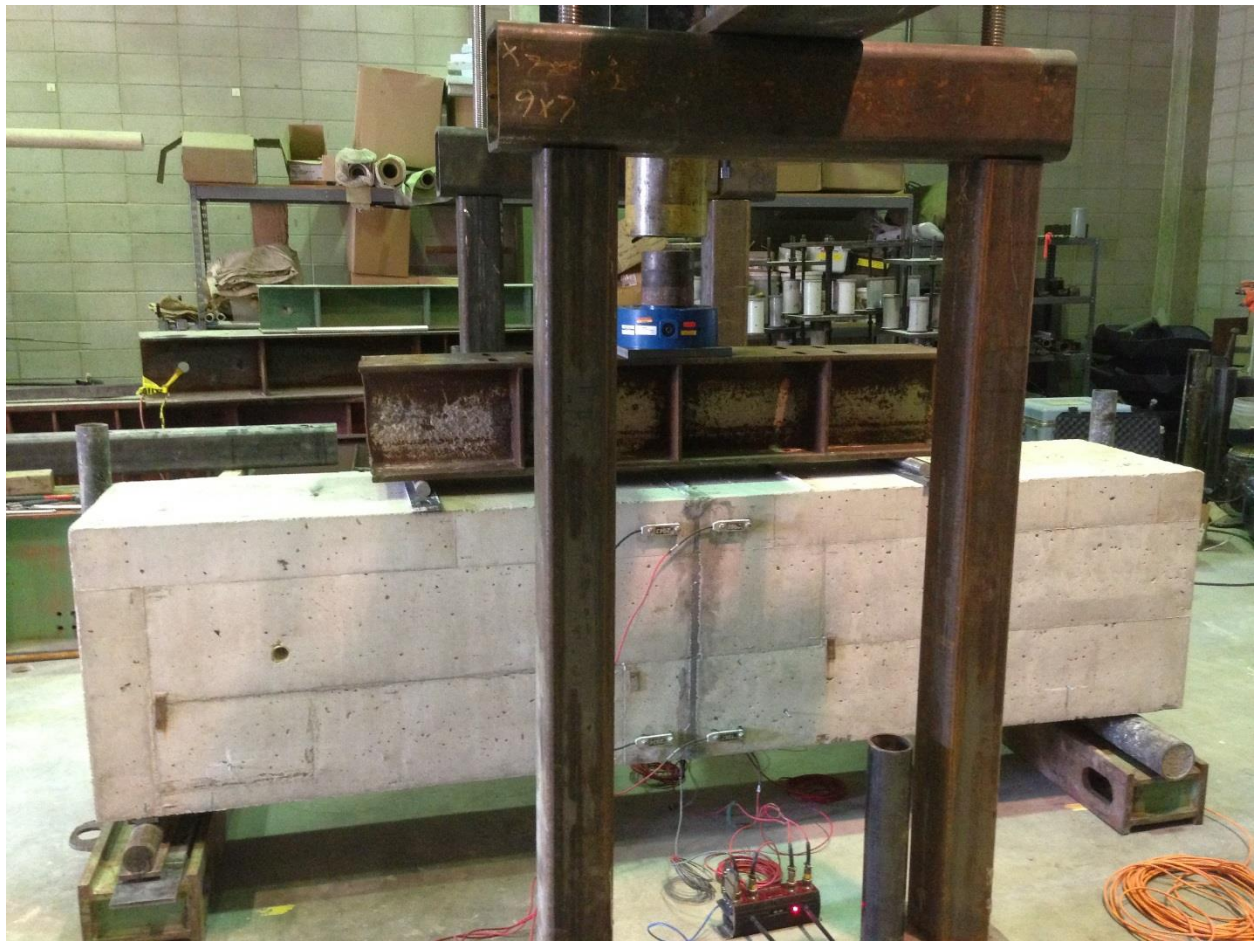
Figure 18. Specimen setup for static four-point bending test
