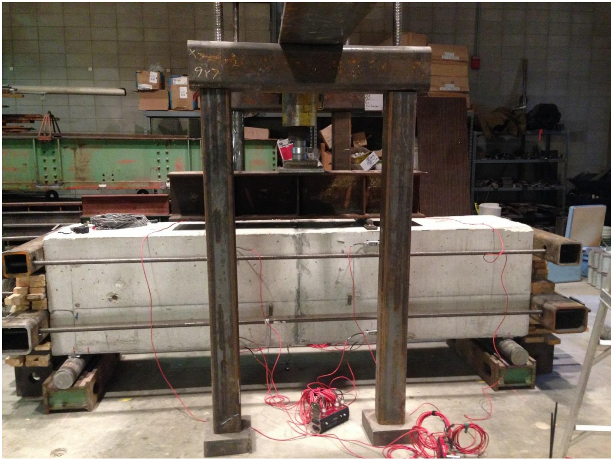
Figure 19. Specimen setup for static four-point bending test with applied axial load
