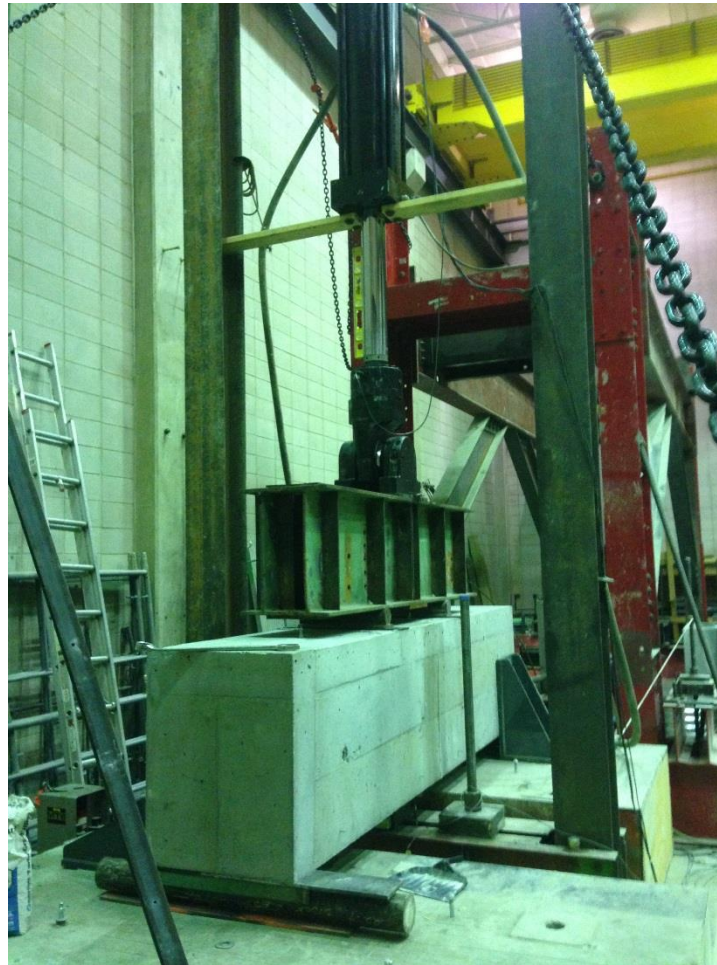
Figure 23. Coupler specimen setup for fatigue testing
