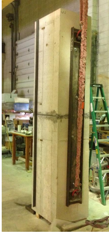
Figure 15. Vertical braced specimen before lowering to horizontal position for testing
