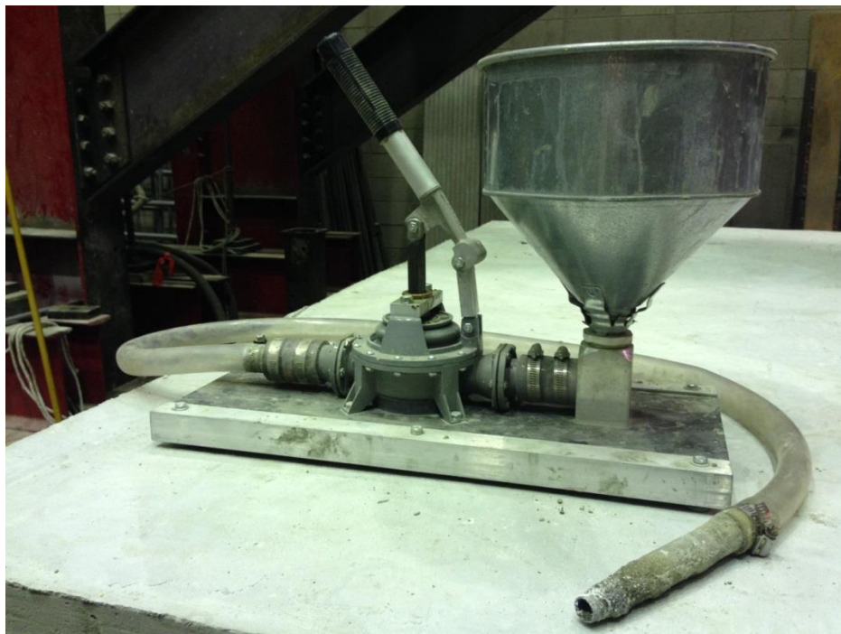
Figure 12. Grout pump used for grouting the reinforcing steel couplers
