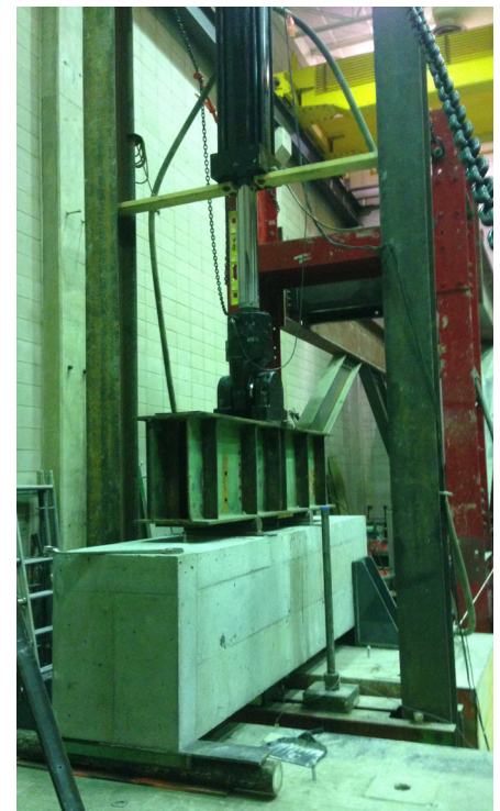
Coupler specimen setup for four-point bending fatigue testing
