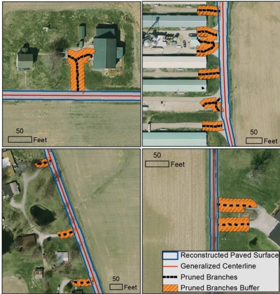
Figure 3.18 Examples of reconstructed paved surface and excluded branches.
