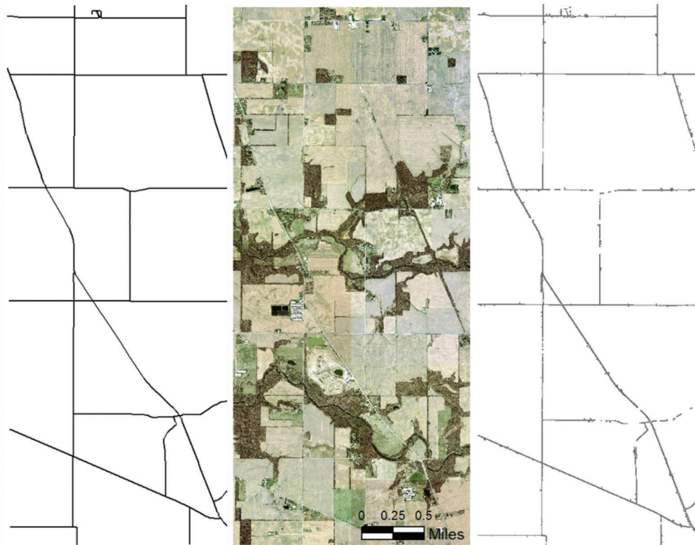
Figure 3.11 INDOT road network (left), orthophoto (middle), road pavement classification result (right) for part of the Indiana Orthophotography Project dataset.
