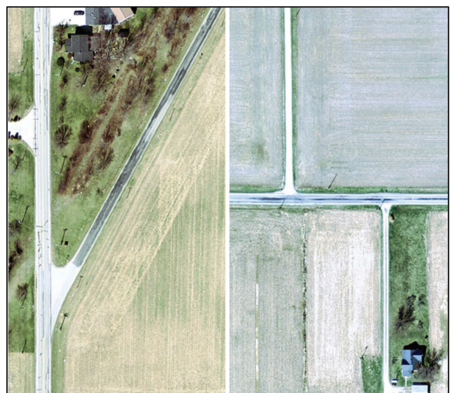
Figure 3.5 Examples of visible spectral differences of road surfaces from the orthophotos.
