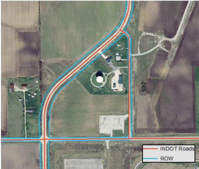
Figure 2.3 Sample from the ROW dataset of Tippecanoe County Highway Department acquired from Tippecanoe County GIS together with INDOT road network.
