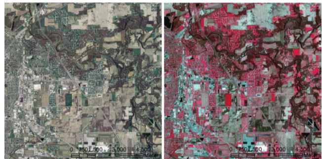
Figure 2.6 Samples of RGB (left), CIR (right) orthophotos from Tippecanoe County acquired in scope of 2005 Statewide Orthophotography Project.
