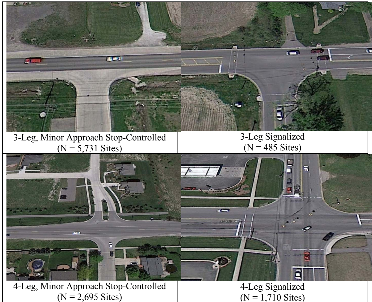
Figure 1. Intersection Site Types
