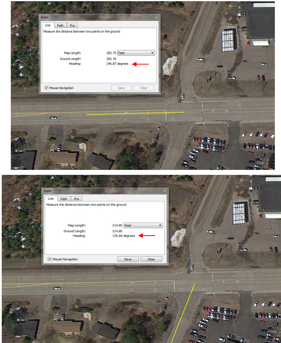
Figure 13. Skew Angle Measurement Example
