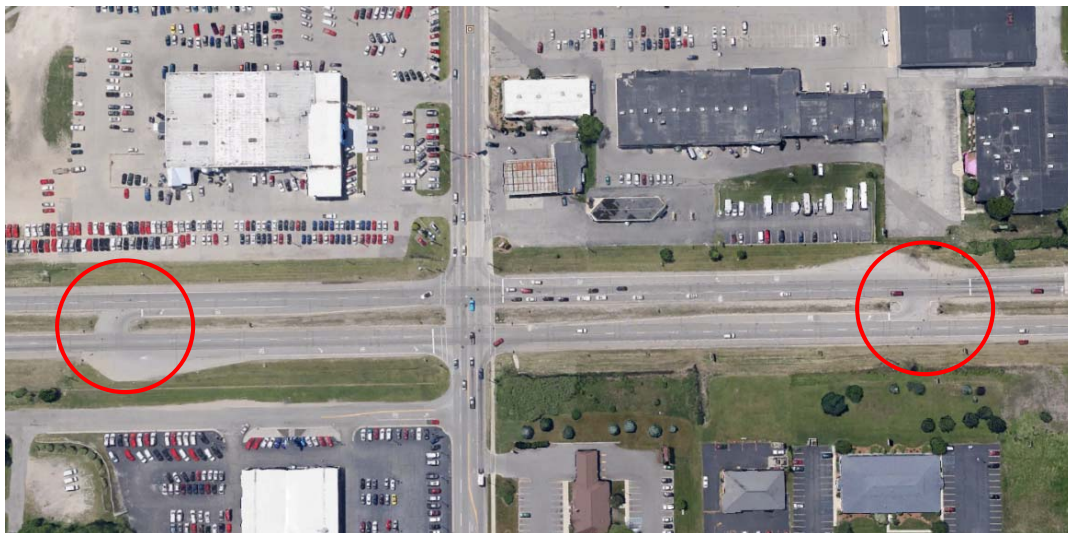
Figure 14. Median Turn-around Field Example
