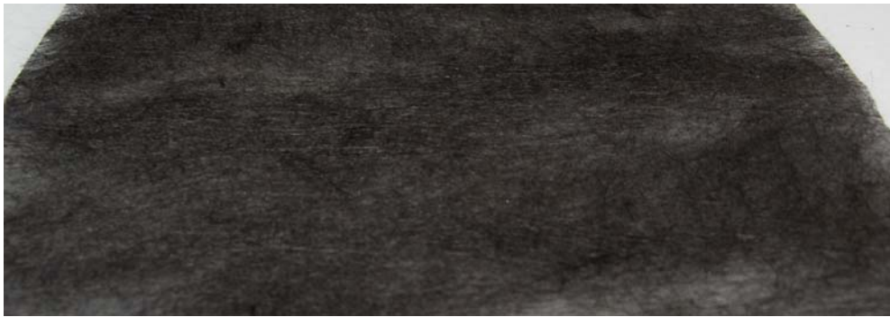
Figure 45 Carbon fiber mat made from a bundle of carbon fiber and epoxy resin binder
