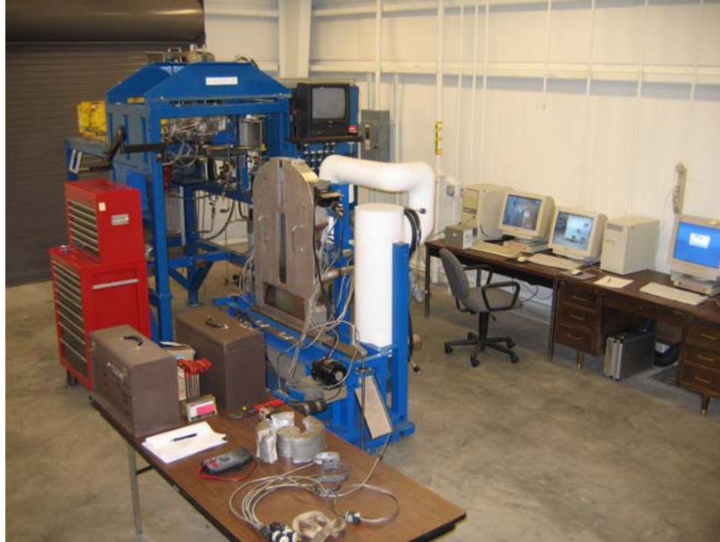
Figure 1 Carbon fiber spinning apparatus mounted on the mobile fiber collection platform with the secondary gas heater, showing most of the components, unassembled
