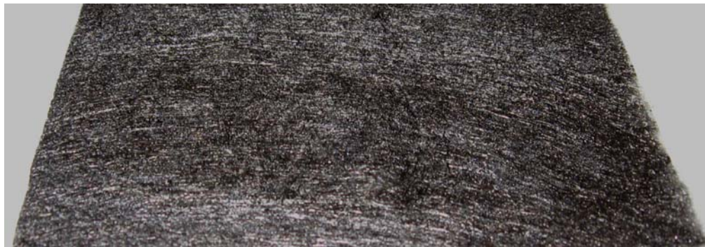
Figure 43 Carbon fiber mat made from strands of carbon fiber and phenolic resin binder
