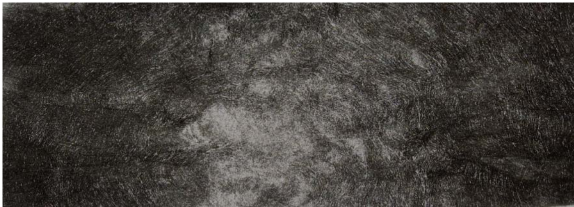
Figure 42 Carbon fiber mat made from a bundle of carbon fiber and PVA binder
