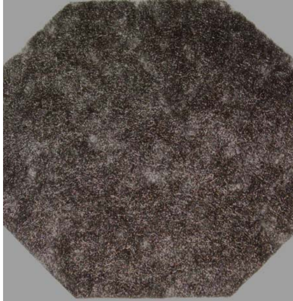
Figure 44 Carbon fiber mat made from chopped carbon fiber (2-10 mm) and phenolic resin binder
