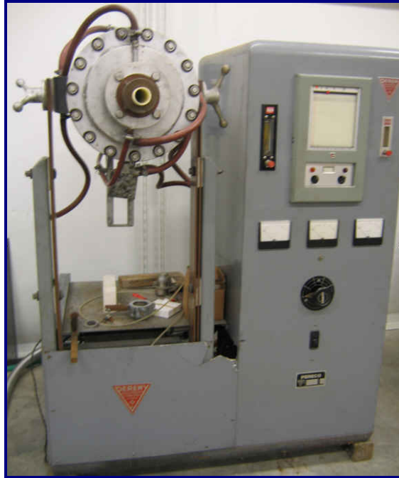
Figure 6 A high temperature furnace for carbonization and graphitization
