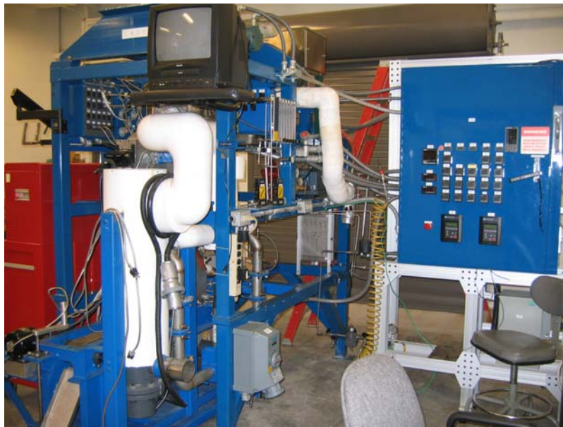
Figure 2 UTSI Spin Lab, a close view of the spin tower, control panel and the fiber collection platform with the secondary gas heater (white duct) in the foreground
