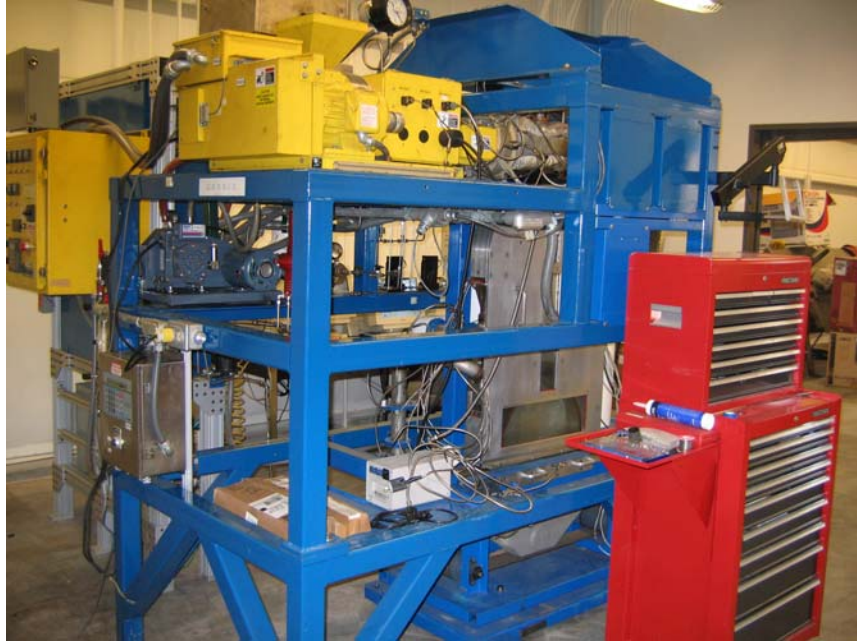
Figure 3 UTISI Spin Lab, side view, showing the extruder system and the control panels for various pumps
