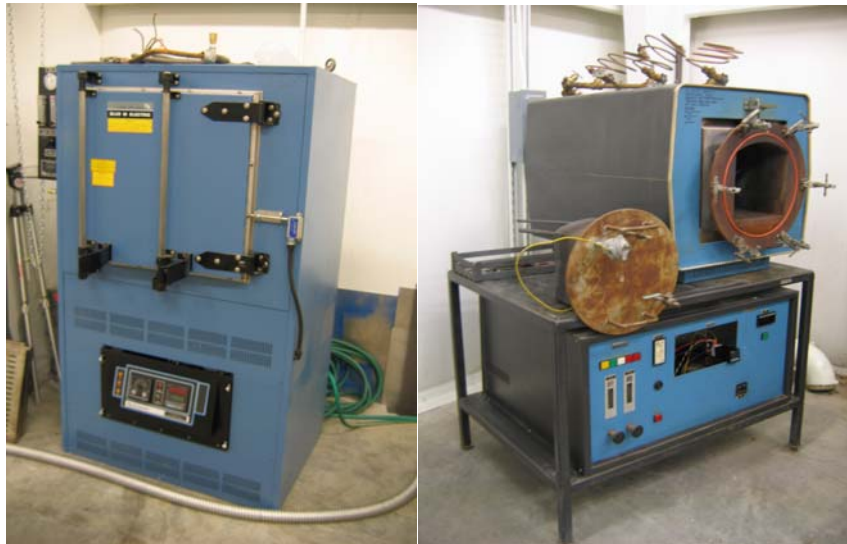
Figure 4 Drying and stabilization (left) and pre-carbonization (right) furnaces
