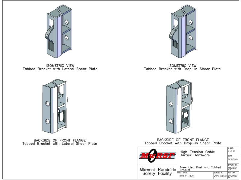
Figure 41. Assembled Post and Tabbed Bracket, Test Nos. HTTB-41 through HTTB-48
