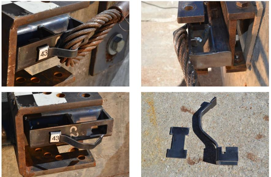
Figure 62. Pre-Test (Upper) and Post-Test (Lower) Photographs, Test No. HTTB-43
