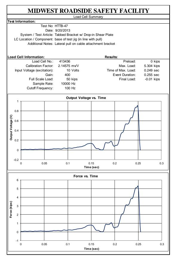
Figure B-7. Load Cell Results, Test No. HTTB-47
