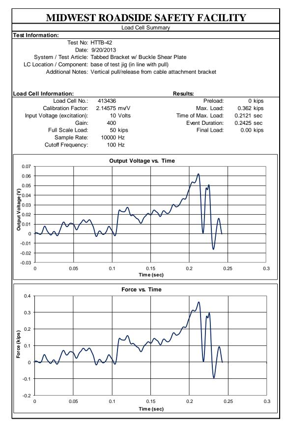
Figure B-2. Load Cell Results, Test No. HTTB-42
