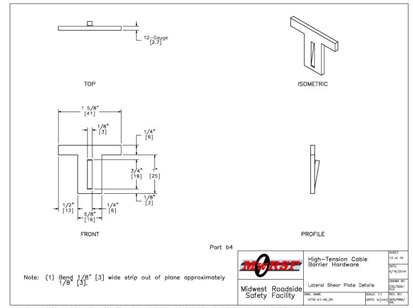
Figure 49. Lateral Shear Plate Details, Test Nos. HTTB-41, HTTB-42, HTTB-45, and HTTB-46
