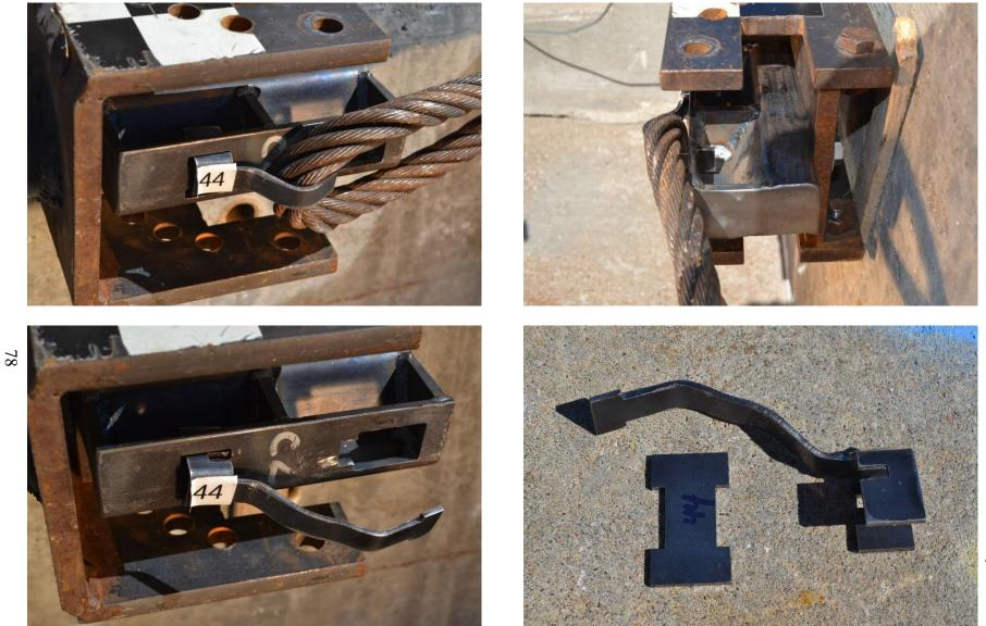
Figure 65. Pre-Test (Upper) and Post-Test (Lower) Photographs, Test No. HTTB-44
