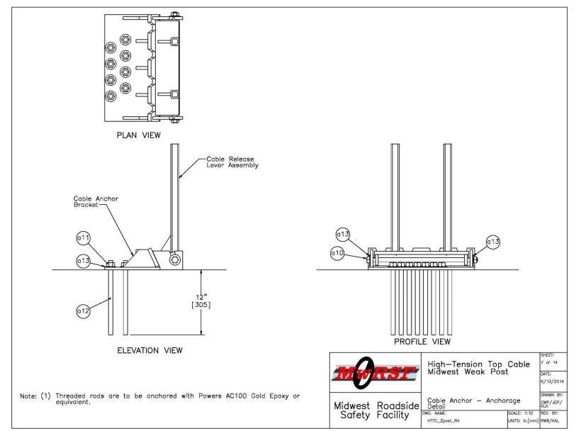
Figure 90. Cable Anchor – Anchorage Detail, Test No. HTTC-2
