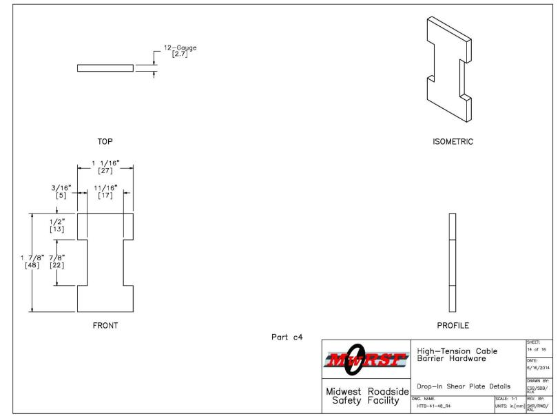
Figure 50. Drop-In Shear Plate Details, Test Nos. HTTB-43, HTTB-44, HTTB-47, and HTTB-48
