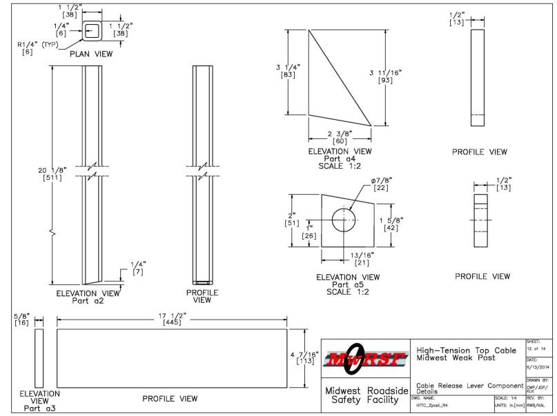
Figure 95. Cable Release Lever Component Details, Test No. HTTC-2
