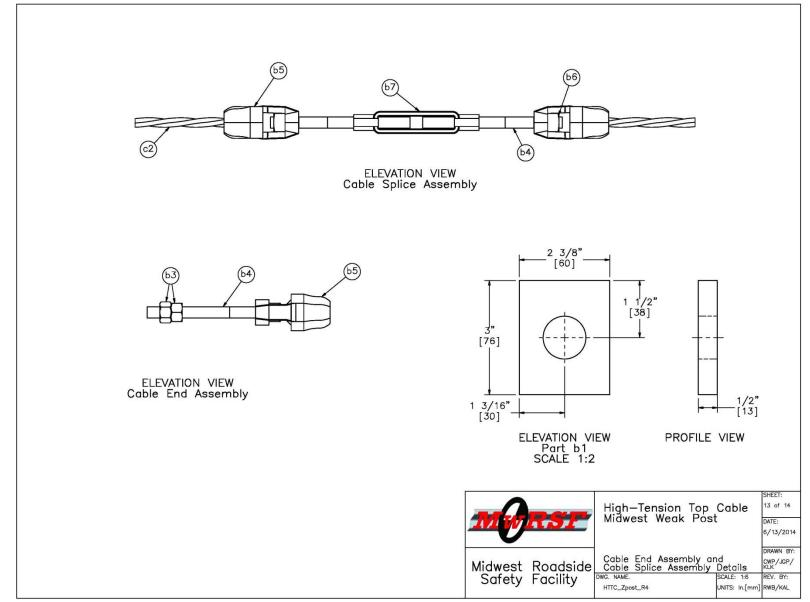
Figure 96. Cable End Assembly and Cable Splice Assembly Details, Test No. HTTC-2
