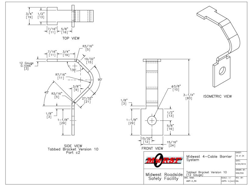
Figure 2. Bolted Tabbed Bracket V-10, Design Details
