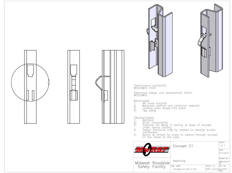
Figure 29. Concept C1, Lateral Shear Plate
