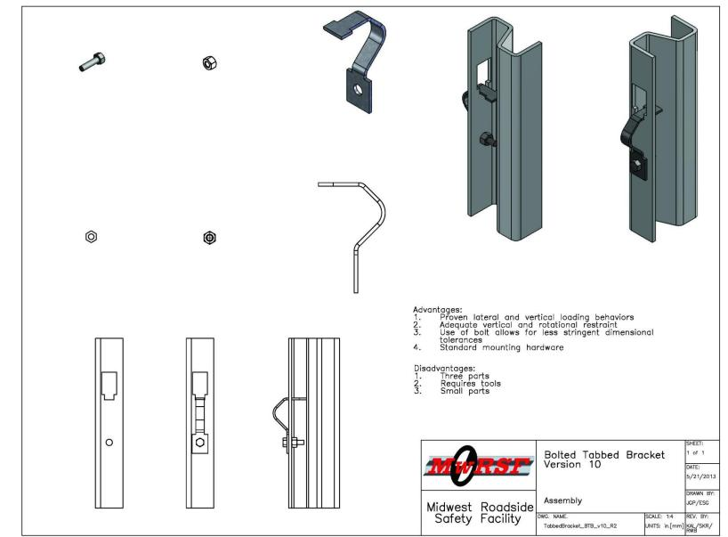
Figure 3. Bolted, Tabbed Bracket V-10
