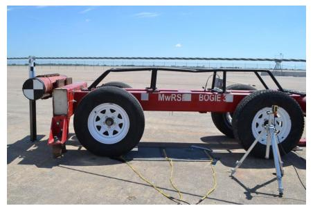
Figure 99. Rigid-Frame Bogie on Guidance Track
