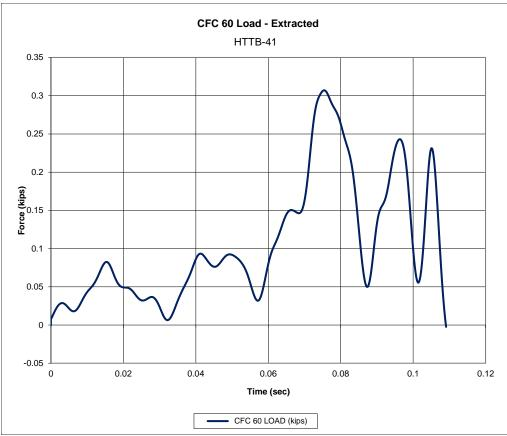
Figure 55. Force vs. Time Data, Test No. HTTB-41
