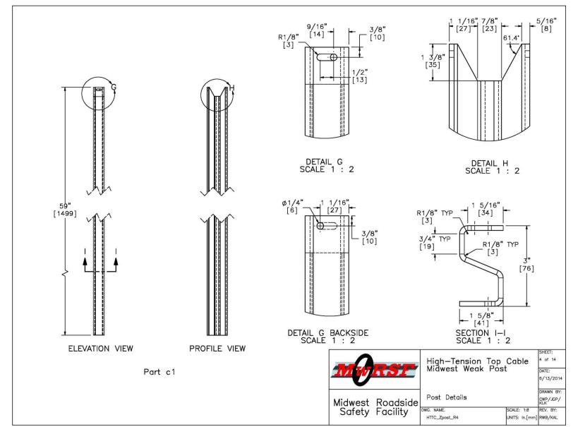
Figure 87. Midwest Weak Post Details, Test No. HTTC-2
