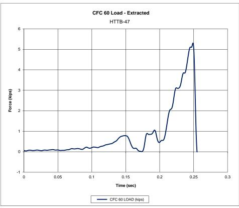
Figure 73. Force vs. Time Data, Test No. HTTB-47
