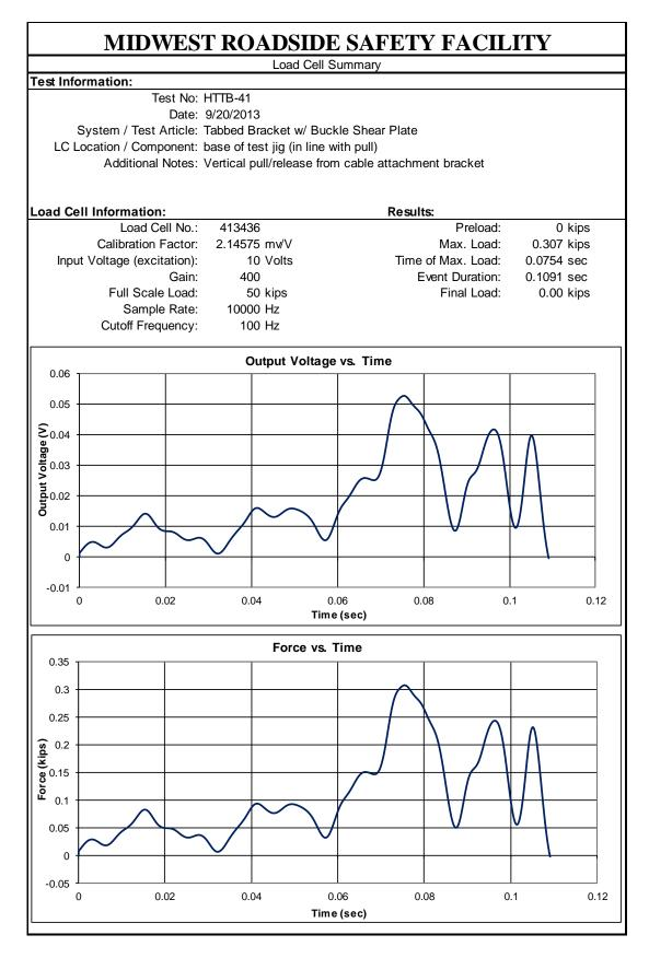
Figure B-1. Load Cell Results, Test No. HTTB-41
