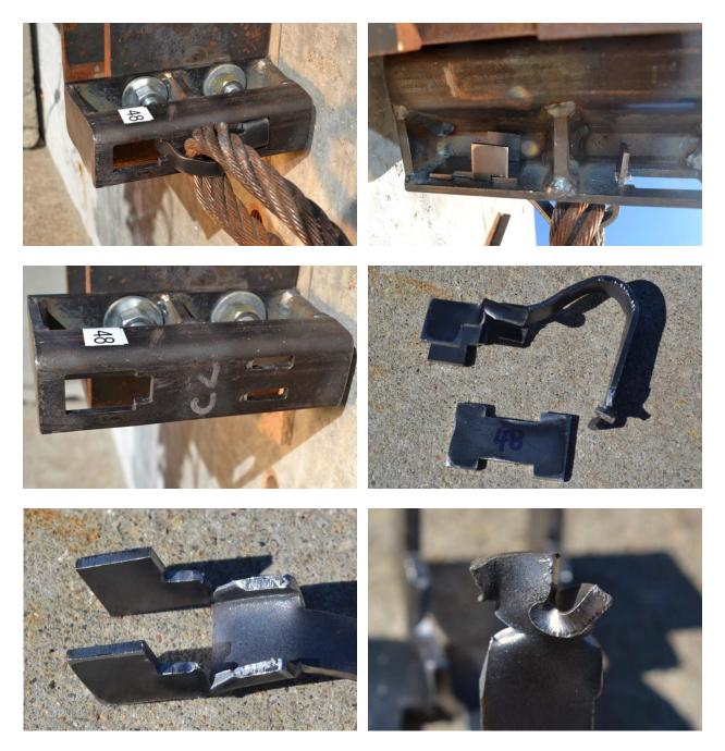
Figure 77. Pre-Test (Top Two) and Post-Test (Bottom Four) Photographs, Test No. HTTB-48
