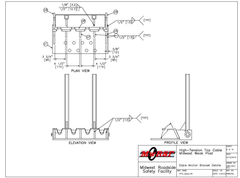
Figure 91. Cable Anchor Bracket Details, Test No. HTTC-2
