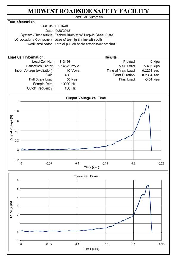
Figure B-8. Load Cell Results, Test No. HTTB-48
