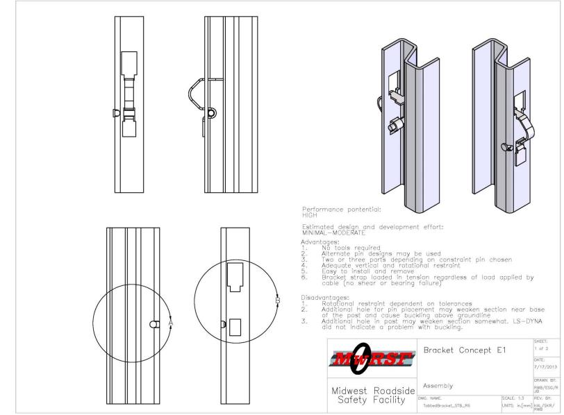
Figure 33. Concept E1, Lateral Pin
