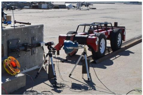
Figure 53. Rigid-Frame Bogie on Guidance Track
