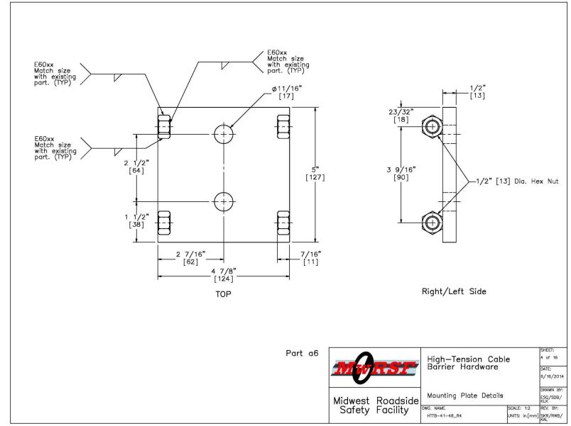
Figure 40. Mounting Plate Details, Test Nos. HTTB-41 through HTTB-48
