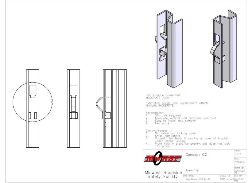
Figure 31. Concept C2, Drop-In Shear Plate
