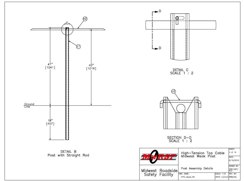
Figure 86. Post Assembly Details, Test No. HTTC-2
