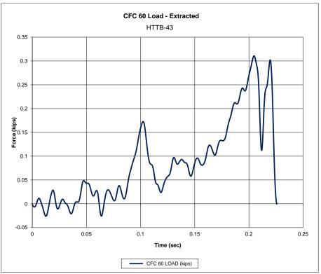
Figure 61. Force vs. Time Data, Test No. HTTB-43
