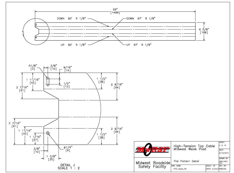
Figure 88. Midwest Weak Post Flat Pattern Detail, Test No. HTTC-2
