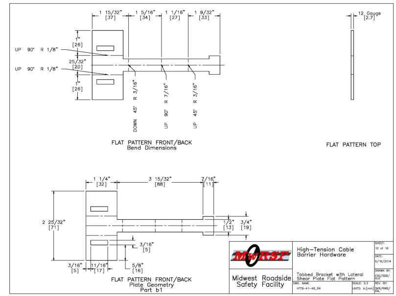
Figure 46. Tabbed Bracket with Lateral Shear Plate Flat Pattern, Test Nos. HTTB-41, HTTB-42, HTTB-45, and HTTB-46
