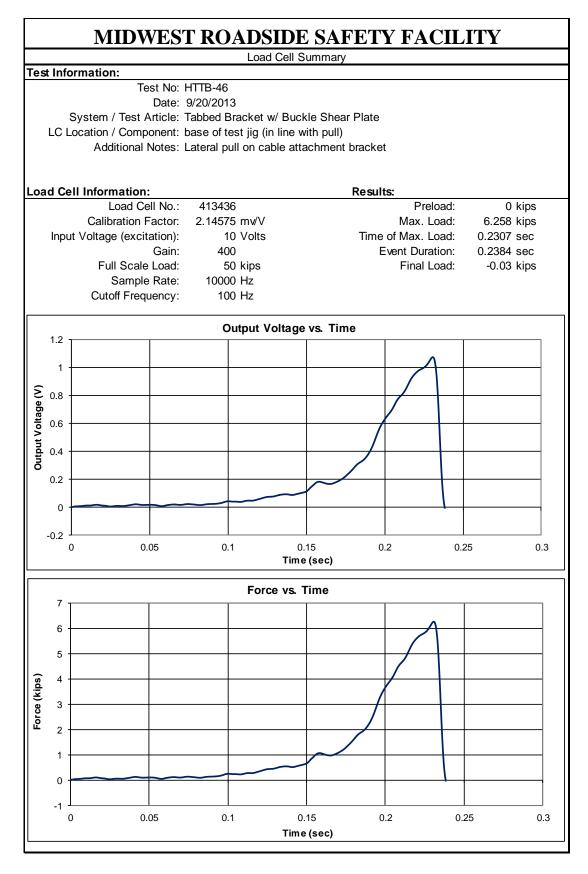
Figure B-6. Load Cell Results, Test No. HTTB-46
