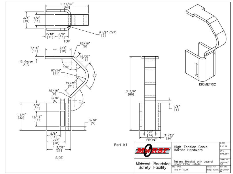
Figure 45. Tabbed Bracket with Lateral Shear Plate Details, Test Nos. HTTB-41, HTTB-42, HTTB-45, and HTTB-46
