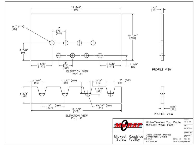
Figure 93. Cable Anchor Bracket Component Details, Test No. HTTC-2
