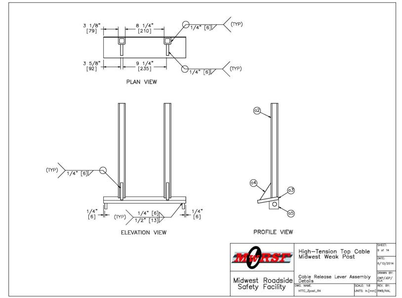
Figure 92. Cable Release Lever Assembly Details, Test No. HTTC-2
