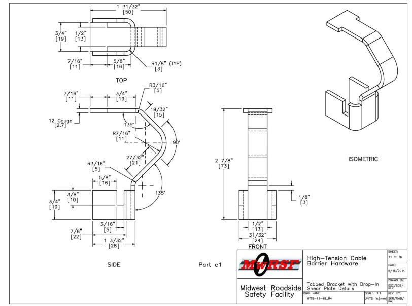
Figure 47. Tabbed Bracket with Drop-In Shear Plate Details, Test Nos. HTTB-43, HTTB-44, HTTB-47, and HTTB-48
