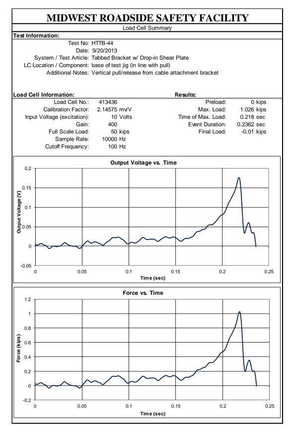
Figure B-4. Load Cell Results, Test No. HTTB-44
