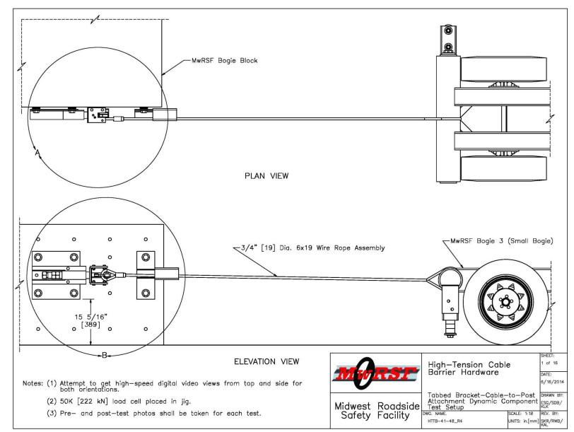
Figure 37. Cable-to-Post Attachment Dynamic Component Test Setup, Test Nos. HTTB-41 through HTTB-48
