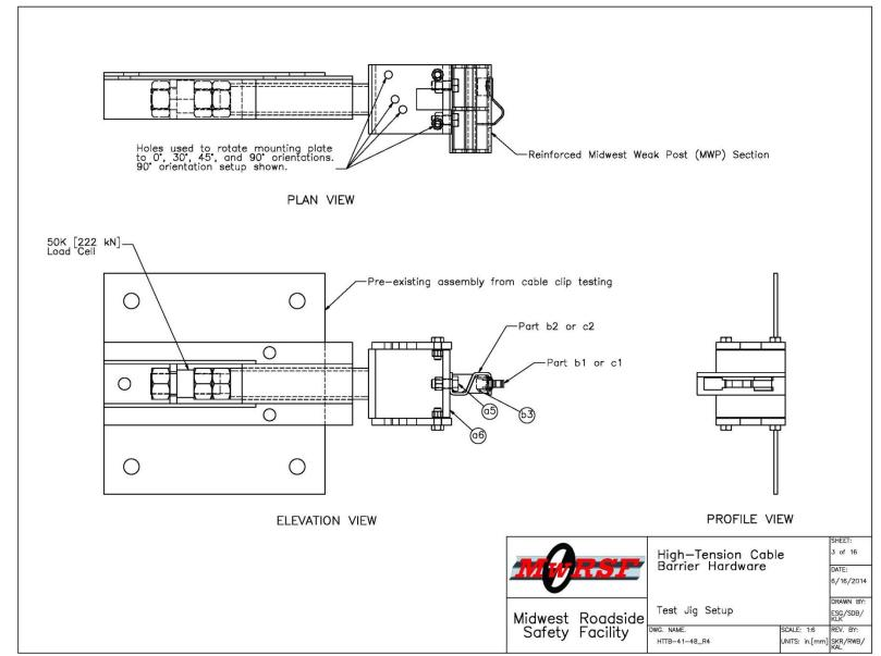
Figure 39. Test Jig Setup, Test Nos. HTTB-41 through HTTB-48
