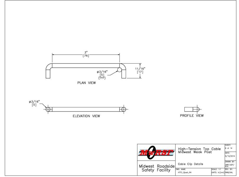
Figure 89. Cable Clip Details, Test No. HTTC-2
