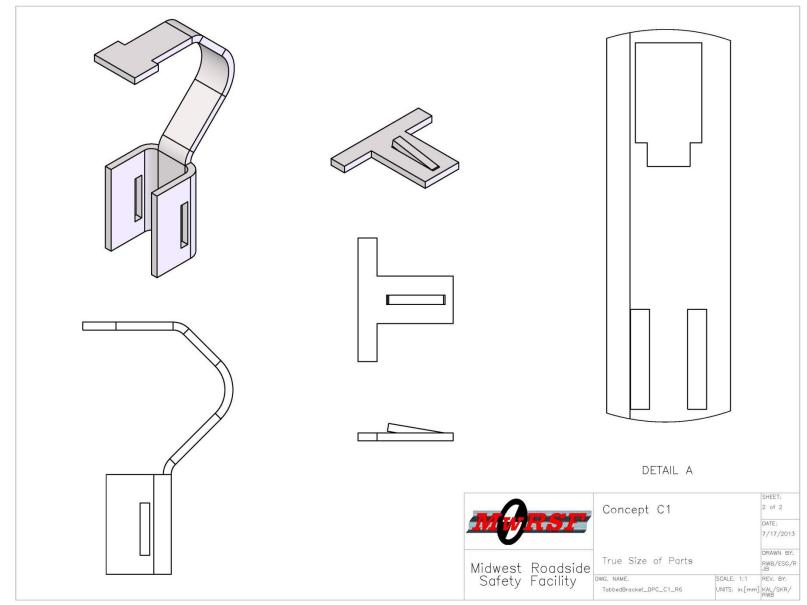
Figure 30. Concept C1, Lateral Shear Plate, Continued
