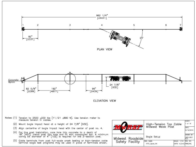
Figure 84. Bogie Setup, Test No. HTTC-2
