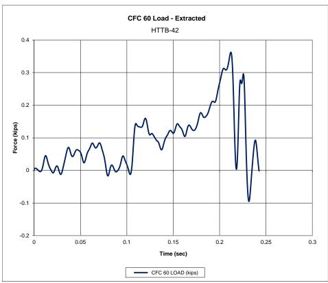
Figure 58. Force vs. Time Data, Test No. HTTB-42
