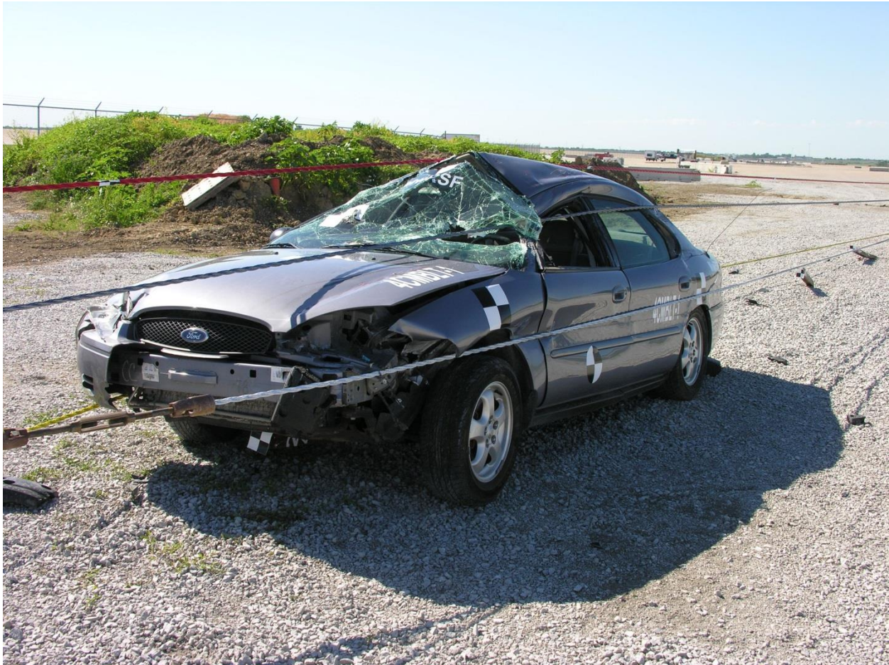
Figure 1. A-pillar Damage. Test No. 4CMBLT-1
