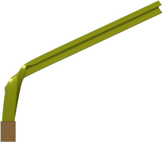
Figure 86. Deformed Post Shape, Test Nos. 4CMBC-11 and 4CMBC-12, and LS-DYNA Simulation
