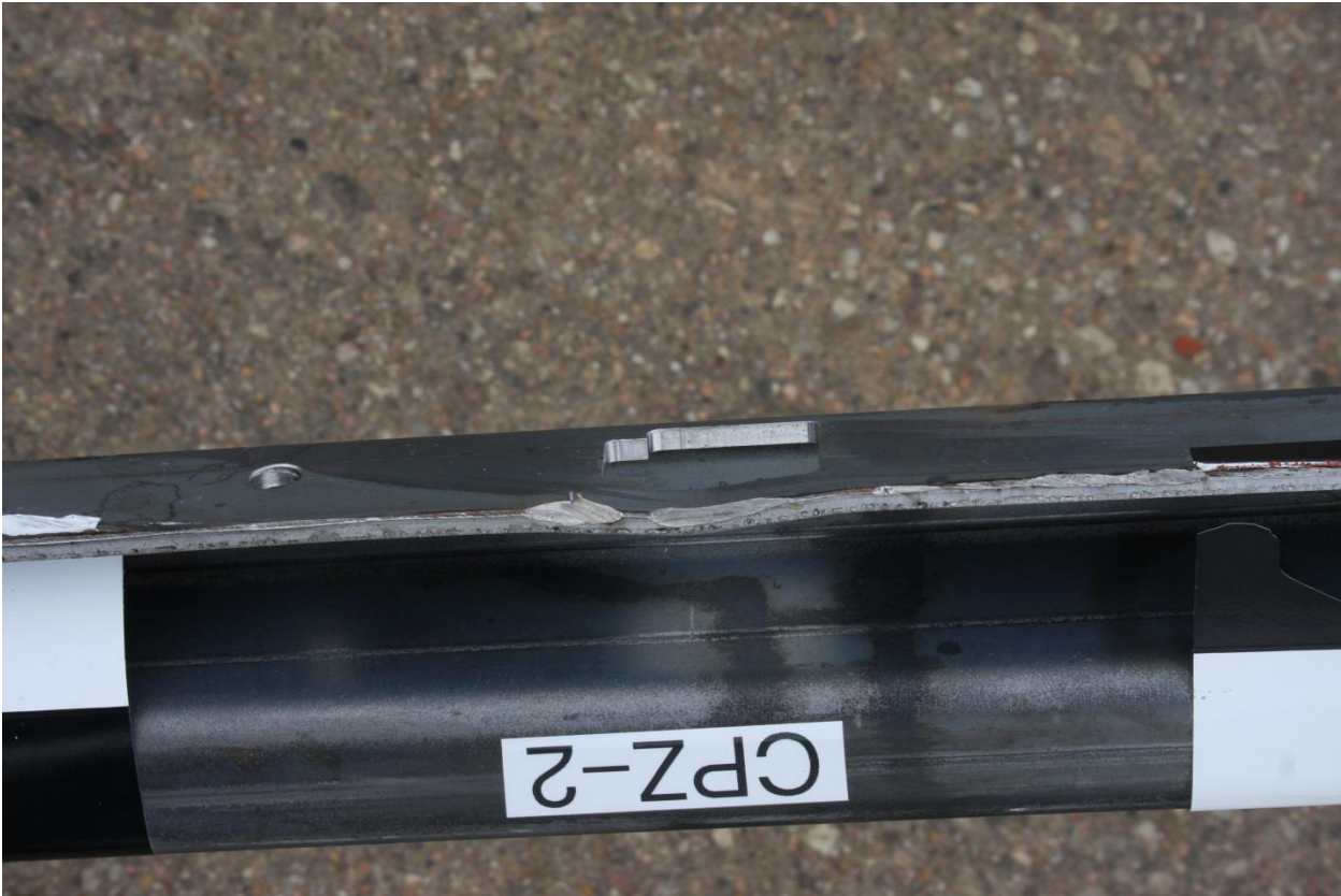
Figure 115. Localized Deformation of MWP Post Near Upper Keyway, Test No. CPZ-2
