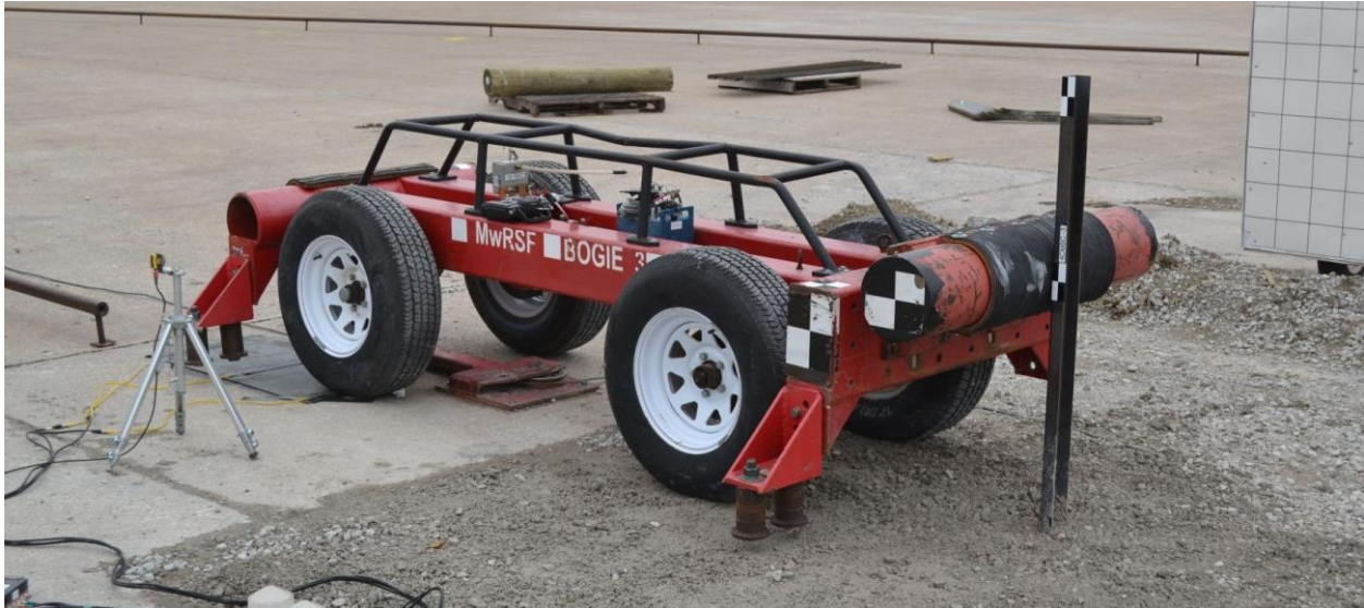
Figure 4. Rigid Frame Bogie and Guidance Track
