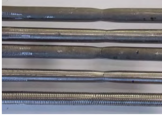
Figure 3.47: Initial surface roughness samples (top to bottom: surface blasted, rough finish, light turn blasted, light turn, and heavy turn).
