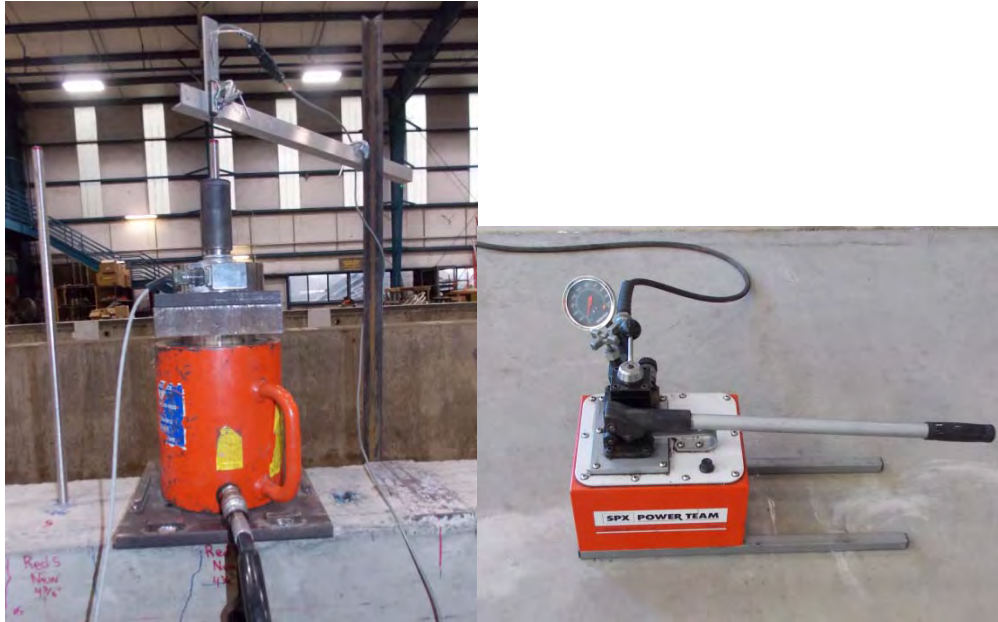
Figure 3.49: Pullout test setup and hydraulic hand pump.
