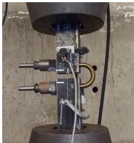
Figure 3.51: Sample 180° hook in test setup.
