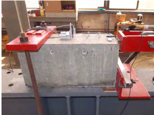
Figure 3.46: Loading setup for bond length specimens.
