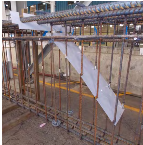
Figure 3.23: Preformed crack placement (IT specimen).
