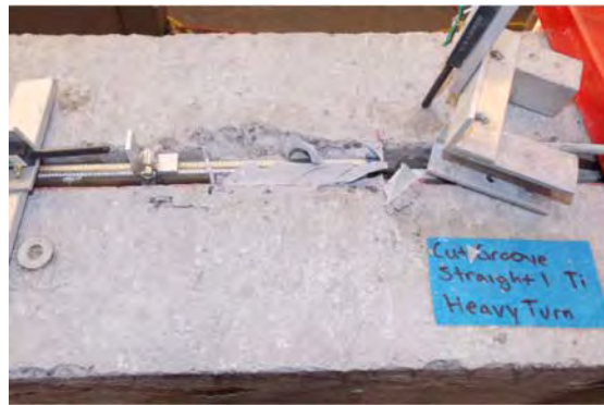
Figure 4.46: Bond stress specimen with 4 in. (102 mm) bond length at failure.
