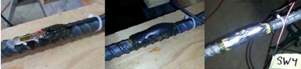
Figure 3.34: Application of strain gage on reinforcing bar.
