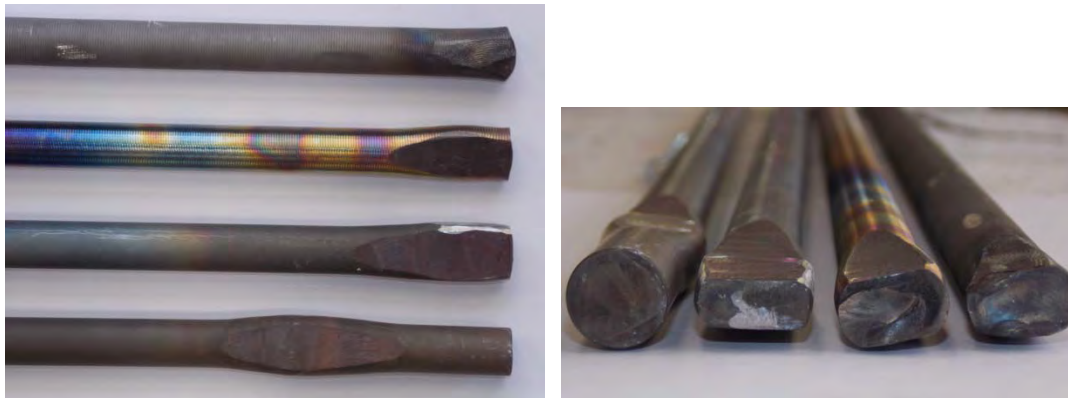
Figure 3.48: Bulb end samples for pullout testing.
