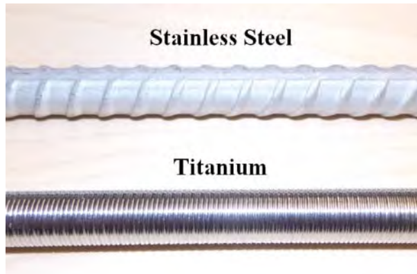
Figure 3.32: Deformation patterns on stainless steel (top) and titanium (bottom).
