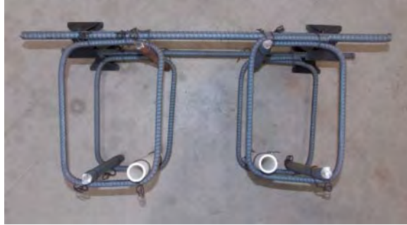
Figure 3.45: Reinforcing cage for bond length specimens.
