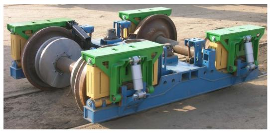
Figure 2. Prototype HST Used for Fitment and Yard On-Track Testing
