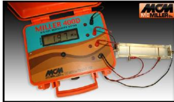
Figure 8. Miller 400D soil resistivity meter (M.C. Miller, 2010)
