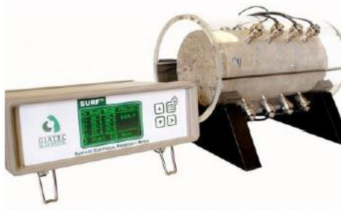
Figure 9. Giatec Surf surface resistivity meter (Giatec Scientific, 2015)
