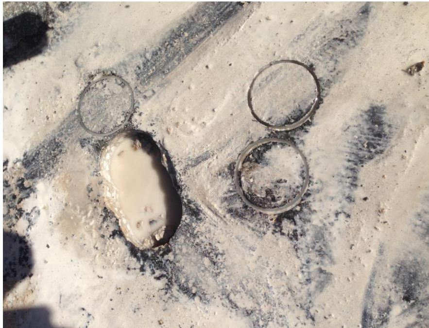
Figure 53. Six more unsuccessful attempts at drilling a core of the bridge deck
