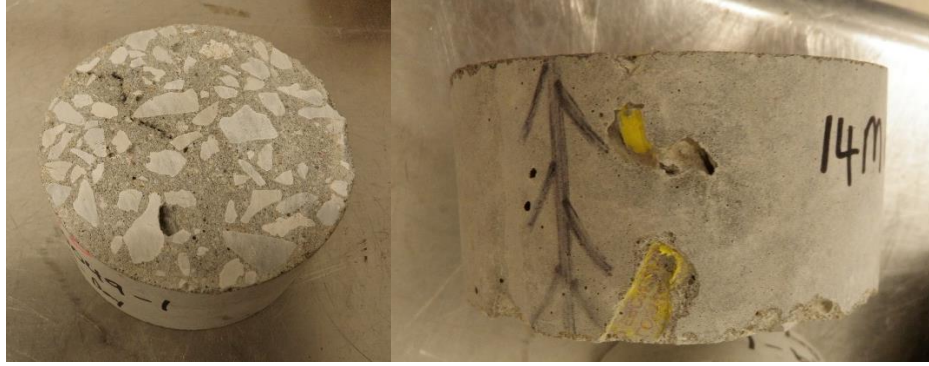
Figure 18. Field produced concrete cylinders with defects
